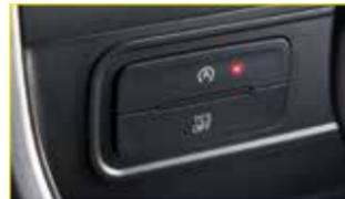
The system helps reduce fuel consumption by automatically stopping and restarting the engine when your vehicle has stopped. The engine restarts automatically when you release the brake pedal.
