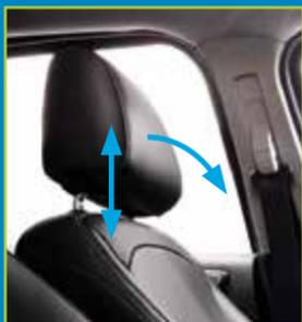
Tilt the head restraint forward for additional comfort by gently pulling the top of the head restraint. Once it is in the forward-most position, tilting it forward again releases it to the upright position.
