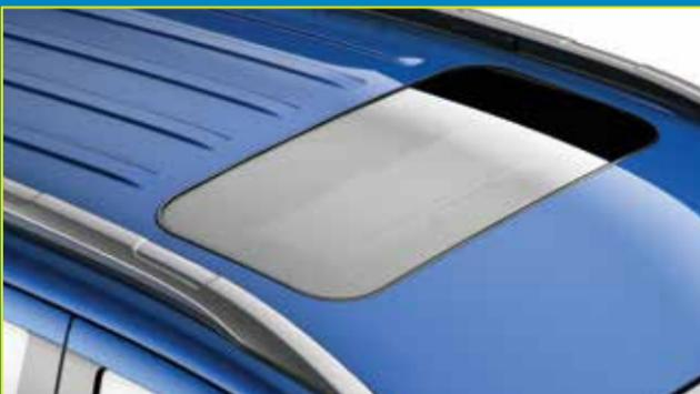
The moonroof has a one-touch open and close feature. To stop it during a one-touch operation, press the control a second time.
