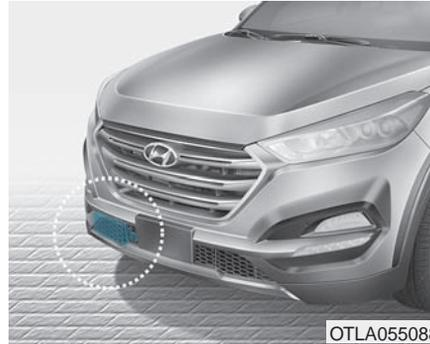
In order for the AEB system to operate properly, always make sure the radar sensor lens cover is clean and free of dirt, snow, and debris. Dirt, snow, or foreign substances on the lens may adversely affect the sensing performance of the radar.
