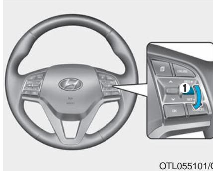
3. Push the toggle switch (1) down (SET-), and release it. The SET indicator light will illuminate.
