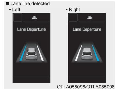
1. A visual warning appears on the cluster LCD display. Either the left lane line or the right lane line in the cluster LCD display will blink depending on which direction the vehicle is veering.
