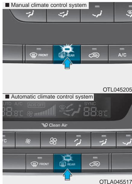
The defroster heats the window to remove frost, fog and thin ice from the interior and exterior of the rear window, while the engine is running.
