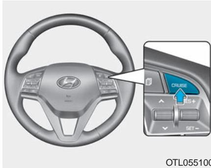
1. Press the CRUISE button on the steering wheel to turn the system on. The "CRUISE" indicator will illuminate.
