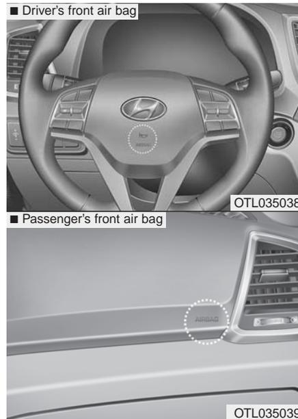
The purpose of the SRS is to provide the vehicle's driver and front passengers with additional protection than that offered by the seat belt system alone. The SRS uses sensors to gather information about the driver's and front passenger's seat belt usage and impact severity.
