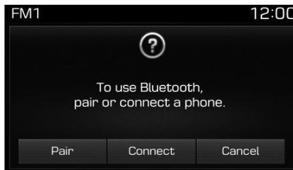
If *Bluetooth*® Wireless Technology devices are paired but none are currently connected, pressing the **[PHONE]** key or the **[↶]** key on the steering wheel displays the following screen. Press the **[Pair]** button to pair a new device or press the **[Connect]** to connect a previously paired device.
