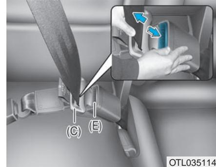
1. Press the release button on the rear center seat belt buckle (E) located on the left hand (driver) side of the center seat and remove the large tongue plate (C).
