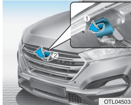
3. Go to the front of the vehicle, raise the hood slightly, push up the secondary latch (1) inside the hood center and lift the hood (2).
