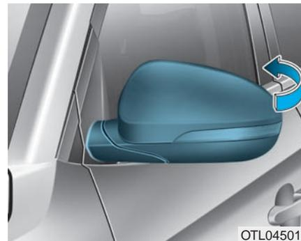
To fold either the left or right hand side view mirror, grasp the housing of the mirror and then fold it toward the rear of the vehicle.
