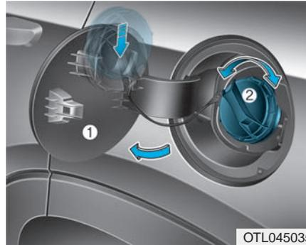
3. Pull the fuel filler door (1) outward to access the fuel tank cap.
