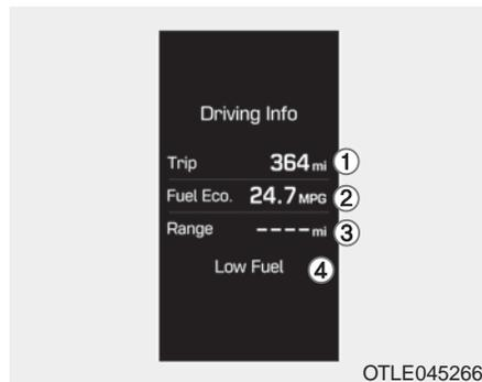
At the end of each driving cycle, the Driving Info message is displayed. This display shows the trip distance, the average fuel economy, and the remaining vehicle range.
