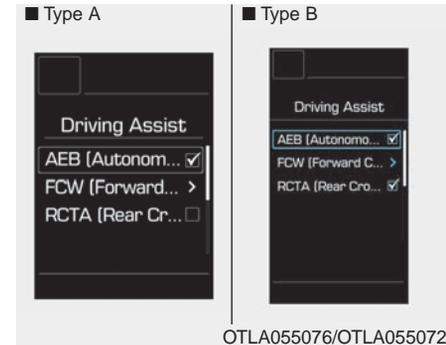
The driver can activate the AEB by placing the ignition switch to the ON position and by selecting 'User Settings', 'Driving Assist', and 'AEB (Autonomous Braking System)'. The AEB deactivates, when the driver cancels the system setting.
