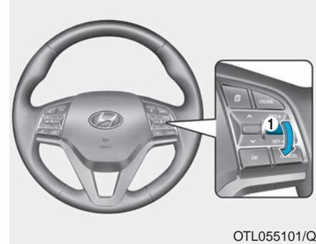
Push the toggle switch (1) up (RES+). If the vehicle speed is over 20 mph (30 km/h), the vehicle will resume the preset speed.
