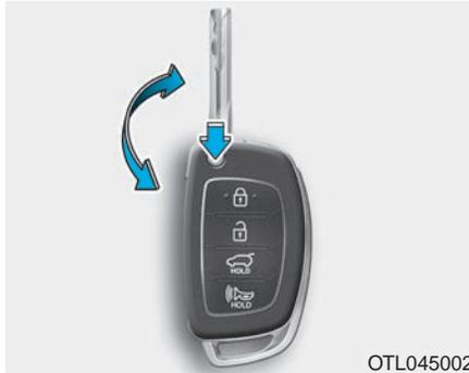
If the remote key does not operate normally, you can lock or unlock the door by using the mechanical key.
