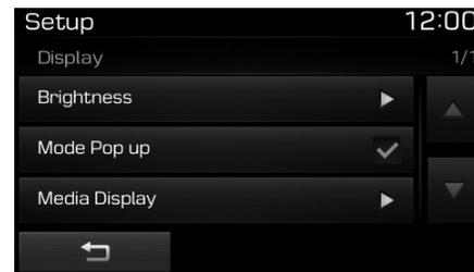
This feature is used to display the Mode Pop up screen when entering radio and media modes.
