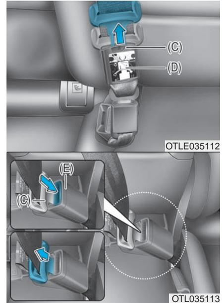
3. Slip the large tongue plate (C) out of the pocket (D) located on the belt assembly.
