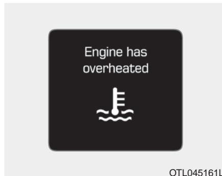
This warning message is displayed when the engine coolant temperature is above 248°F (120°C). This means that the engine is overheated and may be damaged.
