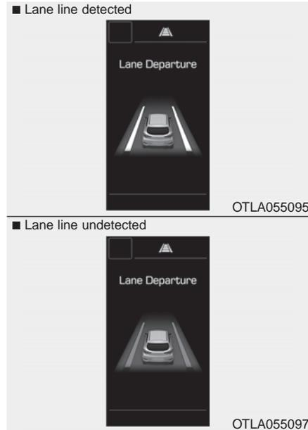
If your vehicle speed exceeds 40 mph (64 km/h) and the LDWS button is ON, the system is enabled. If your vehicle departs from the projected lane in front of you, the LDWS operates as follows:
