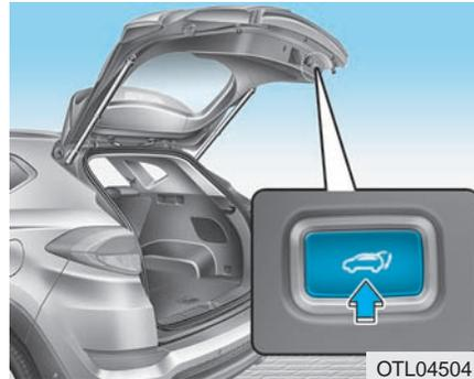
1. Press the power liftgate inner button for approximately 1 second.
