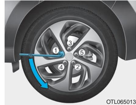
6. Loosen the wheel lug nuts counterclockwise one turn each in the order shown above, but do not remove any lug nuts until the tire has been raised off of the ground.
