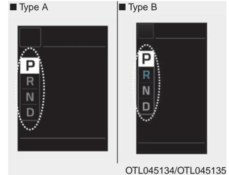
The pop-up displays the current gear position selected for 2 seconds (P/R/N/D).
