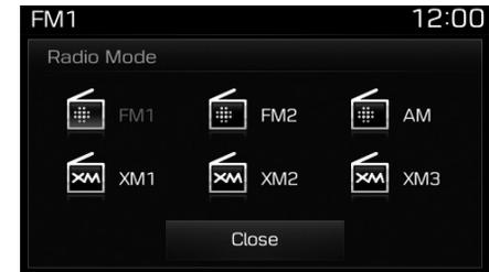
Turn the **TUNE** knob to move the focus. Press the knob to select.
