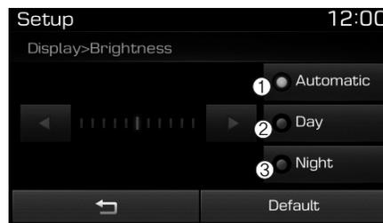
Use the **◀**, **▶** buttons to adjust the screen brightness or set the Brightness on Automatic, Day, or Night mode.
