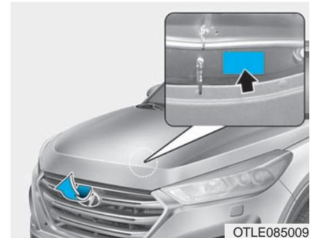
The refrigerant label provides information such as refrigerant type and amount. The label is located on the underside of the hood.
