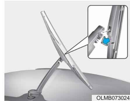
3. Install the new blade assembly by inserting the center part into the slot on the wiper.
