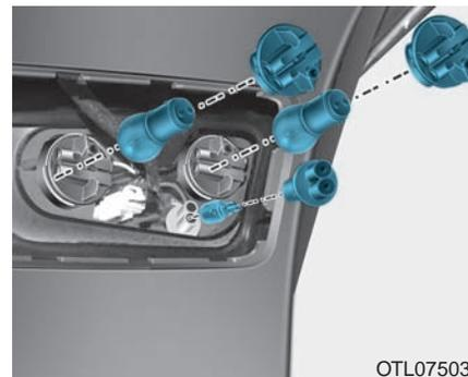
4. Remove the socket from the assembly by turning the socket counterclockwise until the tabs on the socket align with the slots on the assembly.
