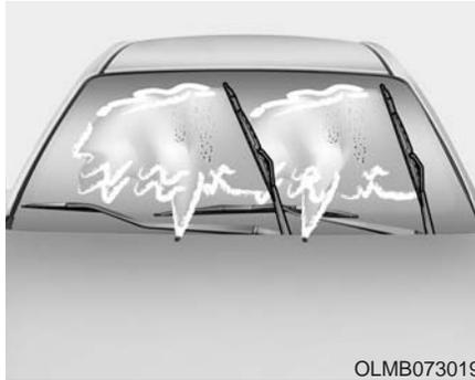
Contamination of either the windshield or the wiper blades with foreign matter can reduce the effectiveness of the windshield wipers. Common sources of contamination are insects, tree sap, and hot wax treatments used by some commercial car washes. If the blades are not wiping properly, clean both the window and the blades with a clean cloth dampened with washer fluid.
