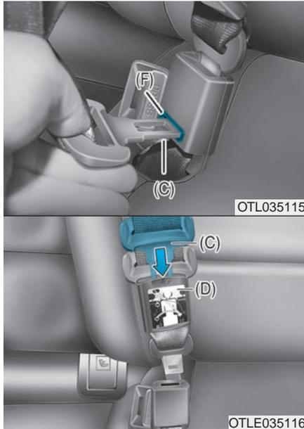
2. To release and retract the rear center seatbelt assembly, insert a small tool or key into the primary buckle release hole (F) located on the right hand (passenger) side of the center seat. You can also insert the large buckle (C) into the release hole to release the seat belt assembly.
