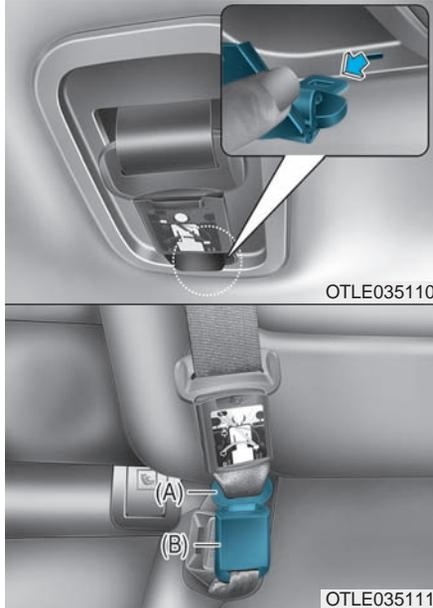
1. Extract the small tongue plate from the slot on the belt assembly pocket located in the headliner.
