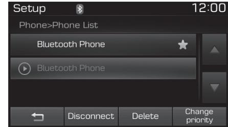
From the paired phone list, select the currently connected device and press the **Disconnect** button.
