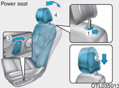
To reinstall the head restraint:
