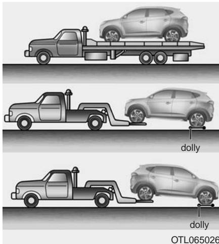
If emergency towing is necessary, we recommend having it done by an authorized HYUNDAI dealer or a commercial tow-truck service. Proper lifting and towing procedures are necessary to prevent damage to the vehicle. The use of wheel dollies or flatbed is recommended.
