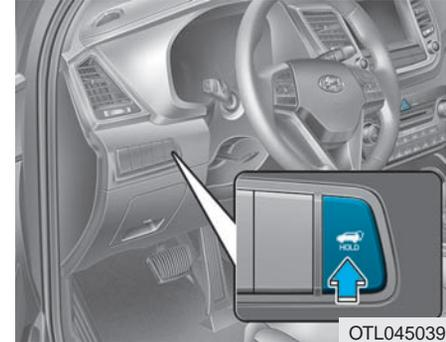
When the ignition switch is in the ON position and the shift lever is in Park (P), the power liftgate can be opened by using the console button on the dash.
