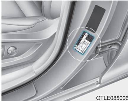
The tires supplied on your new vehicle are chosen to provide the best performance for normal driving. The tire label located on the driver's side center pillar gives the tire pressures recommended for your car.
