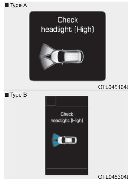
This warning message is displayed if the headlamps are not operating properly. The headlamp bulb may need to be replaced. If the vehicle is equipped with LED headlamps, have the vehicle inspected by an authorized HYUNDAI dealer.
