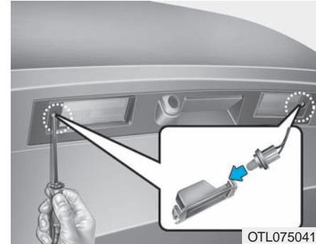
1. Loosen the lens retaining screws with a screwdriver.
