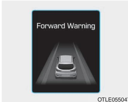
This initial warning message appears on the LCD display with a warning chime.
