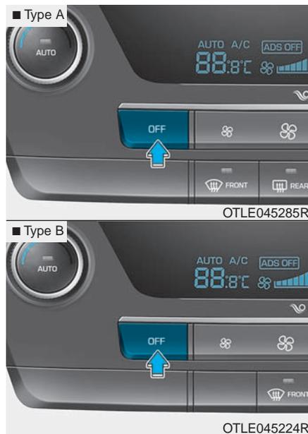
Push the OFF button of the front to turn off the air climate control system. You can still operate the mode and air intake buttons as long as the ignition switch is in the ON position.
