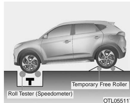
A full-time AWD vehicle should not be tested on a 2WD roll tester. If a 2WD roll tester must be used, perform the following procedure:
