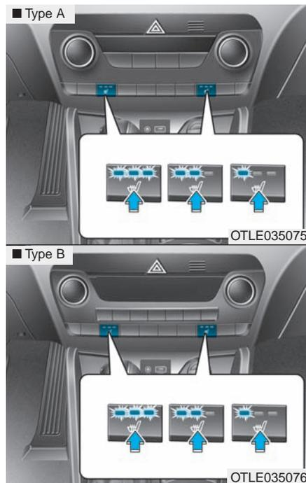
While the engine is running, push either of the switches to warm the driver's seat or front passenger's seat.
