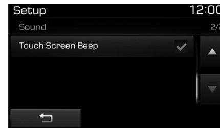
This feature is used to turn the touch screen beep on/off.
