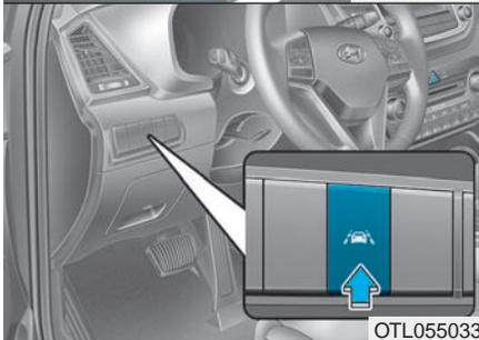
The Lane Departure Warning (LDWS) System feature is designed to monitor the vehicle's position relative to the lane in front of you and detect when the vehicle begins to move out of its lane.
