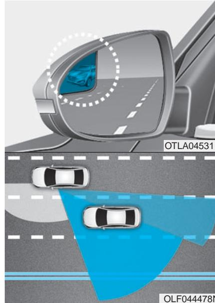
The Blind Spot Mirror (BSM) is a supplemental mirror that minimizes the driver's blind spot zone by expanding the field of view on the rear side of the vehicle. The blind spot mirror is equipped on the driver's left side view mirror.
