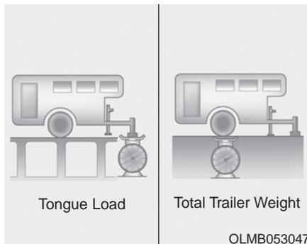
What is the maximum safe weight of a trailer? It should never weigh more than the maximum trailer weight with trailer brakes. But even that can be too heavy. It depends on how you plan to use your trailer. For example, speed, altitude, road grades, outside temperature and how often your vehicle is used to pull a trailer are all important. The ideal trailer weight can also depend on any special equipment that you have on your vehicle.
