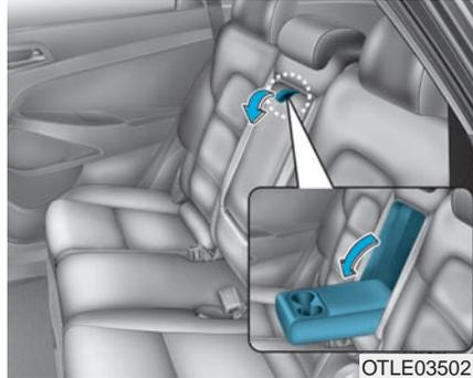
The armrest is located in the center of the rear seat. Pull the armrest down by using the strap from the seatback to use it.
