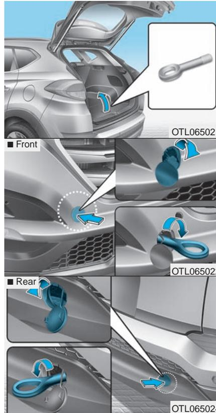
1. Open the tailgate, and remove the towing hook from the tool case.
