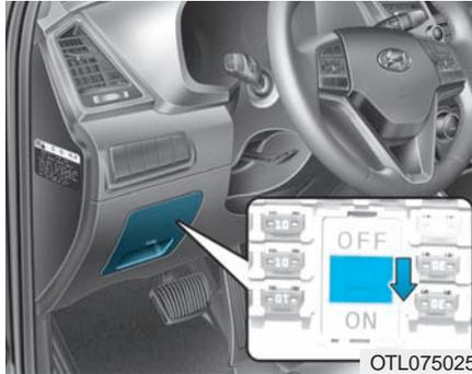
Always, place the fuse switch to the ON position.
