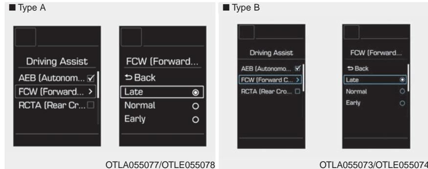
The driver can select the initial warning activation time in the User Settings in the Driver LCD display. The options for the initial Forward Collision Warning include the following:
