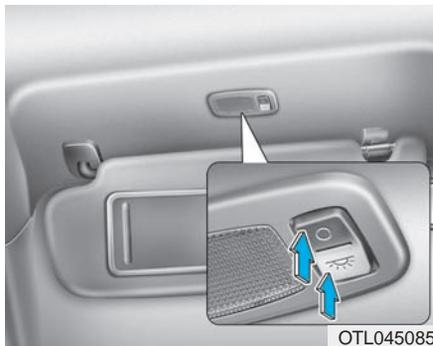
The vanity mirror lamp is located in the headliner just behind the sun visor. Push the switch to turn the vanity light on or off.
