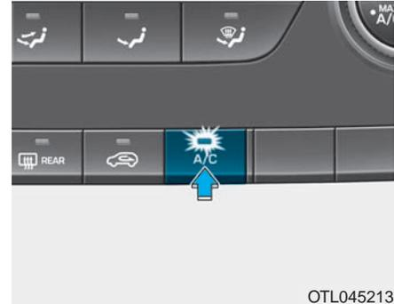
Press the A/C button to turn the system on (indicator light will illuminate) and off.
