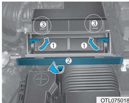
5. Pull up the lever (1) to the LOCK position.
