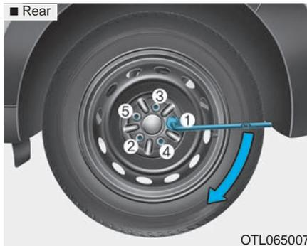
13. Use the wheel lug nut wrench to tighten the lug nuts in the order shown. Double-check each lug nut until they are tight. After changing tires, have an authorized HYUNDAI dealer tighten the lug nuts to their proper torque as soon as possible. **The wheel lug nut should be tightened to 65~79 lb.ft (9~11 kg.m).**
