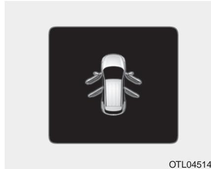
This warning message is displayed indicating which door, or the hood, or the liftgate is open.
