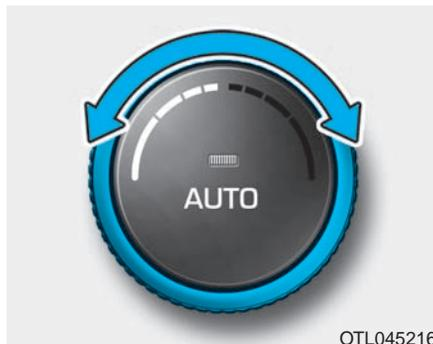
2. Turn the temperature control knob to the desired temperature. If the temperature is set to the lowest setting (Lo), the air conditioning system will operate continuously.
