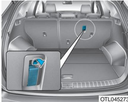
To hang a plastic bag, open the tailgate and find a hook attached on rear seat back.
