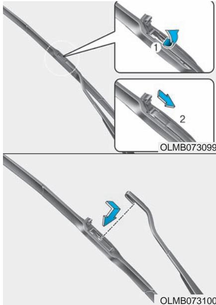
2. Lift up the wiper blade clip (1). Then pull down the blade assembly (2) and remove it.
