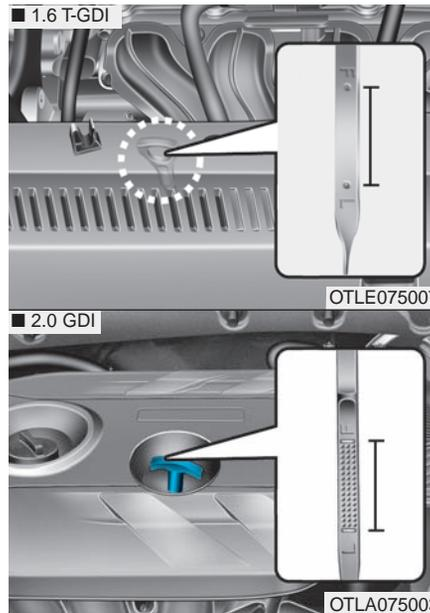
6. Pull the dipstick out again and check the level. The level should be between F and L.
