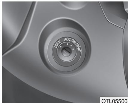
Whenever the front door is opened, the ignition switch will illuminate, provided the ignition switch is not in the ON position. The light will go off immediately when the ignition switch is turned on or go off after about 30 seconds when the door is closed.
