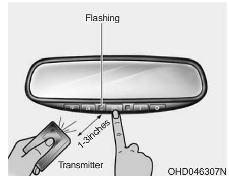
2. Press and hold the button on the HomeLink system you wish to train and the button on the transmitter while the transmitter is approximately 1 to 3 inches away from the mirror. Do not release the buttons until step 3 has been completed.
