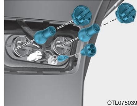
4. Remove the socket from the assembly by turning the socket counterclockwise until the tabs on the socket align with the slots on the assembly.
