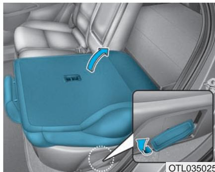
5. To use the rear seat, lift and pull the seatback rearward. Pull the seatback firmly until it clicks into place. Make sure the seatback is locked in place.
