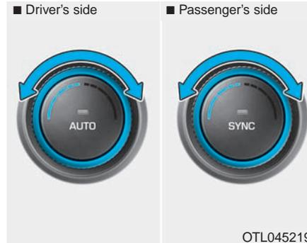
Turn the knob to the right to increase the temperature. Turn the knob to the left to decrease the temperature.
