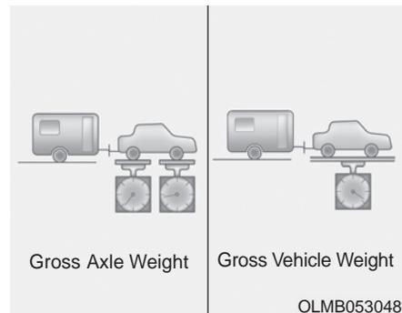
The tongue load is an important weight to measure because it affects the total Gross Vehicle Weight (GVW) of your vehicle. The trailer tongue should weigh a maximum of 10% of the total loaded trailer weight, within the limits of the maximum trailer tongue load permissible.
