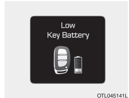
This warning message is displayed if the battery of the smart key is discharged when the Engine Start/Stop button changes to the OFF position.
