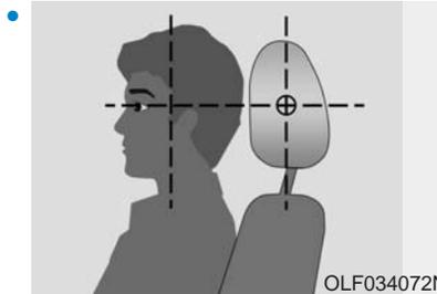
Adjust the head restraints so the middle of the head restraints is at the same height as the height of the top of the eyes.
