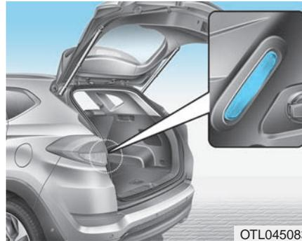
The liftgate room lamp comes on when the tailgate is opened.
