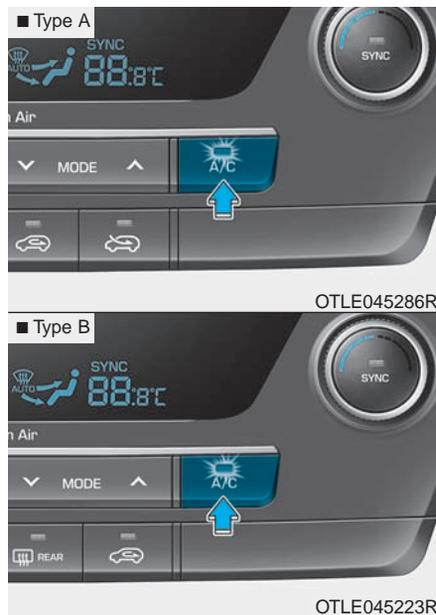
Push the A/C button to manually turn the system on (indicator light will illuminate) and off.
