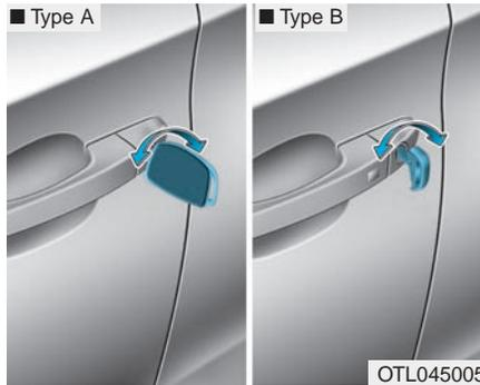
If you lock the driver's door with turning the key toward the front of the vehicle, all vehicle doors will lock. If you unlock the driver's door with turning the key toward the rear of the vehicle, the driver's door will unlock.
