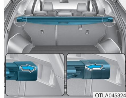
1. Push one side of the cargo screen inward to compress the spring mechanism and release the screen from the vehicle.
