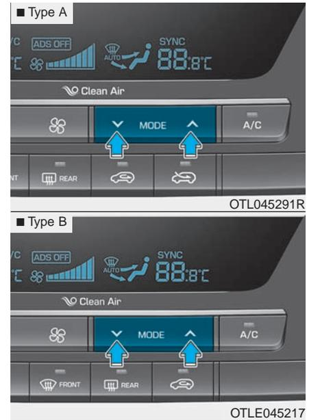
The mode selection button controls the direction of the air flow through the ventilation system.
