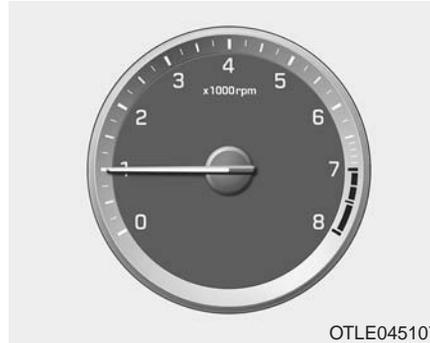
The tachometer indicates the approximate number of engine revolutions per minute (rpm).
