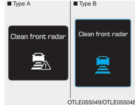
When the sensor lens cover is blocked with dirt, snow, or debris, the AEB system operation may stop temporarily. If this occurs, a warning message will appear on the LCD display. Remove any dirt, snow, or debris and clean the radar sensor lens cover before operating the AEB system.
