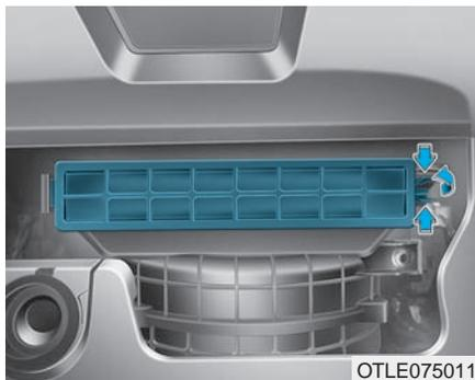
3. Remove the climate control air filter case by pulling out the right side of the cover.
