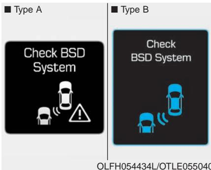
If there is a problem with the BSD system, a warning message will appear and the light on the switch will turn off. The system will turn off automatically. Have your vehicle inspected by an authorized HYUNDAI dealer.
