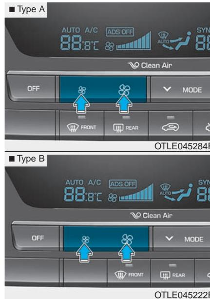
The fan speed can be set to the desired speed by pushing the fan speed control button. Pressing the OFF button turns off the fan.
