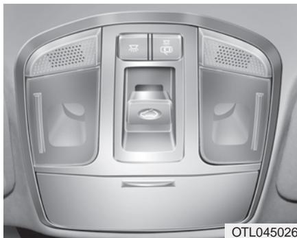
The ignition switch must be in the ON position before you can open or close the sunroof.
