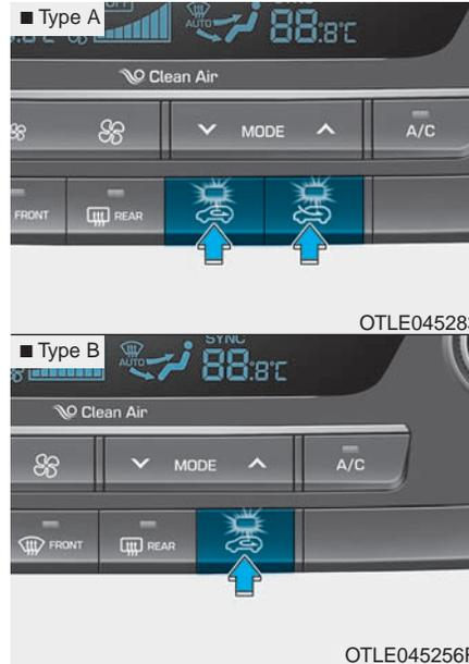
This button is used to select the outside (fresh) air position or recirculated air position.
