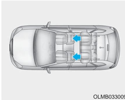
The vehicle's front seats are equipped with adjustable head restraints for both safety and comfort.
