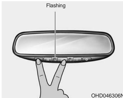
1. When programming the buttons for the first time, press and hold the left and center buttons (🏠, 🏠) simultaneously for approximately 20 seconds until the indicator light begins to flash. (This procedure erases the factory-set default codes. Do not perform this step to program additional hand-held transmitters.)
