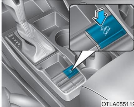
The Downhill Brake Control (DBC) feature assists the driver to descend down a steep hill without having to depress the brake pedal. The system automatically applies the brakes to maintain the vehicle speed below 5 mph (8 km/h) and allows the driver to concentrate on steering the vehicle down hill.
