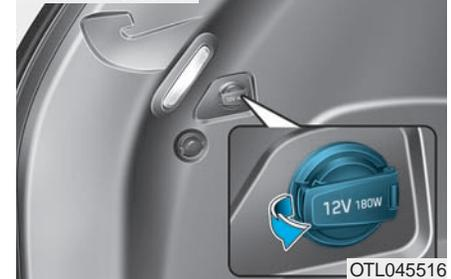
The power outlet is designed to provide power for mobile telephones or other devices designed to operate with vehicle electrical systems. The devices should draw less than 180 W with the engine running.
