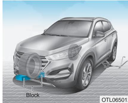
5. Block both the front and rear of the tire diagonally opposite of the tire you are changing.
