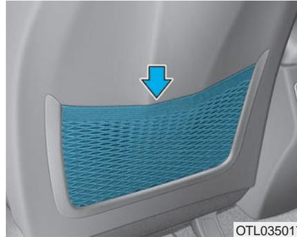
The seatback pocket is provided on the back of the front seatbacks.
