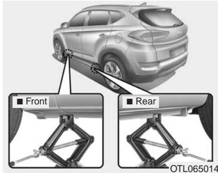
7. Place the jack at the designated jacking position under the frame closest to the tire you are changing. The jacking positions are plates welded to the frame with two notches and two dimples. Never jack any other position or part of the vehicle. Doing so may damage the side seal molding or other parts of the vehicle.
