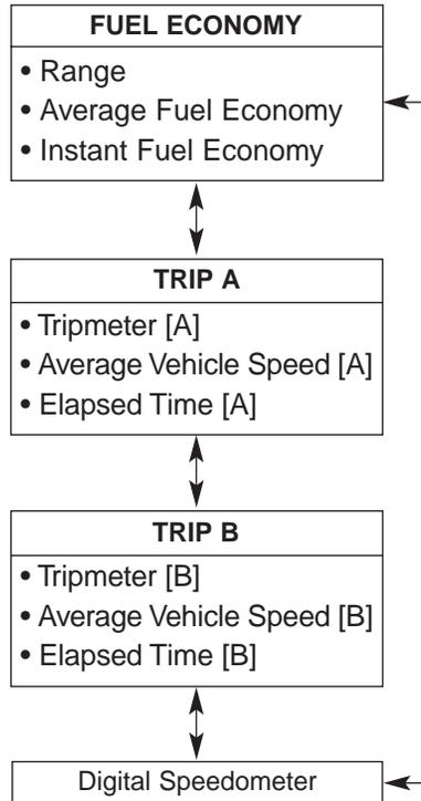
To change the trip mode, toggle the UP/DOWN arrow switch "▲", "▼" on the steering wheel.
