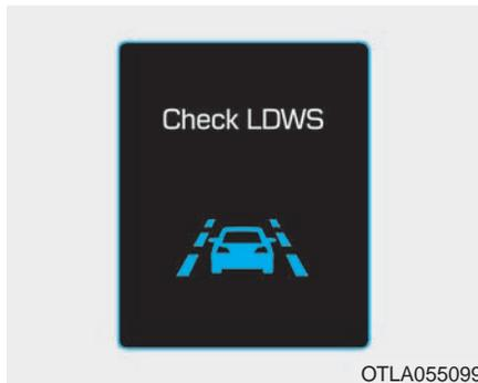
If there is a malfunction with the LDWS, the indicator on the cluster will illuminate yellow. Additionally, a message that reads, "Check LDWS", will appear on the cluster LCD display. After the message disappears, the master warning light (⚠) will illuminate.
