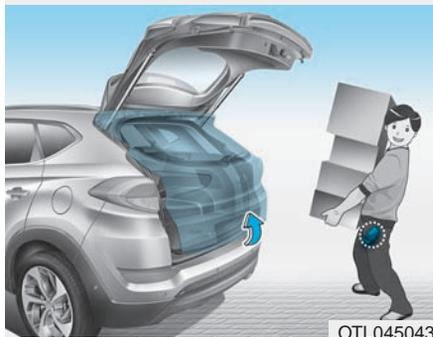
On vehicles equipped with a smart key, the liftgate can be opened with hands-free activation using the Smart Liftgate system.
