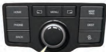
Press and hold the controller to save station.
