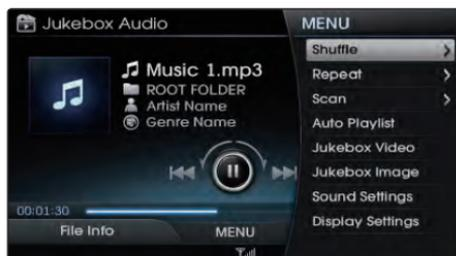
After selecting the desired feature, press the controller to start operating feature. Press the **MENU** key again to hide the menu window.
