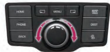
Turn the controller to left/right and select the desired HD Radio station.
