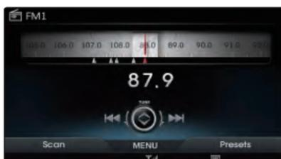
Within the TUNE mode, turn the controller left/right to search for frequencies.
