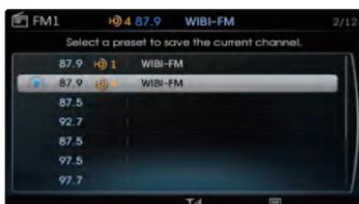
Stations can also be saved manually by pressing the **MENU** key ► Selecting **Save Station**.
