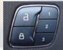
The memory function allows a one-touch recall of personalized memory features including the driver seat, power mirrors and steering column\*. Use the memory controls on the driver's door to program and then recall memory positions. To program position **1**, press and hold **1** until you hear a tone. Use this same procedure to set positions **2** and **3** by pressing the respective buttons. You can now use these controls to recall the set memory positions.
