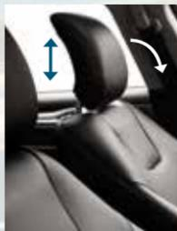
After the head restraint reaches the forward-most tilt position, pivoting it forward again releases it to the rearward, un-tilted position.
