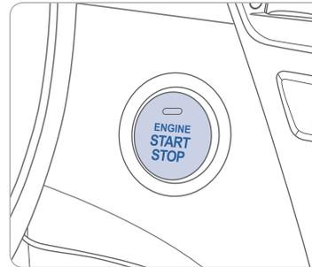
With the ignition OFF, press the engine start/stop button:
