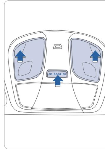
Press the lens to turn the lamp on or off.
