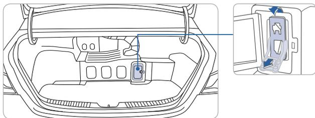
The Service plug is located inside the trunk. This plug should only be serviced or inspected by an authorized Hyundai dealer.
