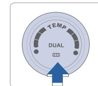
Press the DUAL button to operate the driver and passenger side temperatures individually.
