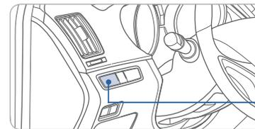
Push button to the left to reduce brightness and push button to the right to increase brightness.
