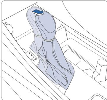
The rearview camera will activate when the ignition switch is ON and the shift lever is in the R (Reverse) position.
