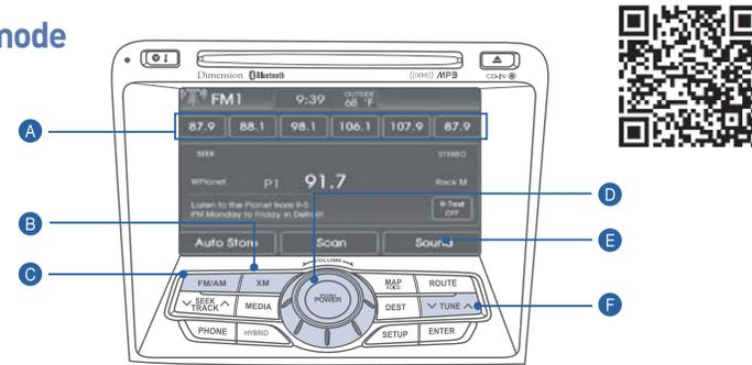
Press POWER button **D** to turn radio on.
