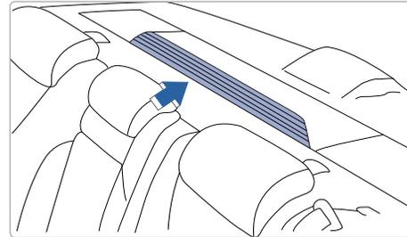
The Hybrid battery air intake vent is located behind the rear seat head rest. Do not cover the air vent or spill liquid.
