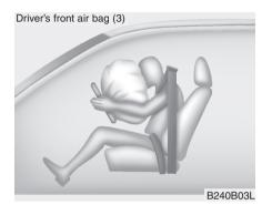
A fully inflated air bag, in combination with a properly worn seat belt, slows the driver's or the passenger's forward motion, reducing the risk of head and chest injury.
