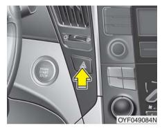
The hazard warning flasher should be used whenever you find it necessary to stop the car in a hazardous location. When you must make such an emergency stop, always pull off the road as far as possible.
