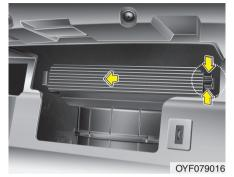
Remove the climate control air filter cover while pressing the lock on the right of the cover.
