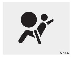
The SRS air bag warning light " on the instrument panel will illuminate for about 6 seconds after the engine start/stop button is turned to the ON position, after which the SRS air bag warning light " should go out.
