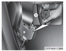
Anchor connector for front seat belt
