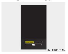
This State of Charge(SOC) gauge indicates the remaining Hybrid battery power. If the SOC is near L level, the vehicle automatically operates the engine to charge the battery. However, if the service indicator and MIL(Malfunction indicator lamp) turn on when the State of Charge(SOC) is near L(Low), have your vehicle checked by an authorized HYUNDAI dealer immediately.
