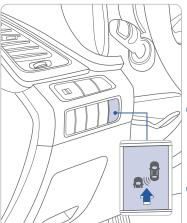
The BSD system sensor senses the rear side territory of the vehicle and provides information to the driver.
