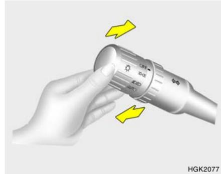
To flash the headlights, pull the switch lever toward you, then release it. The headlights can be flashed even though the headlight switch is in the "OFF" position.
