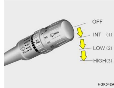
The windshield wiper switch has three positions:
