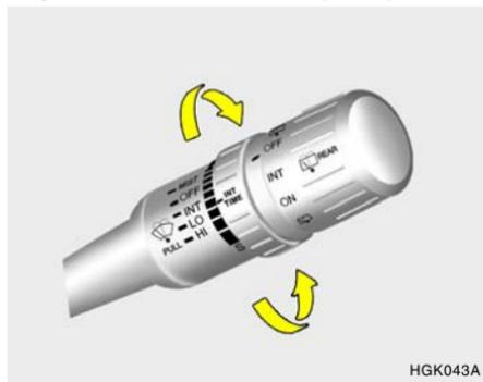
To use the intermittent wiper feature, place the wiper switch in the "INT" position. With the switch in this position, the interval between wipes can be varied from 2 to 10 seconds by turning the interval adjuster barrel.
