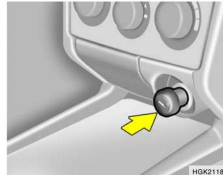
For the cigarette lighter to work, the key must be in the "ACC" position or the "ON" position. To use the cigarette lighter, push it all the way into its socket. When the element has heated, the lighter will pop out to the "ready" position. Do not hold the cigarette lighter pressed in. This can damage the heating element and create a fire hazard.
