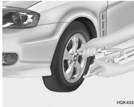
If you have a tire gauge, remove the valve cap and check the air pressure. If the pressure is lower than recommended, drive slowly to the nearest service station and inflate to the correct pressure. If it is too high, adjust it until it is correct. Always reinstall the valve cap after checking or adjusting tire pressure. If the cap is not replaced, air may leak from the tire. If you lose a valve cap, buy another and install it as soon as possible.
