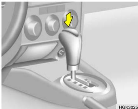
The highly efficient Hyundai automatic transaxle has four forward speeds and one reverse speed. The individual speeds are selected automatically, depending on the position of the speed selector lever. The selector lever has 2 gates; the main gate and the manual gate.
