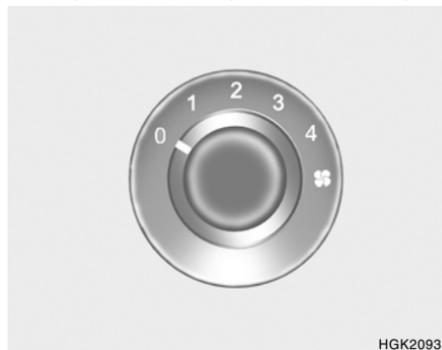
This is used to turn the blower fan on or off and to select the fan speed.
