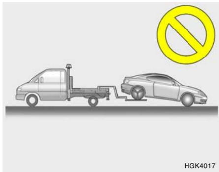
**A vehicle with an automatic transaxle should never be towed from the rear with the front wheels on the ground. This can cause serious damage to the transaxle. Be sure to use a towing dolly under the front wheels.**
