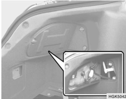
3. Remove the nut (8mm) with a spanner.
