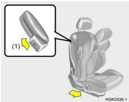
By pulling up the walk in device lever (1) at the right-upper side of the passenger side seatback, the seatback will tilt forward. Then push the seat forward to allow the occupants to enter.
