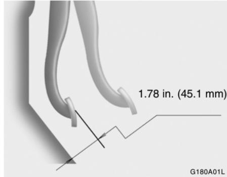
You need a helper to check the brake pedal clearance. With the engine running, have your helper press down on the brake pedal several times and then hold it down with a force of about 110 lbs (50 kg, 490 N). The brake pedal clearance is the distance from the top surface of the brake pedal to the asphalt sheeting under the floor mat.
