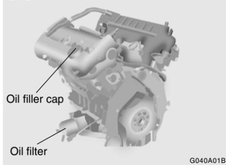
The engine oil and filter should be changed at those intervals specified in the maintenance schedule in Section 5. If the car is being driven in severe conditions, more frequent oil and filter changes are required.
