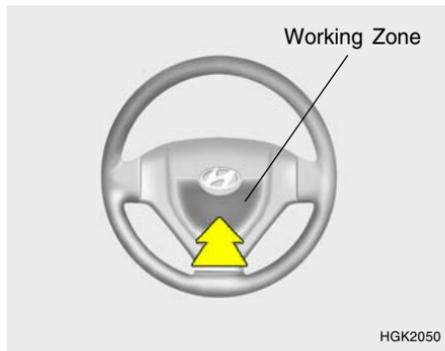
Press the pad on the steering wheel to sound the horn.
