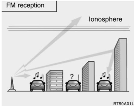
AM and FM radio signals are broadcast from transmitter towers located around your city. They are intercepted by the radio antenna on your car. This signal is then received by the radio and sent to your car speakers.
