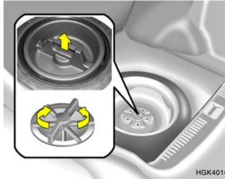
Remove the installation bolt to remove the spare tire. To replace the spare tire in its storage compartment, tighten the bolt firmly with your fingers until there is no more play in the spare tire.
