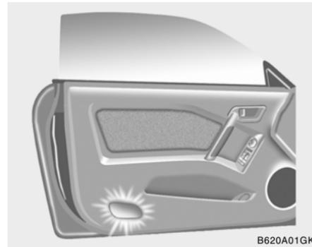
A red light comes on when the front door is opened. The purpose of this light is to assist when you get in or out and also to warn passing vehicles.
