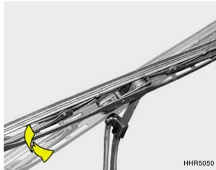
1. Put a new wiper blade onto the wiper arm and lower the wiper blade at the level of the wiper arm as shown in the drawing.
