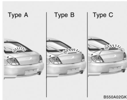
In addition to the lower-mounted rear stoplights on either side of the car, the high mounted rear stoplight in the center of the rear window or inserted in the rear spoiler also lights when the brakes are applied.
