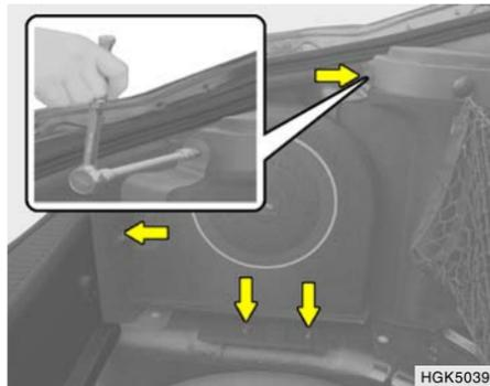
3. Extract the mounting screws (10mm) around the woofer speaker with a spanner.
