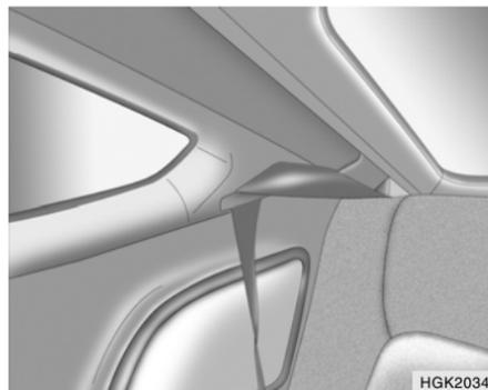
In order to prevent the shoulder belt from being damaged while folding the rear seat, the shoulder belt must be passed through the hanger to keep it out of the way.
