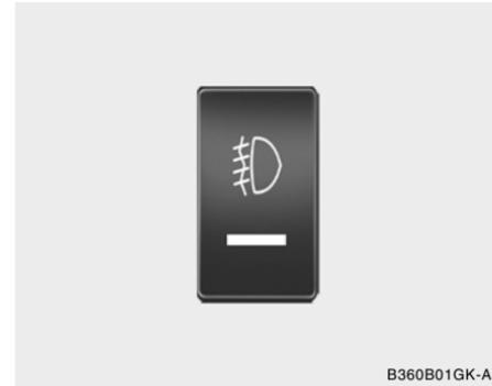
To turn on the front fog lights, push the switch. They will light when the headlight switch is in the second position and the ignition key is in the "ON" position.
