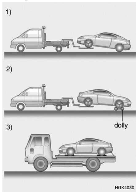
Your vehicle can be towed by wheel lift type truck (1), (2) or flatbed equipment (3).
