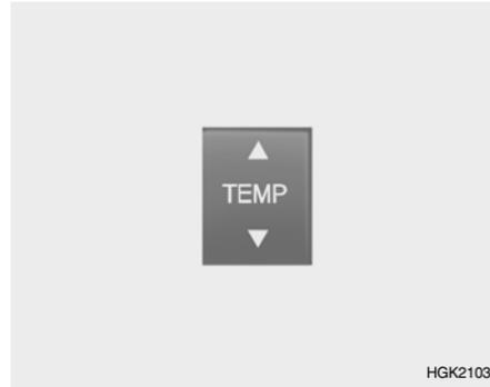
2. Push the "TEMP" button to set the desired temperature.
