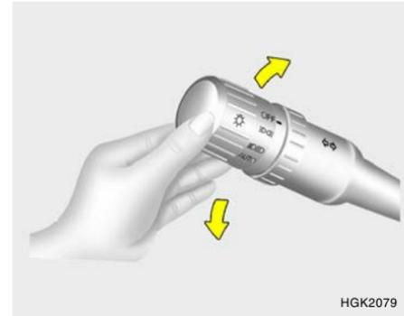
To indicate a lane change, move the lever up or down to a point where it begins flashing. The lever will automatically return to the center position when released.
