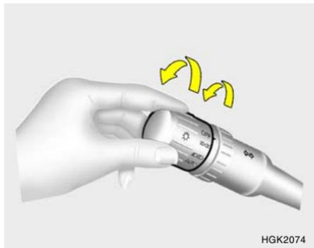
To operate the headlights, turn the barrel on the end of the multi-function switch. The first position turns on the parking lights, sidelights, tail lights and instrument panel lights. The second position turns on the headlights.
