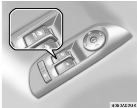
The Auto-Down window is moved to its fully open position by pushing the switch. To stop at the desired position push in on the switch again.
