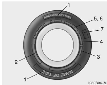
Federal law requires tire manufacturers to place standardized information on the sidewall of all tires. This information identifies and describes the fundamental characteristics of the tire and also provides the tire identification number (TIN) for safety standard certification. The TIN can be used to identify the tire in case of a recall.
