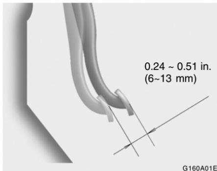
With the engine off, press lightly on the clutch pedal until you feel a change in resistance. This is the clutch pedal free-play. The free-play should be within the limits specified in the illustration. If it is not, have it inspected by your Hyundai dealer and adjusted or repaired if necessary.
