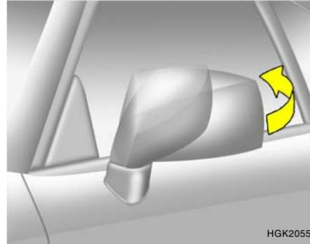
To fold the outside rear view mirrors, push them toward the rear. The outside rear view mirrors can be folded rearward for parking in narrow areas.
