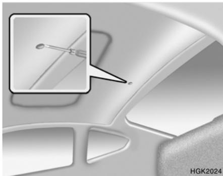
1. Remove the cap located in the rear roof panel by using a coin or screw driver.
