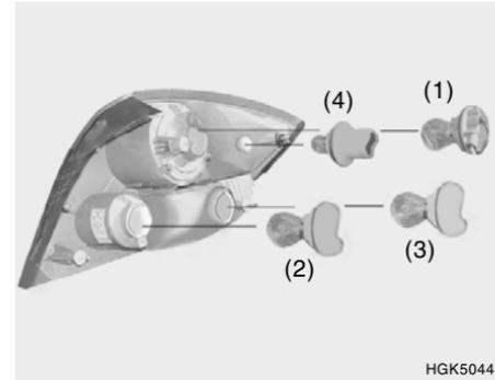
5. To replace the rear combination light (stop/tail light, back-up light, turn signal light, side mark light), take it out from the bulb holder by turning it counterclockwise.
