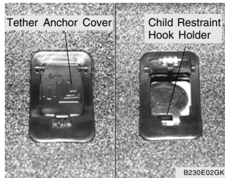
1. Open the tether anchor cover on the rear luggage compartment floor.
