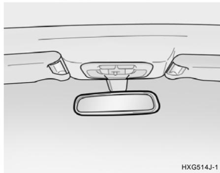
The electric type day/night inside rearview mirror automatically controls the glare of headlights of the car behind you. Adjust the rearview mirror to the desired position.
