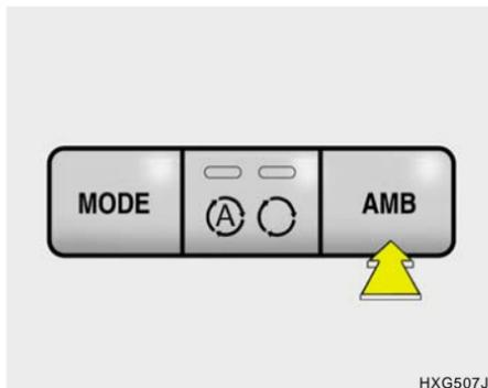
Pressing the AMB button displays the ambient temperature on the display.
