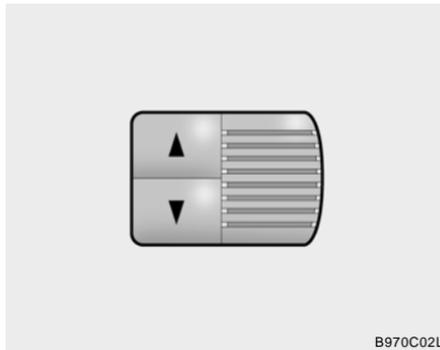
2. Push the "TEMP" button to set the desired temperature. The temperature will increase to the maximum 90°F(32°C) by pushing on the ▲ button. Each push of the button will cause the temperature to increase by 1°F (0.5°C). The temperature will decrease to the minimum 62°F(17°C) by pushing on the ▼ button. Each push of the button will cause the temperature to decrease by 1°F (0.5°C).
