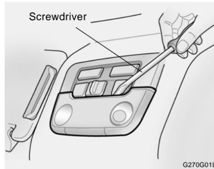
1. Remove the plastic cover with a flat blade screwdriver.
