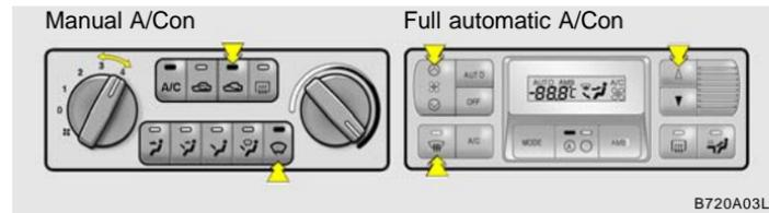
Use the heating/ventilation system to defrost or defog the windshield:
