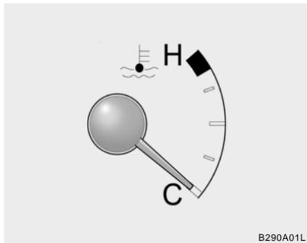
The needle on the engine coolant temperature gauge should stay in the normal range. If it moves across the dial to "H" (Hot), pull over and stop as soon as possible and turn off the engine. Then open the hood and, after the engine has cooled, check the coolant level and the water pump drive belt. If you suspect cooling system trouble, have your cooling system checked by Hyundai dealer as soon as possible.
