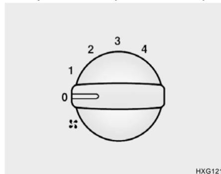
This is used to turn the blower fan on and off and to select the fan speed.
