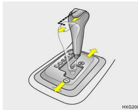
Whether the vehicle is stationary or in motion, sports mode is selected by pushing the selector lever from the "D" position into the manual gate. To return to "D" range operation, push the selector lever back into the main gate. In sports mode, moving the selector lever backwards and forwards can make rapid gearshifts simple. In contrast to a manual transaxle, the sports mode allows gearshifts with the accelerator pedal depressed.
