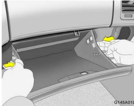
2. Lower the glove box completely by pushing the both sides of the glove box inward.
