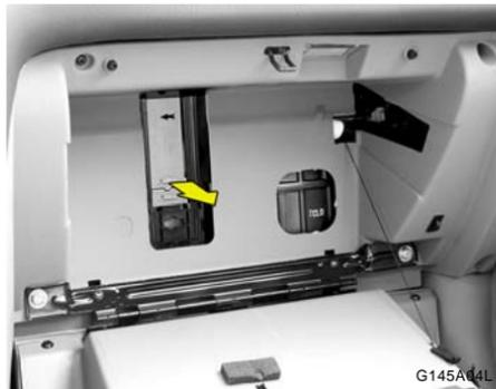
5. Remove the two air conditioner filters by pulling the knob of the air conditioner filter outward.
