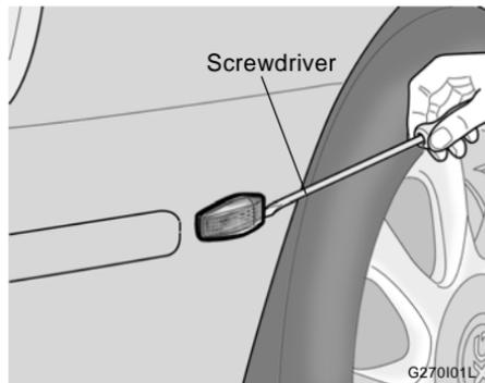
1. Remove the side marker light cover with a blade screwdriver.
