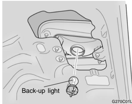
2. To replace the back-up light, remove it from the bulb holder and install the new bulb.
