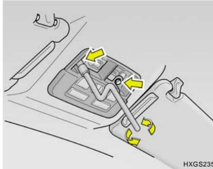
2. Remove the front overhead light and switch panel.
