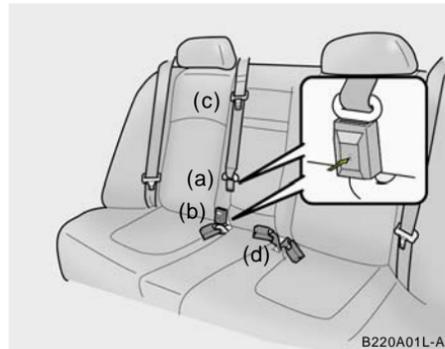
1. Before fastening the rear seat center belt, confirm the metal tab (a) and buckle (b) are latched together.
