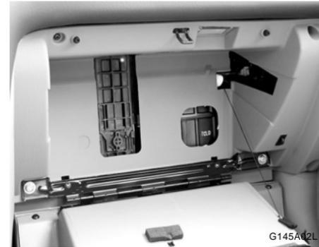
3. Lower the glove box down completely.
