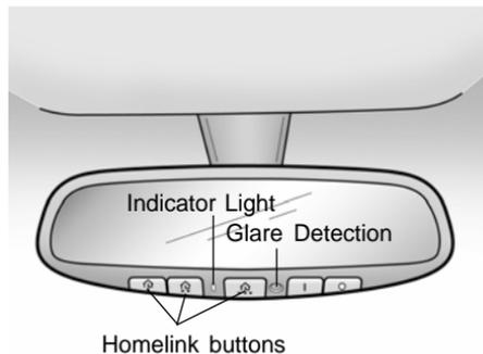
Your new vehicle may be equipped with an automatic night vision mirror. During nighttime driving, this feature will automatically detect and reduce dangerous rearview mirror glare.
