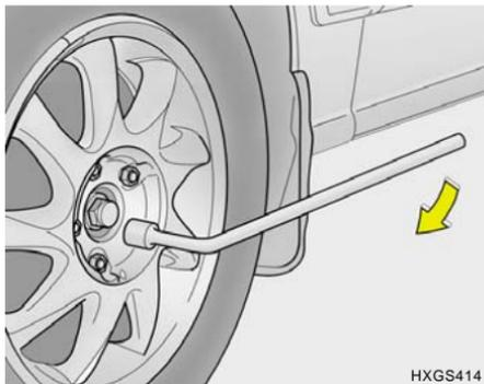
Lower the car to the ground by turning the wheel nut wrench counterclockwise. Then position the wrench as shown in the drawing and tighten the wheel nuts. Be sure the socket is seated completely over the nut. Do not stand on the wrench handle or use an extension pipe over the wrench handle.
