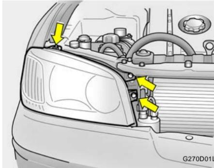
1. Remove the headlight assembly mounting bolts.
