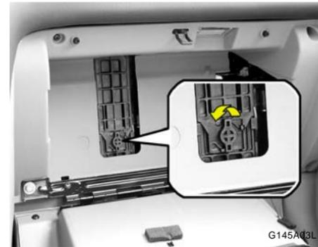
4. Turn the knob of the air conditioner filter cover counterclockwise and remove the air conditioner filter cover.
