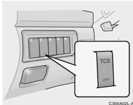
On slippery road surfaces, the traction control system (TCS) limits the drive wheels from spinning excessively, thus helping the car to accelerate. It also provides sufficient driving force and steering performance as the car turns at accelerated speeds.
