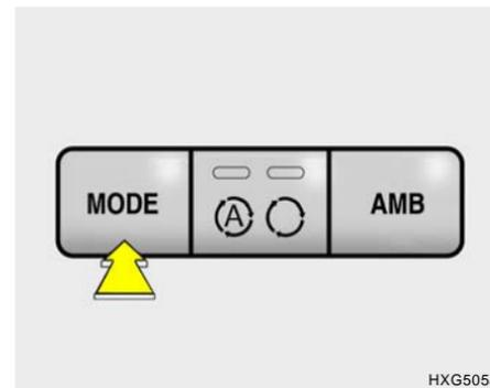
This is used to direct the flow of air. Air can be directed to the floor, dashboard outlets, or windshield. Four symbols are used to represent Face, Bi-Level, Floor and Floor-Defrost air position.
