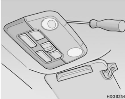
1. Remove the rectangular plastic interior light lens in the front of the roof panel.
