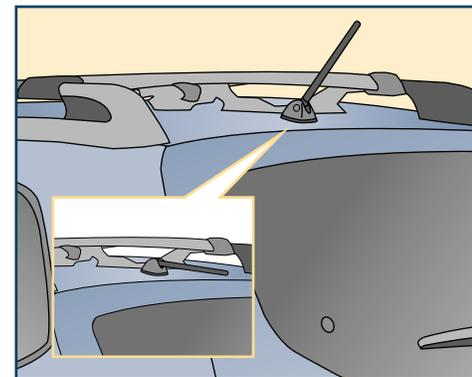
*Note: The antenna mast may be laid down flat when carrying over-size objects such as skis or surfboards.*
