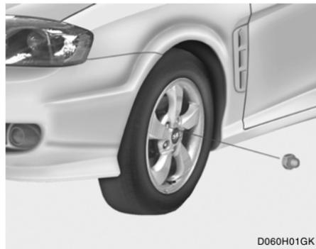
To reinstall the wheel, hold it on the studs, put the wheel nuts on the studs and tighten them finger tight. The nuts should be installed with their small di-
