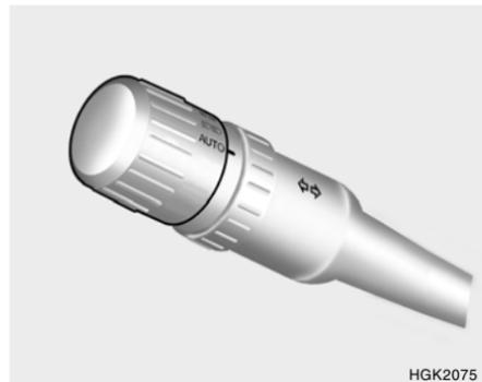
To operate the automatic light feature, turn the barrel on the end of the multi-function switch. If you set the multi-function switch to "AUTO", the tail lights and headlights will be turned automatically on or off according to external illumination.
