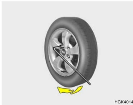
Lower the car to the ground by turning the wheel nut wrench counterclockwise. Then position the wrench as shown in the drawing and tighten the wheel nuts. Be sure the socket is seated completely over the nut. Do not stand
