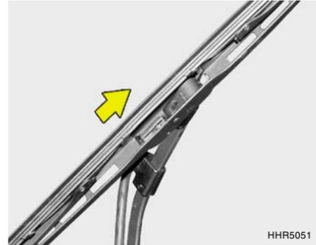
2. Pull up the wiper blade until you hear an audible "click" to engage in the end of the wiper arm.
