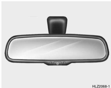
The electric type day/night inside rearview mirror automatically controls the glare of headlights of the car behind you.
