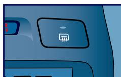
With the engine running, press the defroster switch to activate the rear window and outside rearview mirror heaters\*.
