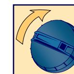
After adding fuel, always reinstall the fuel cap fully and make sure it clicks at least 3 times. Failure to do this may result in the "Check Engine Light" illuminating.
