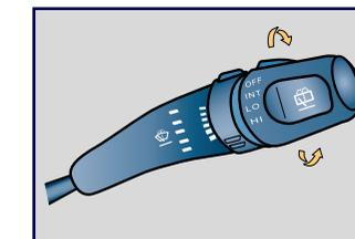
Rotate the right barrel switch to select the following rear window wiper/washer (if equipped) operation modes.
