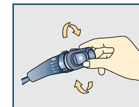
Rotate the right barrel switch to select the following rear window wiper/washer operation modes.
