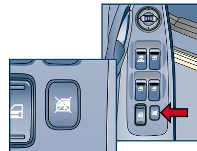
Pressing the lock switch **deactivates all of the power window switches except for the driver's window.**
