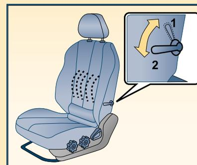
To adjust the lumbar support, move the lever on the outboard or left side of the seat to the desired position.
