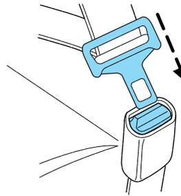
5. To put the retractor in the automatic locking mode, grasp the shoulder portion of the belt and pull downward until all of the belt is extracted and a click is heard.
