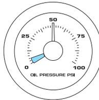
Do not continue to operate your engine as long as the pointer is in the red section. Otherwise, your engine may be severely damaged.
