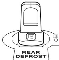
The rear window defroster turns off automatically after 10 minutes or when the ignition is turned to the 1 (OFF/LOCK) position. To manually deactivate the rear window defroster before 10 minutes, push the control forward again (the indicator lamp will turn off).
