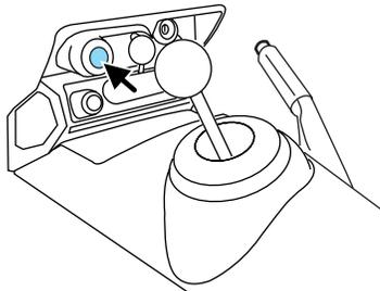
**Note:** If the engine does not start within five seconds on the first try, turn the key to 1 (OFF/LOCK), wait 10 seconds and try again. If the engine still fails to start, press the accelerator to the floor and try again; this will allow the engine to crank with the fuel shut off in case the engine is flooded with fuel.
