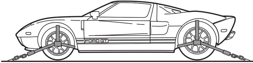
5. Transport the vehicle with the parking brake OFF and the transmission in NEUTRAL.
