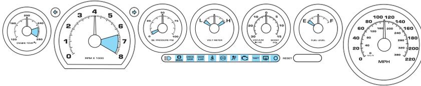
Warning lights and gauges can alert you to a vehicle condition that may become serious enough to cause expensive repairs. A warning light may illuminate when a problem exists with one of your vehicle's functions. Many lights will illuminate when you start your vehicle to make sure the lights work. If any light remains on after starting the vehicle, have the respective system inspected immediately.
