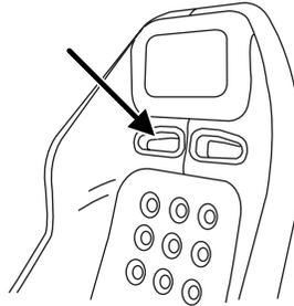
4. You may need to pull the seat forward to access the tether anchors.
