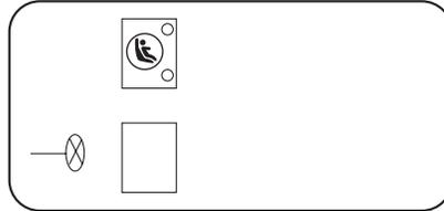
The lower anchors for child seat installation are located at the rear section of the passenger seat between the cushion and seat back. The seat back must be in the full rear position to access the LATCH anchors.
