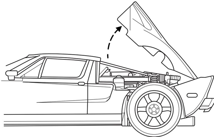
5. Lift the decklid and ensure that it is secure.
