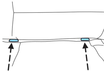
To attach a child seat to the lower anchors, place the vehicle seat in the full rear position and the seatback in upright position.
