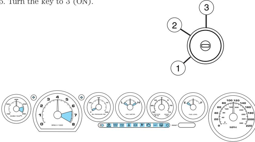
Make sure the corresponding lights illuminate or illuminate briefly. If a light fails to illuminate, have the vehicle serviced.
