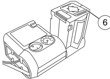
7. Turn the air compressor on by pressing the "I" side of the orange button.
