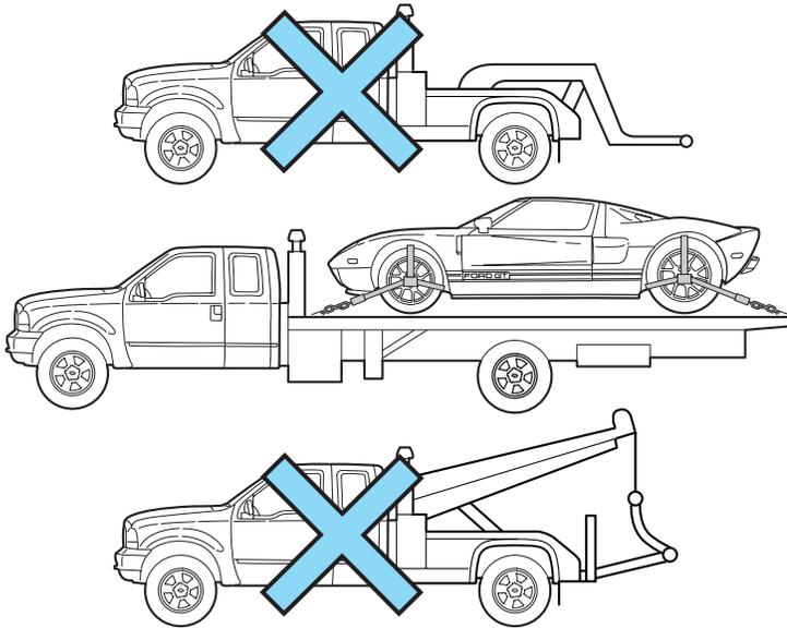
**Note:** Do not attempt to tow this vehicle from the rear. Ford Motor Company has not approved towing this vehicle from the rear.
