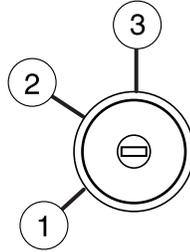
2. Turn the ignition from the 1 (OFF/LOCK) position to the 3 (ON) position. Keep the ignition in the 3 (ON) position for at least one second, but no more than 10 seconds.
