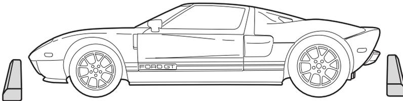
**Note:** Because of low vehicle ground clearance, use caution when approaching curbs/curb stops from front and rear — vehicle damage could occur.
