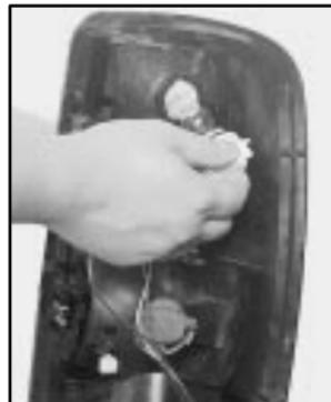
5. Press a new bulb into the socket, insert the socket into the taillamp housing and turn the socket clockwise into the taillamp housing until it clicks.
