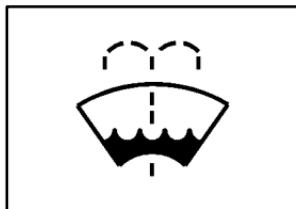
Open the cap with the washer symbol on it. Add washer fluid until the tank is full.
