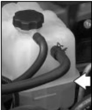
The coolant surge tank is located in the engine compartment on the passenger's side of the vehicle. See "Engine Compartment Overview" in the Index for more information on location.
