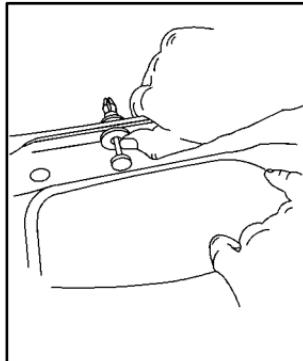
1. Line up each push-pin with its intended retainer and push the washer portion of the push-pin towards the retainer until it locks into place.
