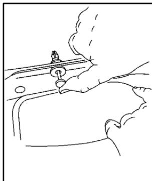
2. Push the flat end of the push-pin towards the retainer until it locks into place, making sure each is secure.
