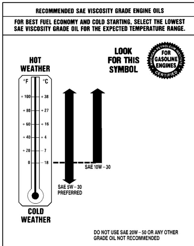
As in the chart shown previously, SAE 5W-30 is best for your vehicle. However, you can use SAE 10W-30 if it's going to be 0°F (-18°C) or above. These numbers on an oil container show its viscosity, or thickness. Do not use other viscosity oils, such as SAE 20W-50.
