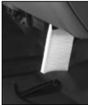
2. Next, pull downward on the filter retaining bracket.
