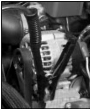
9. Connect the other end of the negative (-) cable to the negative (-) terminal of the dead battery or to a remote negative (-) terminal if the vehicle has one.
