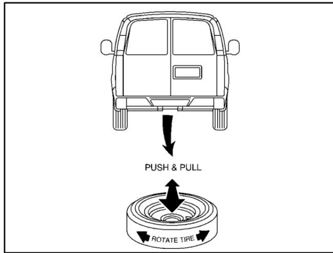
6. Make sure the tire is stored securely. Push, pull, and then try to rotate or turn the tire. If the tire moves, use the wheel wrench to tighten the cable.
