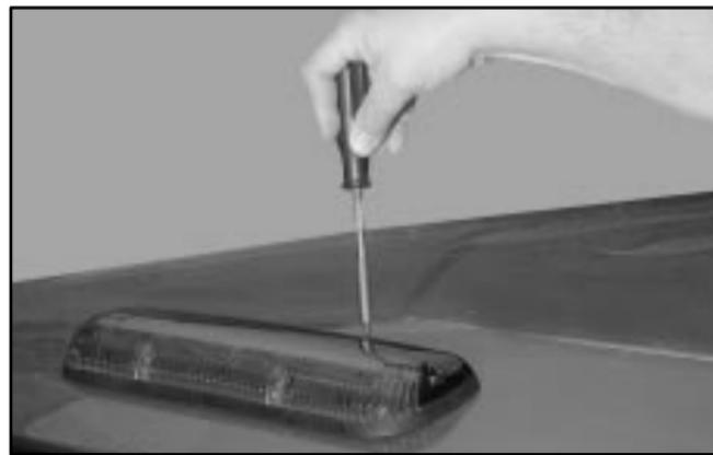
2. The center roof marker lamps has six screws to remove.
