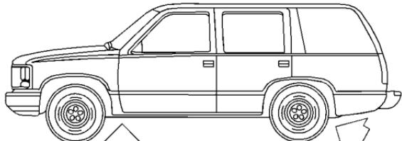
2. Position the jack under the vehicle. If the flat tire is on the front of the vehicle, position the jack on the frame behind the flat tire where the frame sections overlap.
