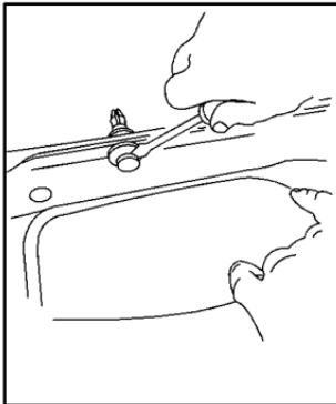
1. Insert a tool into the push-pin slot and pull downward until the push-pin snaps loose.
