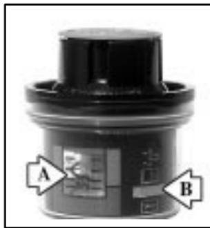
The service window A with the percentage scale shows the amount of engine air cleaner/filter life used. When both service window A and service window B turn orange, replace the engine air cleaner/filter.
