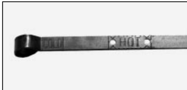
3. Check both sides of the dipstick, and read the lower level. The fluid level must be in the COLD area, below the cross-hatched area, for a cold check or in the HOT area or cross-hatched area for a hot check.
