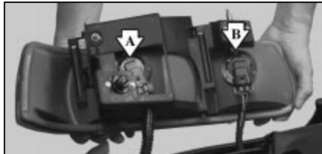
1. Remove the two pins on the top of the headlamp assembly. To remove the pins, turn the outer pin outward and pull it straight up. To remove the inner pin, turn it in and pull it straight up.
