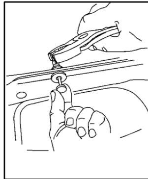
2. While continuing to pull downward on the push-pin, squeeze and turn the expandable end of the push-pin with a tool until it releases from the retainer.
