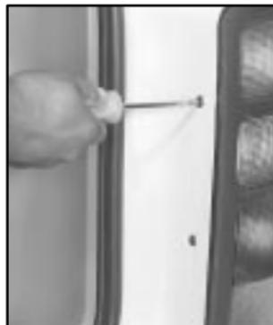
1. Use a tool to remove the two screws from the lamp assembly.
