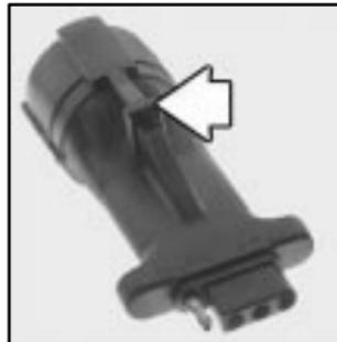
Connect the adapter with the tab (arrow) pointing toward the top. The cap on the wiring harness will lock onto the tab (arrow) and help hold the adapter in place.
