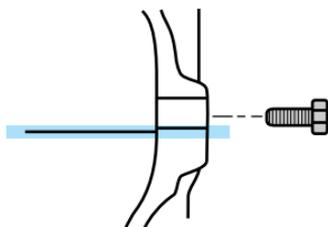
4. Add enough fluid through the filler opening so that the fluid level is at the bottom of the opening.
