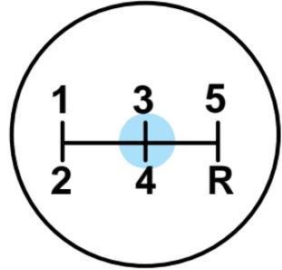
**NOTE:** You can shift into R (Reverse) only by moving the gearshift lever from left of 3 (Third) and 4 (Fourth) gears before you shift into R (Reverse). This is a special lockout feature which prevents you from shifting into R (Reverse) when you downshift from 5 (Fifth).
