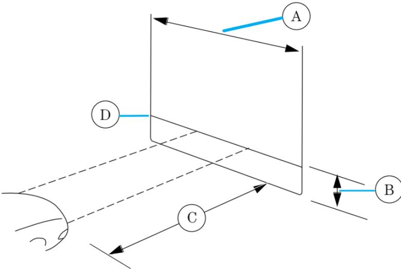
2. Measure the height from the center of your headlamp to the ground and mark a 2.4 meter (8 foot) horizontal reference line on the vertical wall or screen at this height (a piece of masking tape works well). The center of the lamp is marked by a 3.0 mm circle on the headlamp lens.
