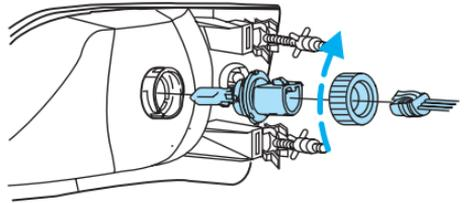
**NOTE:** If the bulb is accidentally touched, it should be cleaned with rubbing alcohol before being used.
