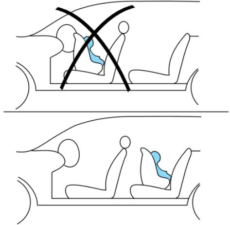
**WARNING:** Air bags can kill or injure a child in a child seat. NEVER place a rear-facing child seat in front of an active air bag. If you must use a forward-facing child seat in the front seat, move the seat all the way back and secure it properly.
