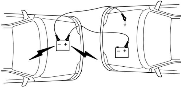
4. Make the final connection of the negative (-) cable to an exposed metal part of the disabled vehicle's engine, away from the battery and the fuel injection system. **NOTE: Do not** use fuel lines, engine rocker covers or the intake manifold as *grounding* points.
