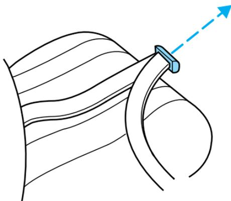
**Shorten and fasten the belt when not in use to keep the belt away from door openings and available after unfolding the seats.**
