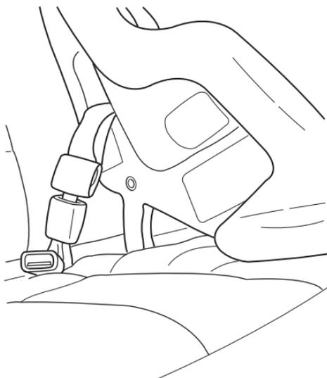
Mazda recommends the use of a child safety seat having a top tether strap. Install the child safety seat in a seating position which is capable of providing a tether anchorage. For more information on top tether straps, refer to *Attaching child safety seats with tether straps*.
