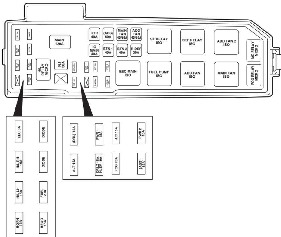
The high-current fuses are coded as follows.
