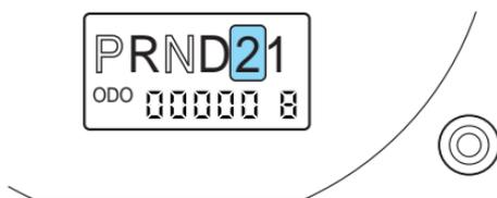
**To avoid damage to the engine and/or transaxle do not go faster than 108 km/h (68 mph) when in this gear. You can upshift from 2 (Second) to overdrive at any time.**
