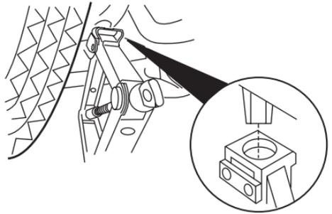
6. Position the jack according to the following guides and turn the jack handle clockwise until the tire is a maximum of 25 mm (1 inch) off the ground.
