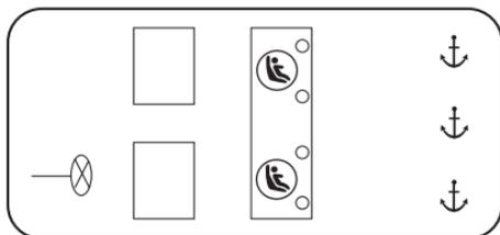
**WARNING: Do not attach a child seat to any lower anchors used for child seat installation if an adjacent child seat is attached to that anchor. In a crash, one anchor may not be strong enough to hold two child seat attachments and may break, causing serious injury or death.**
