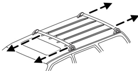
3. Use a long, flat object in order to depress the tongue in the endcaps on both sides of the cross-bar.
