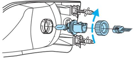
5. Squeeze the retainer spring together releasing it from bulb hooks and rotate it away from the bulb.
