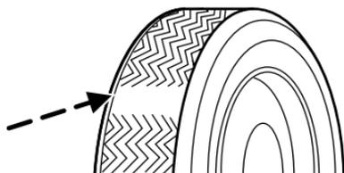
**WARNING:** When replacing full size tires, never mix radial bias-belted, or bias-type tires. Use only the tire sizes that are listed on the Certification Label. Make sure that all tires are the same size, speed rating, and load-carrying capacity. Use only the tire combinations recommended on the label. If you do not follow these precautions, your vehicle may not drive properly and safely and an accident can occur.
