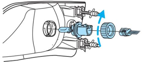
6. Without turning, carefully pull bulb out of headlamp assembly.
