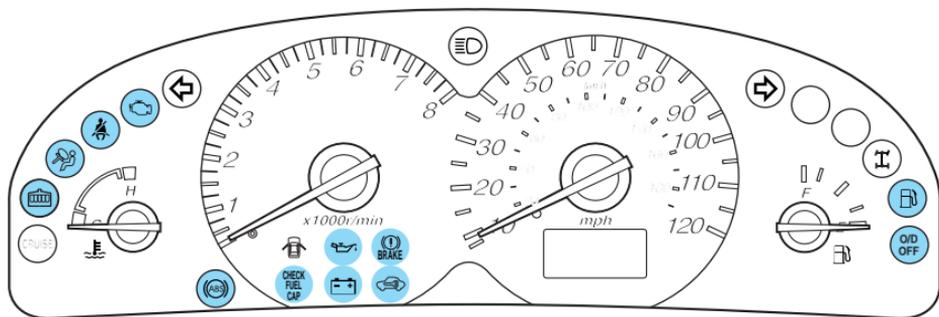
Make sure the corresponding lights illuminate or illuminate briefly. If a light fails to illuminate, have the vehicle serviced.
