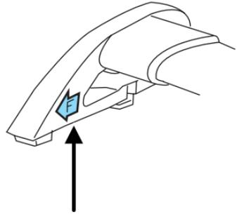
2. Use a long, flat object to depress the tongue in the endcaps on both sides of the cross-bar.
