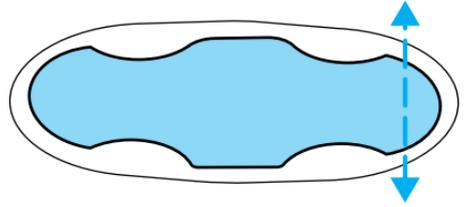
Move the control in the directions shown to move the seat forward, backward, up or down.
