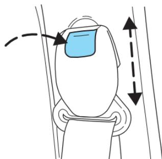
**WARNING: Position the shoulder belt height adjusters so that the belt rests across the middle of your shoulder. Failure to adjust the safety belt properly could reduce the effectiveness of the seat belt and increase the risk of injury in a collision.**
