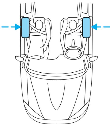
**NOTE:**A side air bag, in combination with seat belts, can help reduce the risk of severe injuries in the event of a significant side impact collision.
