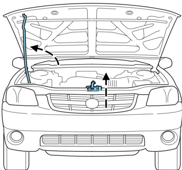
2. At the front of the vehicle, lift up on the auxiliary latch handle located in the center between the hood and the grille.
