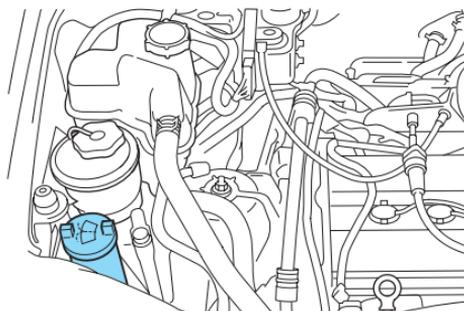
Only use a washer fluid that meets Mazda specifications. Refer to *Lubricant specifications* in the *Capacities and specifications* chapter.
