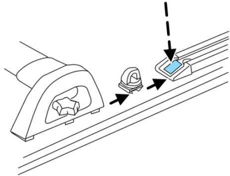
3. Slide the tie down loops and the cross-bar assemblies over the end cap tongue and into the side rails.
