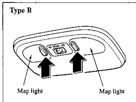
The map lights are switched on or off by pressing the switches.
