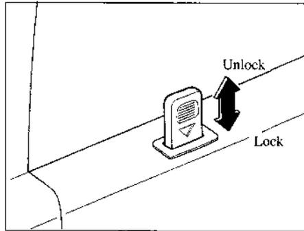
■ **Locking, Unlocking with Door-Lock Button**
