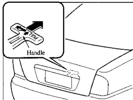
To open the trunk lid from the inside, pull the illuminated "T" shaped handle. The handle is made of material that will glow for hours in the darkness of the trunk following a brief exposure to ambient light.
