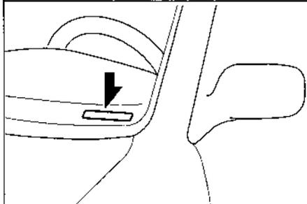
The vehicle identification number legally identifies your vehicle. The number is on a plate attached to the left top side of the dashboard. This plate can easily be seen through the windshield.
