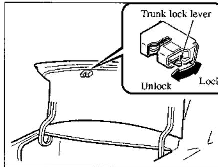
To secure the trunk lid, lock the rear seatbacks (page 2-8), push the trunk lock lever up, and close the trunk.
