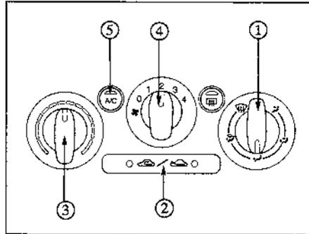
3. Set the temperature control dial to the desired position.
