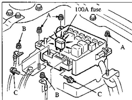
When replacing the 100A fuse:
