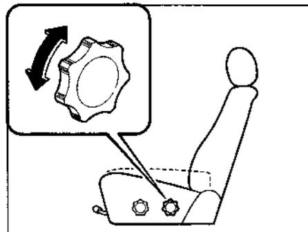
The seat-bottom angle can be adjusted by rotating the dial. The rear dial tilts the rear of the seat bottom upward.
