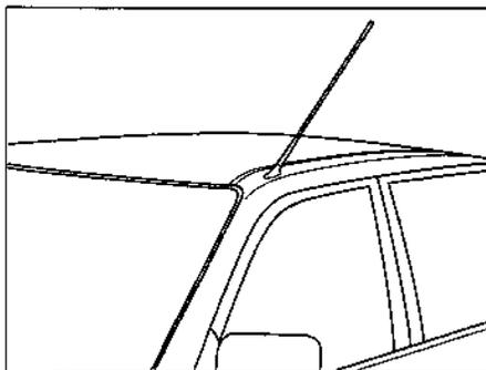
The manual antenna must be raised and lowered by hand.
