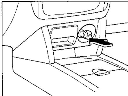
To operate the lighter, press it in and release it. When ready for use, it automatically pops out.
