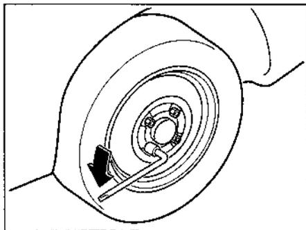
8. Loosen the lug nuts by turning them counterclockwise one turn each, but don't remove any until the tire has been raised off the ground.
