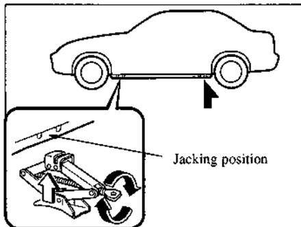
9. Place the jack under the jacking position closest to the tire being changed.
