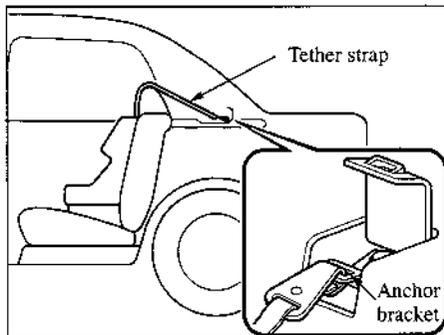
3. If your child-restraint system came equipped with a tether, that probably means it is very important to properly secure the tether for child safety, please carefully follow the child-restraint system manufacturer's instructions when installing tethers. Only the 3 rear seat positions on this vehicle are set up for tethers, all LATCH child-restraint systems are fully compatible only with the two rear outboard seats.
