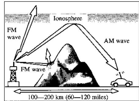
Signals from an FM transmitter are similar to beams of light because they do not bend around corners, but they do reflect. Unlike AM signals, FM signals cannot travel beyond the horizon. Therefore, FM stations cannot be received at the great distances possible with AM reception.
