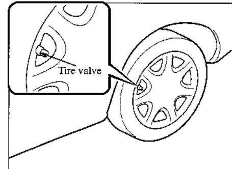
7. Pry off the wheel cover\* with the beveled end of the lug wrench.
