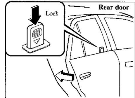
To lock any door with the door-lock button from the outside, push down the door-lock button and close the door.
