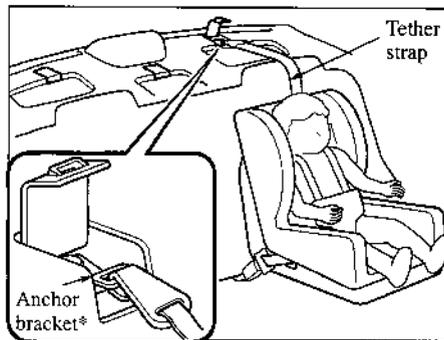
4. If your child-restraint system requires the use of a tether strap, hook the tether strap by following the manufacturer's instructions.
