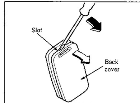
▼ Replacing the transmitter battery
