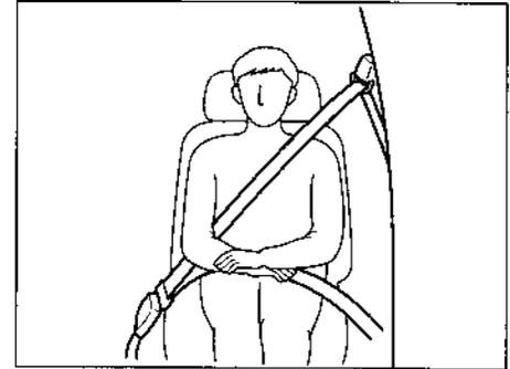
Adjust the height of the shoulder belt if the seat belt touches your neck, if it crosses your arm instead of your shoulder. To raise the shoulder belt adjuster, push the adjuster up. To lower the shoulder belt adjuster, push the button slide it down. Make sure the adjuster is locked.
