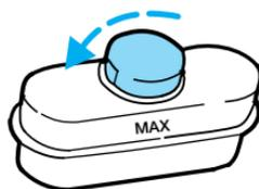
4. Use only brake fluids certified to meet Ford specification ESA-M6C25-A. Refer to *Lubricant specifications* in the *Capacities and specifications* chapter. DOT 3 fluid is recommended. However, if DOT 3 is not available, DOT 4 fluid can be used.
