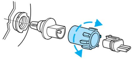
7. Without turning, remove the old bulb from the lamp assembly by gently pulling it straight back out of the lamp assembly.
