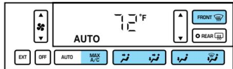
The air conditioning compressor can operate in all modes except
