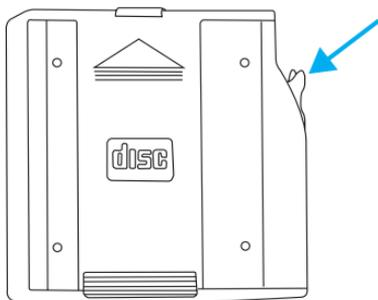
4. Insert one disc into each CD tray of the magazine (up to 6 discs). Ensure that the label side is facing up.
