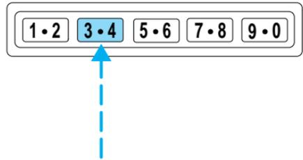
To release the trunk, enter the factory-set code or personal code (driver door unlocks) and press 5/6 within five seconds.
