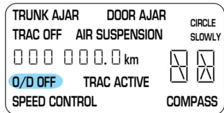
The light may also flash steadily if a transmission malfunction is detected. If the light does not come on when the Transmission Control Switch is depressed or if the light flashes steadily, have your vehicle serviced as soon as possible, damage to the transmission could occur.
