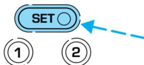
Manually moving any seat, mirror or pedal during these steps will cancel the programming procedure.
