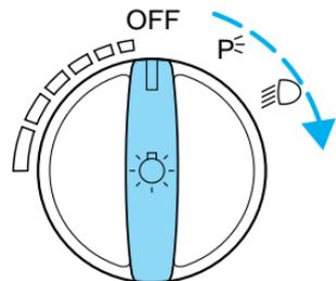
Your vehicle's headlamp system is equipped with a feature that will **not** dim the instrument panel lighting when the headlights are on in the daytime. Even during full daylight, the instrument panel lighting will still be visible with the headlamp operating.
