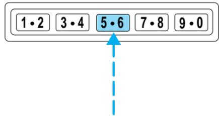
After the factory-set code or personal code has been entered, you can unlock all doors (press 3/4) and release the trunk (press 5/6) as long as the controls are pressed within five seconds of each other.
