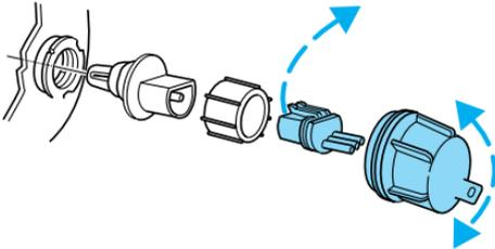
4. Disconnect the electrical connector from the bulb by pulling rearward.
