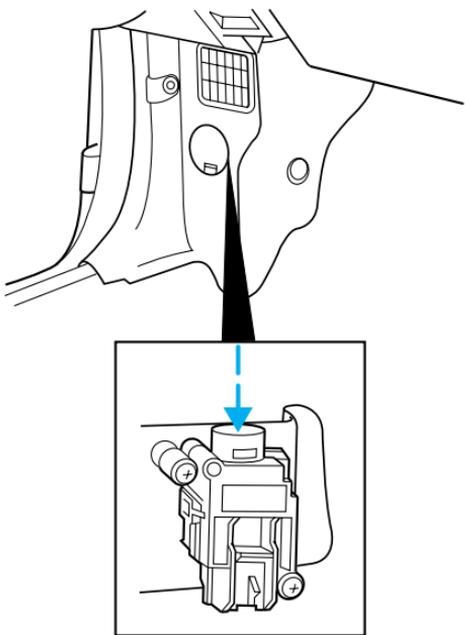
The fuel pump shut-off switch, depending on application, is located on the right side of the trunk behind the trunk liner or in the driver's foot well, behind the kick panel.
