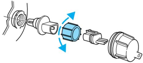
6. Without turning, remove the old bulb from the lamp assembly by pulling it straight back out of the lamp assembly and replace.
