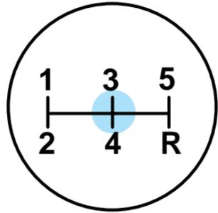
You can shift into R (Reverse) only by moving the gearshift lever from left of 3 (Third) and 4 (Fourth) gears before you shift into R (Reverse). This is a special lockout feature which prevents you from shifting into R (Reverse) when you downshift from 5 (Fifth).
