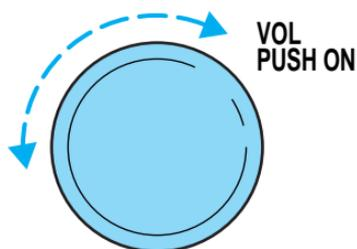
If the volume is set above a certain level and the ignition is turned off, the volume will come back on at a “nominal” listening level when the ignition switch is turned back on. If you wish to maintain your preset volume level, turn the audio system off with the power control before switching off the ignition.
