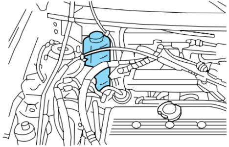
Check the washer fluid whenever you stop for fuel. The reservoir is highlighted with a
