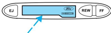
You can switch from CD (if equipped) to tape play by inserting a tape into the cassette deck.
