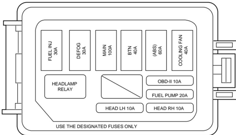
The high-current fuses are coded as follows.
