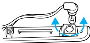
To install the brakelamp bulb:
