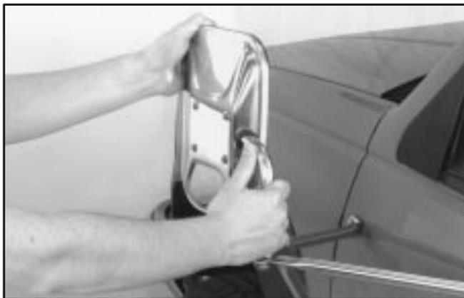
1. To adjust the mirrors when hauling a slide-in camper or towing a trailer, turn the mirror by pushing the mirror head toward the front of the vehicle.
