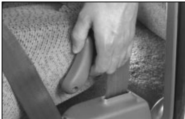
To adjust the front seatback, move the lever rearward. Release the lever to lock the seatback where you want it. Move the lever again rearward and the seatback will go to an upright position.
