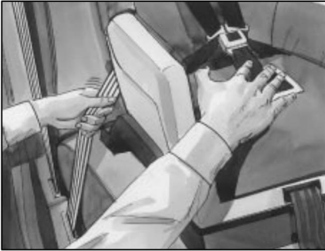
5. To tighten the belt, feed the lap belt back into the retractor while you push down on the child restraint. If you're using a forward-facing child restraint, you may find it helpful to use your knee to push down on the child restraint as you tighten the belt.
