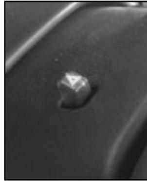
Press the button located at the top of the steering column all the way down to make your front and rear turn signal lamps flash on and off.
