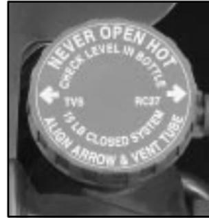
8. Then replace the pressure cap. At any time during this procedure if coolant begins to flow out of the filler neck, reinstall the pressure cap. Be sure the arrows on the pressure cap line up like this.
