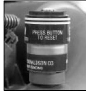
The engine air cleaner/filter assembly has an indicator that lets you know when the engine air cleaner/filter is dirty and needs to be serviced. The indicator is located in the air intake tube between the engine air cleaner/filter and the engine.
