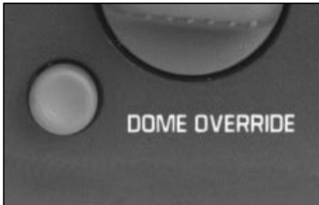
You can use the DOME OVERRIDE button, located below the parking lamp and headlamp knob, to set the dome lamp to come on automatically when a door is opened, or to remain off. To turn the lamp off, press the button “in”. Press the button again and return it to the “out” position to set the dome light to come on.
