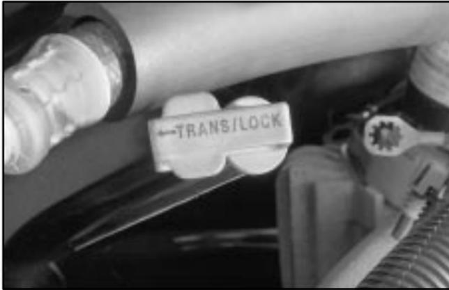
1. The red transmission dipstick handle is located at the rear of the engine compartment, on the passenger's side. See "Engine Compartment Overview" in the Index for more information on location. Flip the handle up and then pull out the dipstick and wipe it with a clean rag or paper towel.
