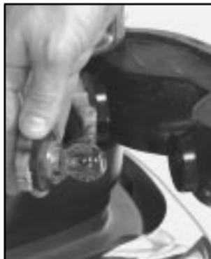
4. Pull the socket out of the lamp assembly.
