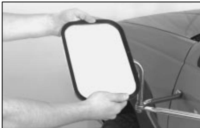
2. Turn the mirror head, so that the mirror surface faces the rear of the vehicle.
