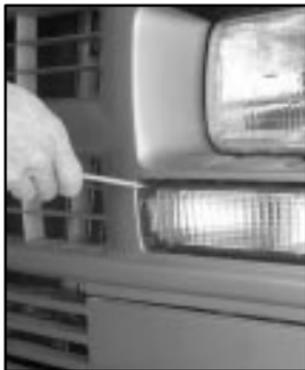
1. Remove the two screws at the inside edge of the parking/turn signal lamp assembly.
