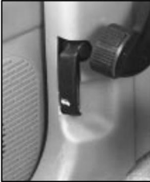
To open the hood, first pull the handle located near the lower left side of the instrument panel.
