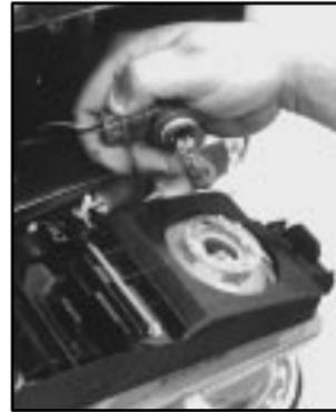
4. Turn the bulb counterclockwise and remove it.
