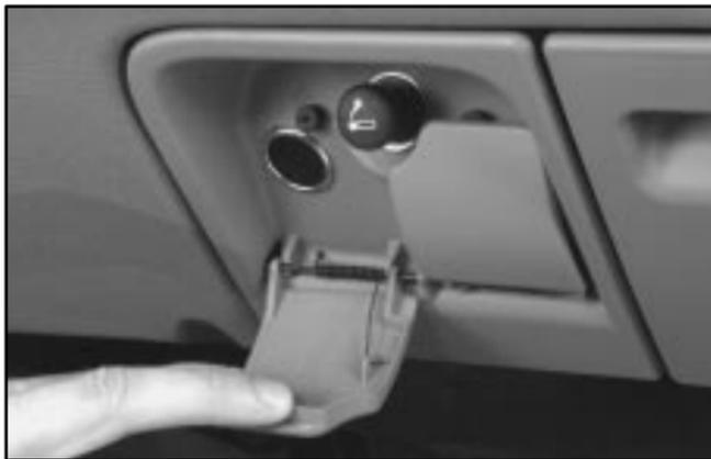
Two accessory power outlets are located near the cigarette lighter. Use these outlets to power mobile telephones or other devices designed to operate with vehicle electrical systems.
