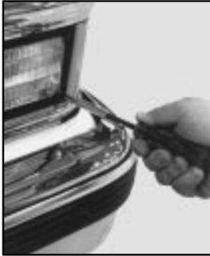
1. Remove the two screws and take out the parking/turn signal lamp assembly.
