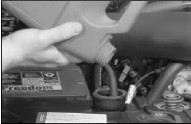
3. Fill the radiator with the proper DEX-COOL<sup>®</sup> coolant mixture, up to the base of the filler neck. See “Engine Coolant” in the Index for more information about the proper coolant mixture.
