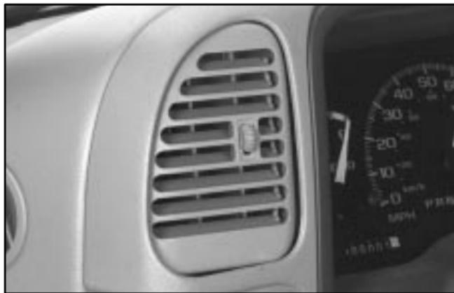
Your vehicle has air outlets in the center and on the sides of your instrument panel. You can move the outlets from side-to-side or up and down to direct the flow of air, or close the outlets altogether. When you close an outlet, it will increase the flow of air coming out of any outlets that are open. These outlets do not completely shut off airflow when in the closed position.
