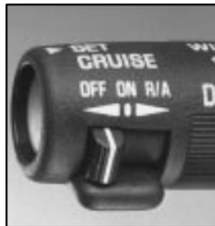
With cruise control, you can maintain a speed of about 25 mph (40 km/h) or more without keeping your foot on the accelerator. This can really help on long trips. Cruise control does not work at speeds below about 25 mph (40 km/h).
