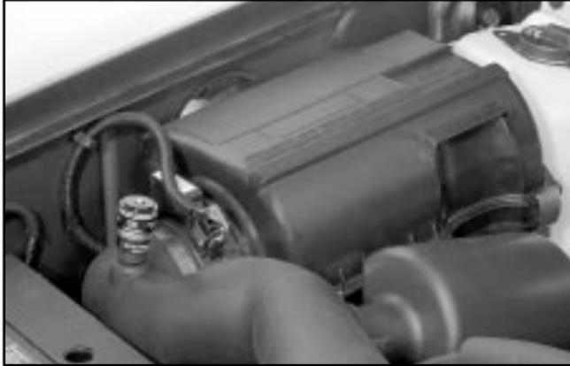
Your engine air cleaner/filter is located between the battery and coolant recovery tank.
