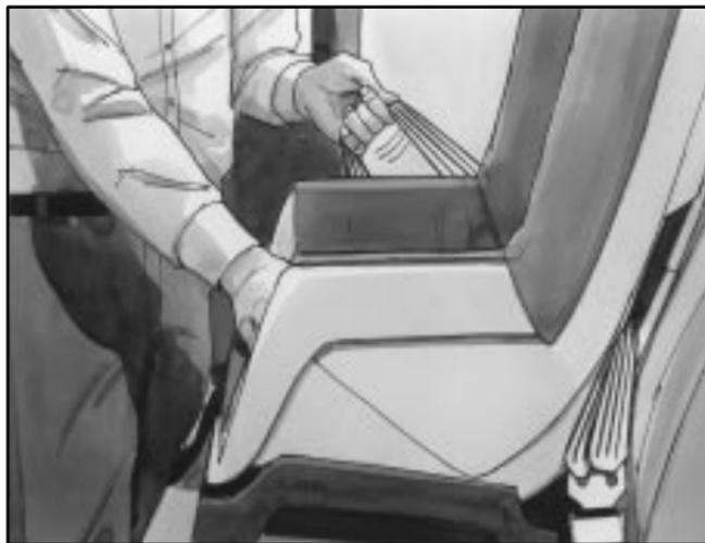
4. Pull the rest of the lap belt all the way out of the retractor to set the lock.
