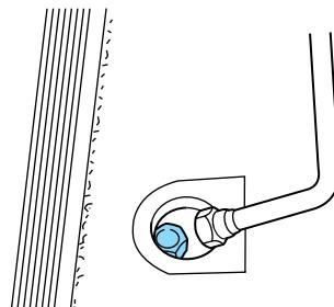
3. Turn the wrench counterclockwise until tire is lowered to the ground and the cable is slightly slack.
