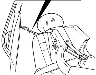
3. Adjust the tether strap length until the hook is about one foot behind the seatback.
