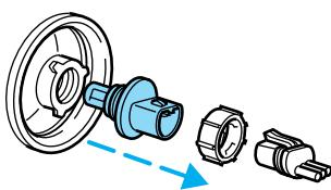
1. With the flat side of the new bulb's plastic base facing upward, insert the glass end of the bulb into the lamp assembly. Turn the bulb left or right to align the grooves in the plastic base with the tabs in the lamp assembly. When the grooves are aligned, push the bulb into the lamp assembly until the plastic base contacts the rear of the lamp assembly.
