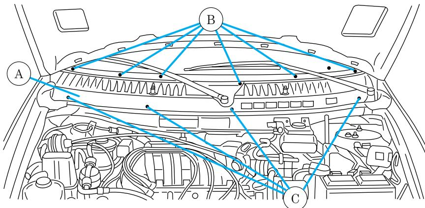
2. Remove the six (6) screws (B) from the cowl grille (A) at the base of the windshield.
