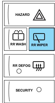
Press the washer control to activate the rear washer. The wiper will come on when the washer control is pressed, if it is not already on.
