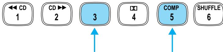
To turn on the rear seat controls, press the memory preset controls 3 and 5 at the same time. The
