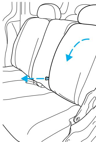
2. Grasp the child seat at the top of the seatback and pull the top forward to release the latch.
