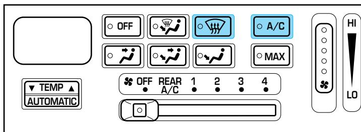
Press the (A/C) and (DEF) simultaneously for one second while rotating the fan speed dial upward until it stops moving, to switch between Fahrenheit and Celsius.
