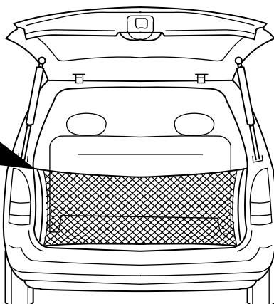
The cargo net helps stabilize lightweight objects in the cargo area. Attach the net to the anchors provided. The cargo restrained in the net must not exceed 22 kg (50 lbs.) or the net may not stay secured.
