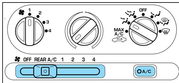
1. Set the main climate control rear fan control to Rear A/C, set the mode selector in any position (other than OFF), and depress the A/C control.
