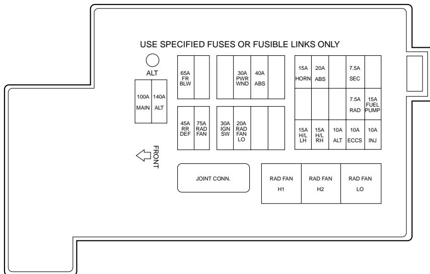
The high-current fuses are coded as follows.
