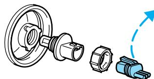
3. Remove the bulb retaining ring by rotating it counterclockwise (when viewed from the rear) to free it from the bulb socket, and slide the ring off the plastic base. Keep the ring to retain the new bulb.
