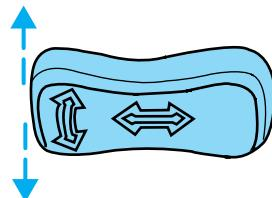
Slide the control forward or backward to move the seat forward or backward.
