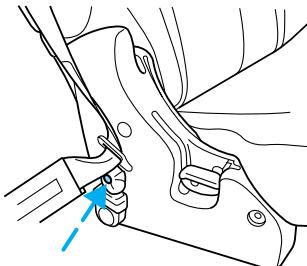
2. From behind the seat, pull up on the release straps located on each side of the seat, releasing the rear floor latches.
