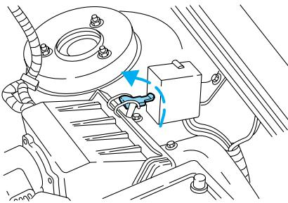
4. Install a new air filter element. Be careful not to crimp the filter element edges between the air filter housing and cover. This could cause filter damage and allow unmetered air to enter the engine if not properly seated.
