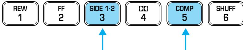
To turn on the rear seat controls, press the memory preset controls 3 and 5 at the same time. The will appear in the radio display.
