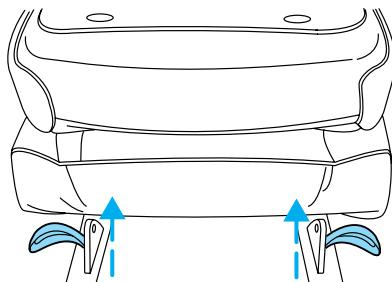
3. Lift up the back of the seat to clear the floor latches and then pull the seat rearward until the front hooks have come out of the floor anchors.
