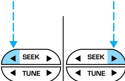
To set the minute, press and hold the CLK control and press the TUNE control:
