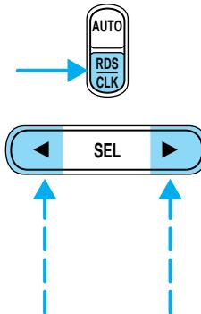
To set the minute, press the RDS/CLK control until SELECT MIN is displayed and press:
