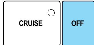
Once speed control is switched off, the previously programmed set speed will be erased.
