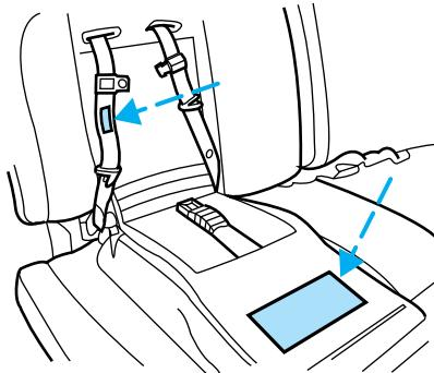
5. If connected, squeeze the top and the bottom of the right half of the chest clip and pull to separate both halves and unbuckle the two safety belt tongues from the crotch belt buckle.
