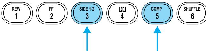
To turn on the rear seat controls, press the memory preset controls 3 and 5 at the same time. The
