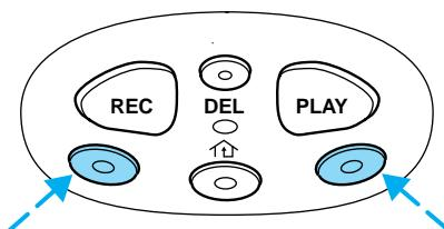
2. Hold the end of your hand-held transmitter 5–14 cm (2–5 inches) away from the HomeLink® Universal Transceiver surface (located on your visor) while keeping the red light in view.
