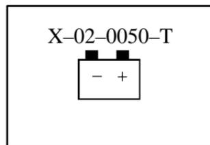
This light will come on briefly when you turn on the ignition, but the engine is not running, as a check to show you it is working. Then it should go out when the engine starts.
