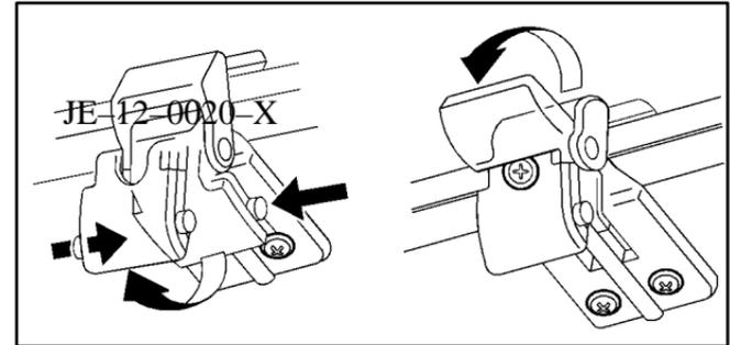
2. Squeeze the front top bow latch buttons and pull the latch back.
