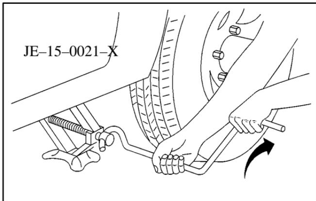
3. Raise the vehicle by turning the jack handle clockwise. Raise the vehicle far enough off the ground so there is enough room for the spare tire to fit.
