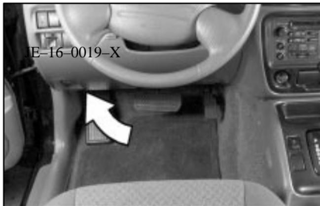
This fuse box is under the left side of the instrument panel. The fuses here protect each separate circuit including headlamps. If you have electrical failure, check here first.
