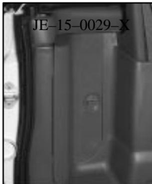
To open the jacking tool storage compartment, turn the knob counterclockwise.
