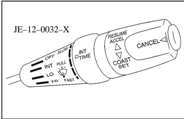
The lever on the right side of the steering column controls the windshield wipers and washers.
