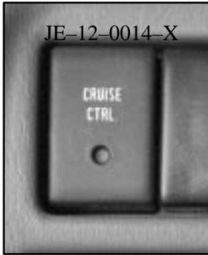
1. Press the CRUISE CTRL. switch on the instrument panel to turn the system on. The indicator light on the switch will come on.
