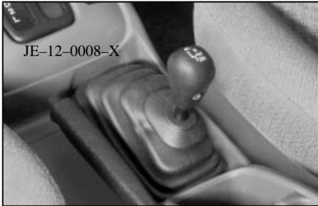
The transfer case shift lever is on the floor to the right of the driver. Use this lever to shift into and out of four-wheel drive. An indicator light comes on when the transfer case is in FOUR-WHEEL HIGH (4H) or FOUR-WHEEL LOW (4L).
