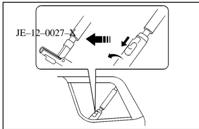
4. Push the release latches on both sides of the vehicle down to release the rear support arms. With the latches released, pull up on the arms at the hinges to release the tension on the canvas top.
