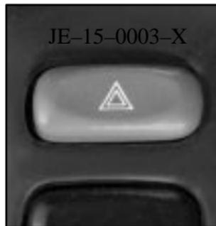
Press the button on the instrument panel to make your front and rear turn signal lamps flash on and off.
