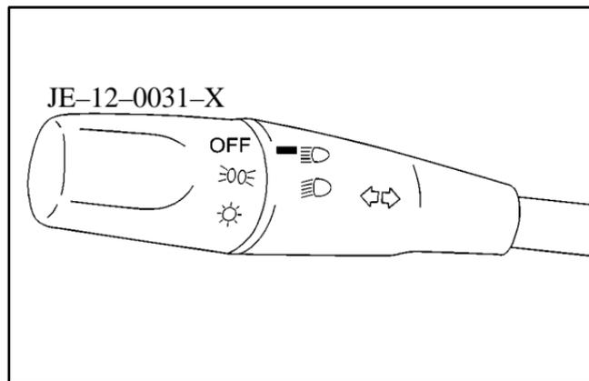
Turn the outside part of the lever to control the lamps. There are three positions for the lamp switch.
