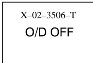
This light comes on when the automatic four-speed transmission has been converted to the three-speed mode and the overdrive is turned off.
