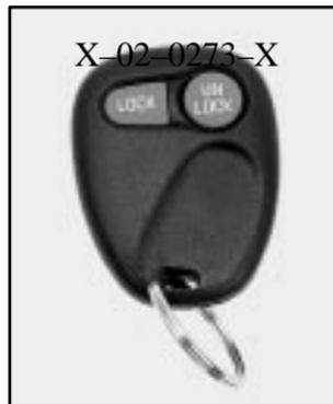
If your vehicle is equipped with this feature, you can lock and unlock your doors or unlock your rear door from about 3 feet (1 m) up to 30 feet (9 m) away using the remote keyless entry transmitter supplied with your vehicle.
