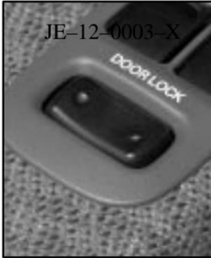
If you have power door locks, the switch is located on the driver's and passenger's door armrest.
