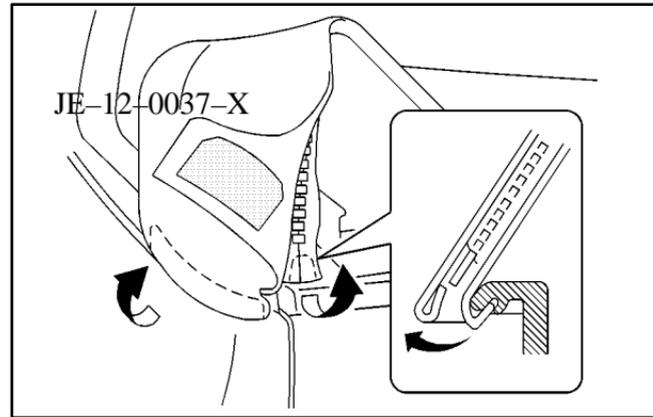
2. Loosen the lower rear corners of the convertible top.
