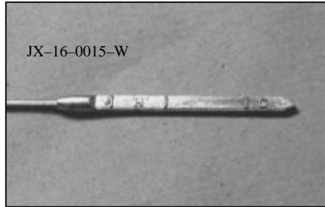
3. Check both sides of the dipstick, and read the lower level. The fluid level must be in the COLD area, below the cross-hatched area, for a cold check or in the HOT area or cross-hatched area for a hot check.
