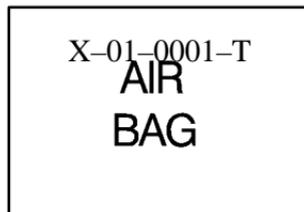
This light will come on when you start your engine, and it will flash for a few seconds. Then the light should go out. This means the system is ready.
