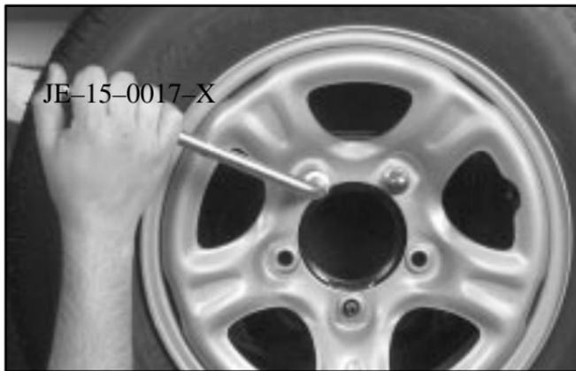
3. Remove the remaining wheel nuts from the spare tire with the wheel wrench.
