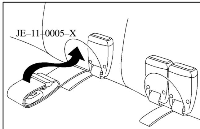
1. Fold the seat belt buckles and center safety belt (if equipped) into the pocket of the rear seatback.
