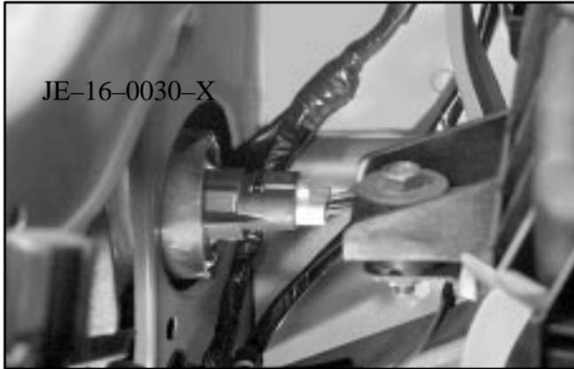
1. Open the hood and locate the turn signal bulb.
