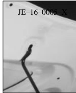
Lift the hood, release the hood prop from its retainer and put the hood prop into the slot in the hood.
