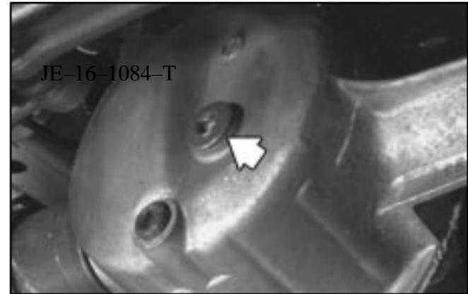
If the level is below the bottom of the filler plug hole, you may need to add some lubricant.
