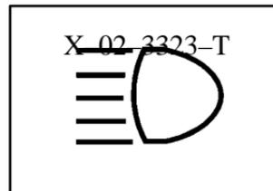
When the high beams are on, a light on the instrument panel also will be on. It will go off when you switch to low beam.
