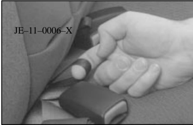
2. Pull the release straps located near the center of the vehicle to release the seat cushion. Fold the seat cushion forward.
