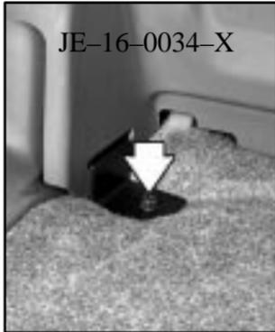
1. Remove the two attaching screws from each lower corner of the cargo area.
