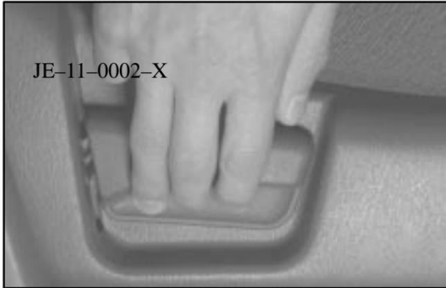
To adjust the seatback, lift the lever on the outer side of the seat. Release the lever to lock the seatback where you want it. Pull up on the lever, and the seat will go to its original upright position.
