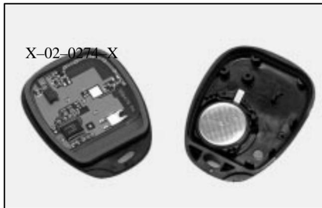
To replace the battery in the transmitter:
