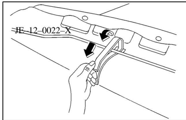
5. Unfasten the holding strap near the dome lamp and pull it through the slot in the front top bow.
