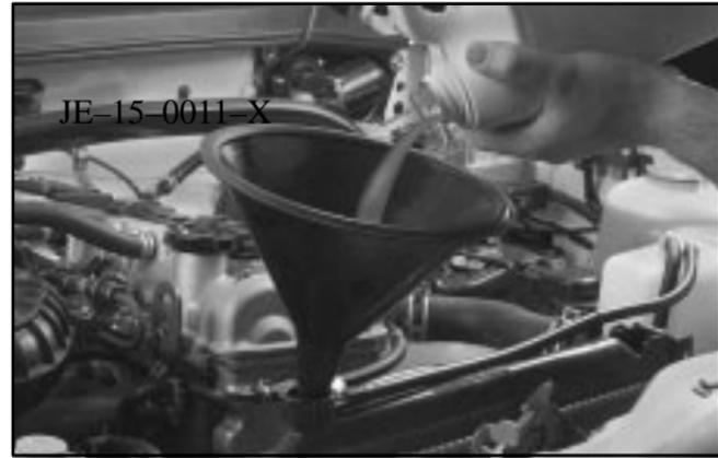
3. Fill the radiator with the proper coolant mixture, up to the base of the filler neck. (See “Engine Coolant” in the Index for more information about the proper coolant mixture.)
