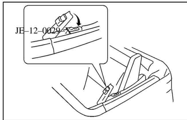
6. Reengage the latches by pushing down on the support arms at the hinges.
