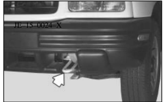
Your vehicle is equipped with recovery hooks. The recovery hooks are provided at the front and rear of your vehicle. You may need to use them if you're stuck off-road and need to be pulled to some place where you can continue driving.
