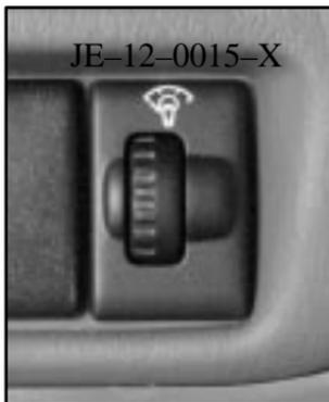
The thumbwheel controls the brightness of your instrument panel lights. Rotate the wheel upward to brighten the lights or downward to dim them.
