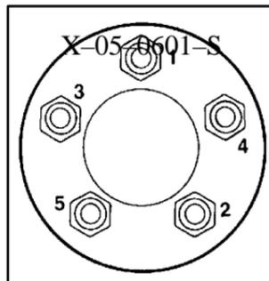
9. Tighten the wheel nuts firmly in a crisscross sequence as shown.
