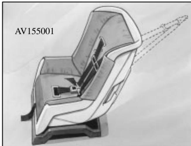
If your child restraint has a top strap, it should be anchored. If you have a two-door model, don't use a restraint like that in your vehicle because the top strap anchor cannot be installed properly. You shouldn't use this type of restraint without anchoring the top strap.
