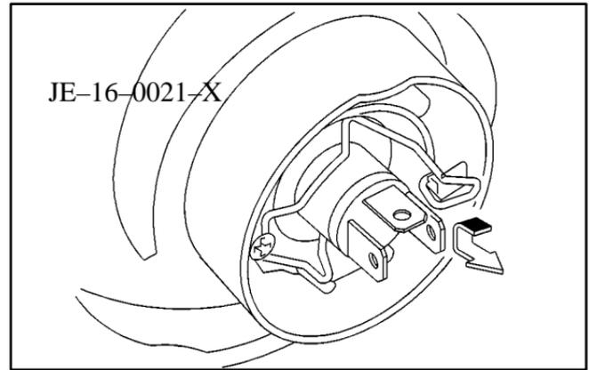
3. Release the retainer clip holding the bulb by pressing down and moving the metal retainer away from you.
