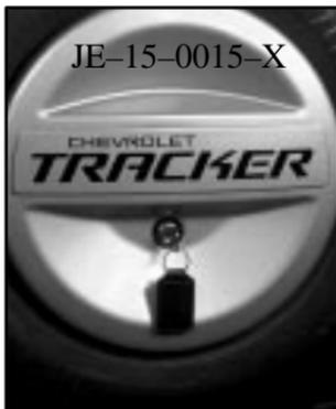
1. The spare tire is mounted on your tailgate. To remove the cover from the spare tire, insert your key into the wheel lock and pull the wheel lock off.
