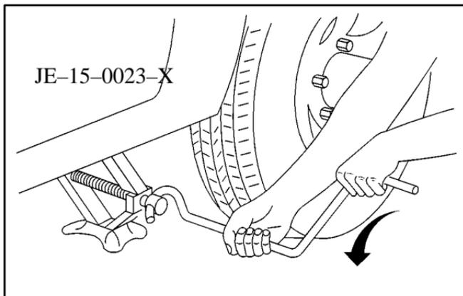
8. Lower the vehicle by turning the jack handle counterclockwise. Lower the jack completely.
