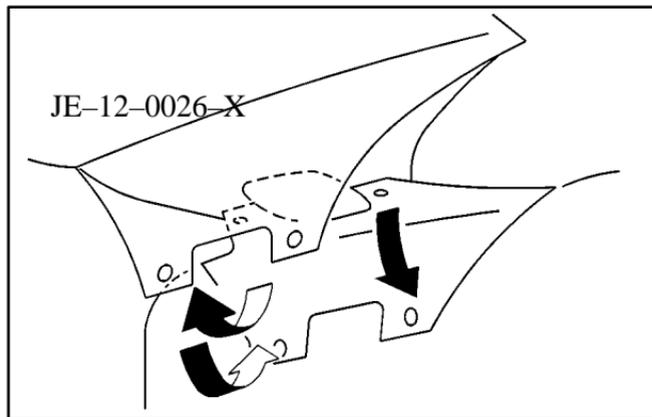
3. Unfasten the snaps that secure the canvas top to the roof piece. The snaps are located on either side of the dome lamp. Reattach the snaps which hold the sunroof canvas in place.
