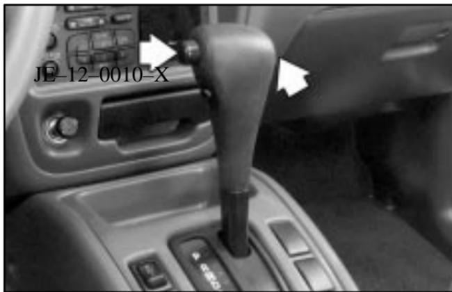
2. Move the shift lever into PARK (P) by holding in the button on the lever and pushing the lever all the way toward the front of your vehicle.
