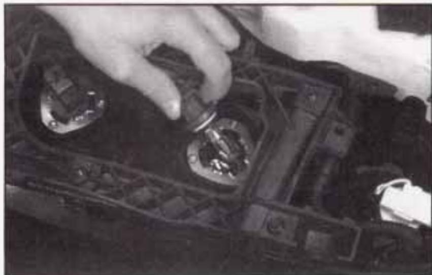
4. Lift the headlamp assembly out of the mounting bracket.
