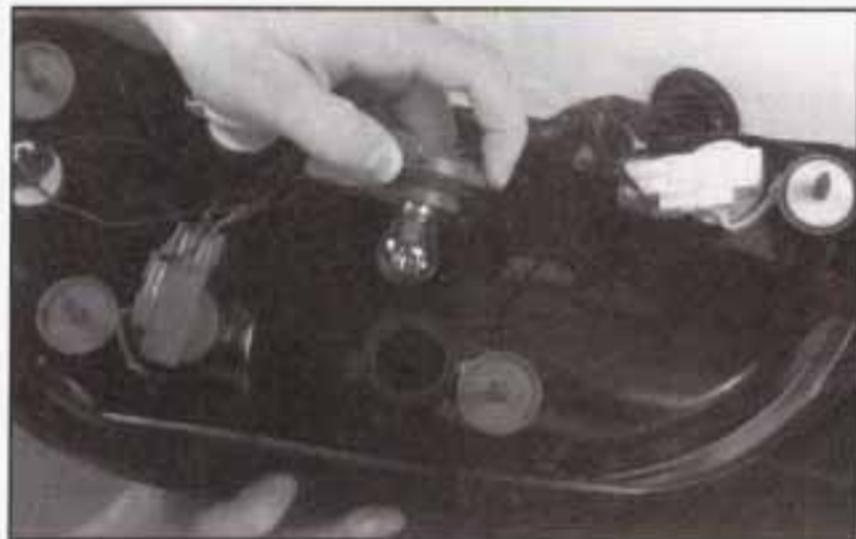
5. To remove a bulb, gently push in and turn the bulb to the left.
