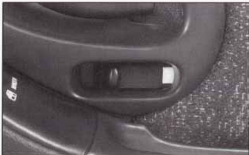
From the inside, you can lock the door by sliding the locking lever rearward.
