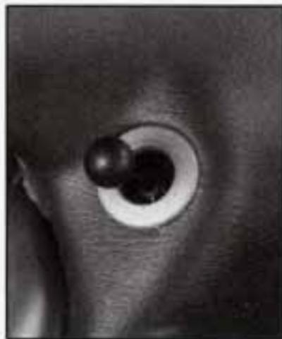
Adjust the driver's side outside mirror with the control lever on the driver's door.
