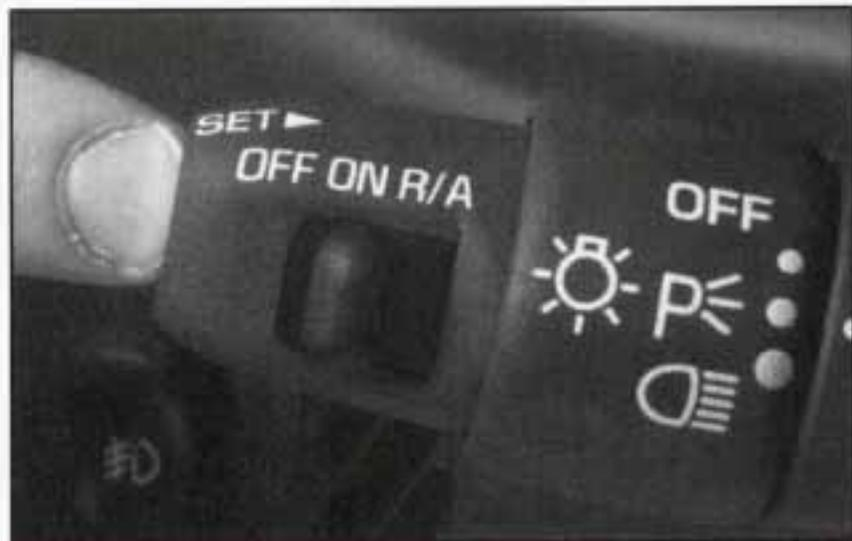
3. Push in the SET button at the end of the lever and release it.
