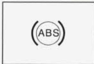
With the anti-lock brake system, this light will come on when you start your engine and it will stay on for three seconds. That's normal.
