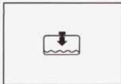
If this light comes on and stays on, the vehicle should be promptly pulled off the road and the coolant level checked. See “Engine Coolant” in the Index.
