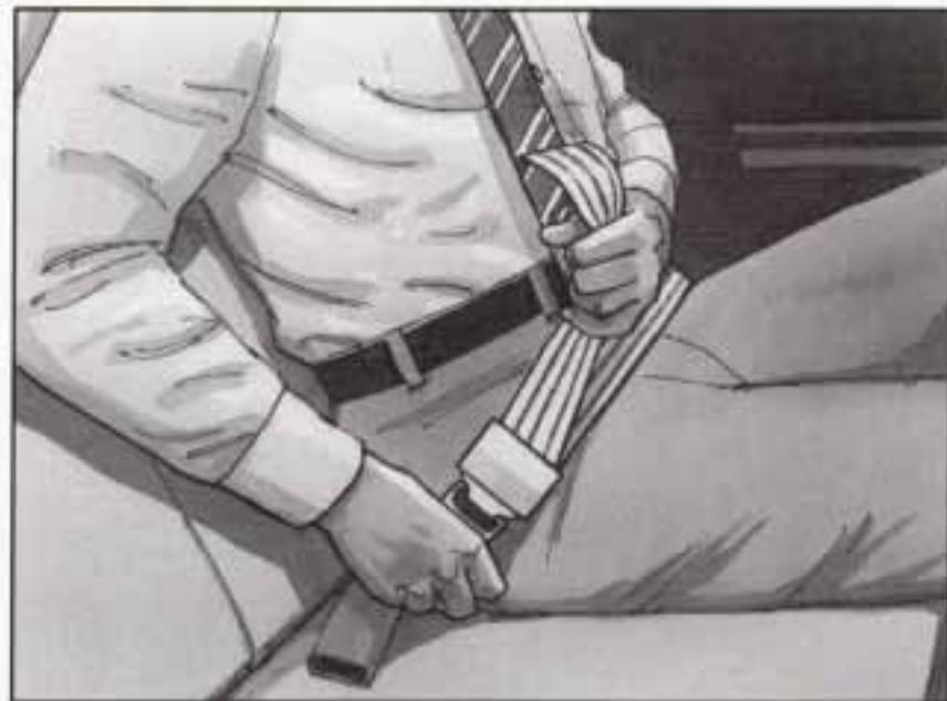
To make the belt shorter, pull its free end as shown until the belt is snug.
