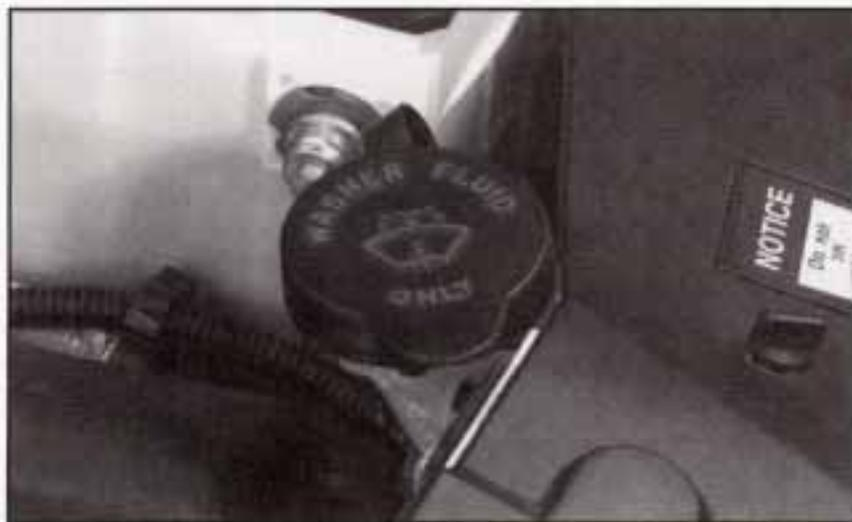
Open the cap labeled WASHER FLUID ONLY. Add washer fluid until the tank is full.
