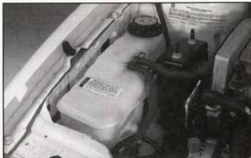
The coolant surge tank is located on the passenger's side of the engine compartment.
