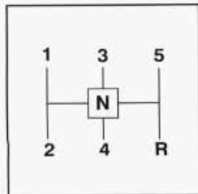
**REVERSE (R):** To back up, press down the clutch pedal and shift into REVERSE (R). Let up on the clutch pedal slowly while pressing the accelerator pedal.
