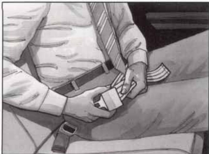
When you sit in the center seating position, you have a lap safety belt, which has no retractor. To make the belt longer, tilt the latch plate and pull it along the belt.
