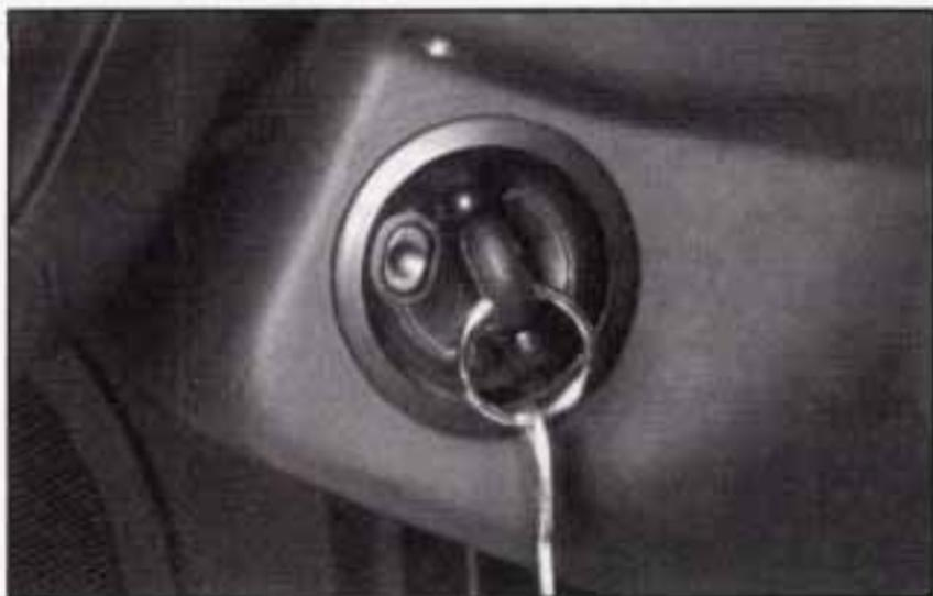
The key cannot be removed from the ignition unless the key release button is used.
