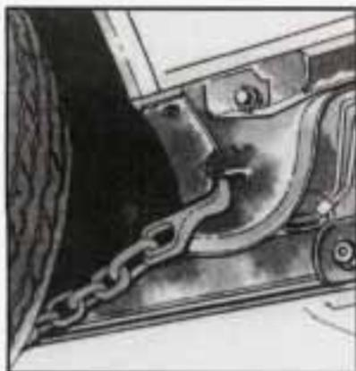
Attach T-hook chains into the slots in the bottom of the floor pan, just behind the front wheels on both sides.
