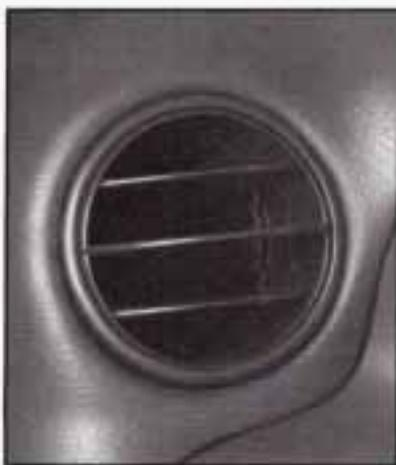
Adjust the direction of airflow by moving the louvered vents.
