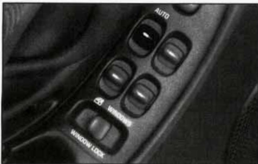
The power window switches are located on the door armrests; the driver's door armrest has controls for all of the windows. These switches will only work when the ignition is on.
