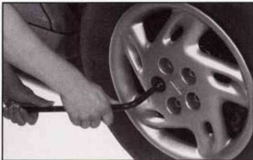
2. Then use the wheel wrench to loosen all the wheel nuts. Don't remove them yet.
