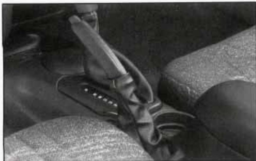
To set the parking brake, hold the regular brake pedal down with your right foot. Pull up on the parking brake handle. If the ignition is on, the brake system warning light will come on.
