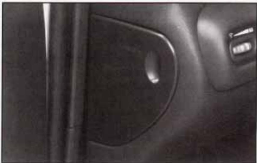
The main fuse panel is located on the left side of the instrument panel. To access the fuses, open the fuse panel door.
