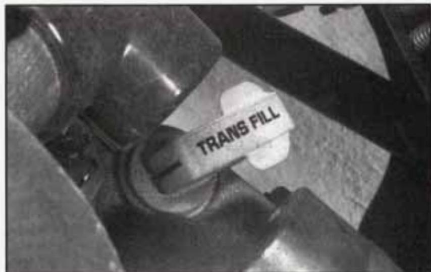
1. The manual transaxle dipstick is white and is located on the driver's side rear of the engine. Flip the handle up and then pull out the dipstick and clean it with a rag or paper towel.
