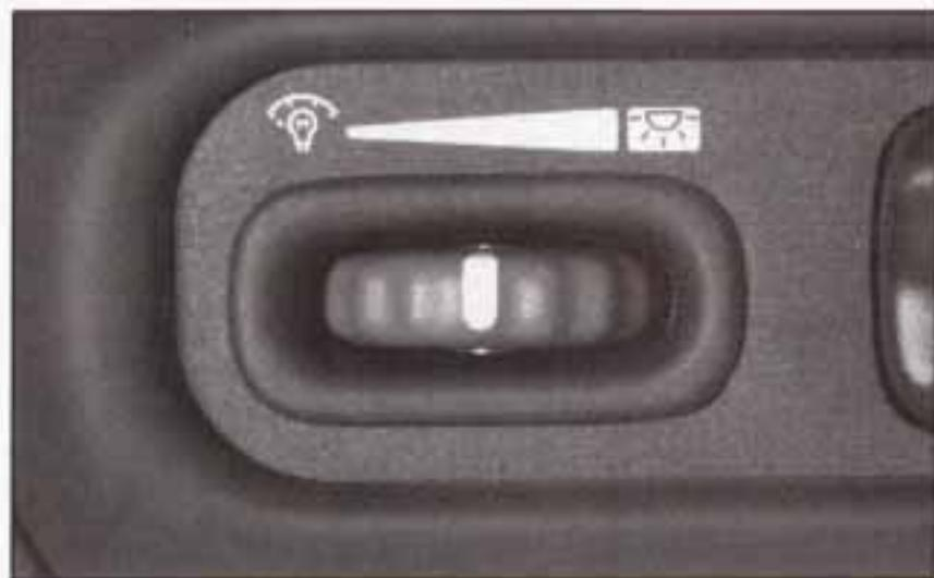
You can brighten or dim your instrument cluster lamps by rotating the instrument panel intensity control switch. Rotate the switch all the way to the right to turn on the interior courtesy lamps. Rotate the switch to the left to turn off the instrument cluster lamps and displays.
