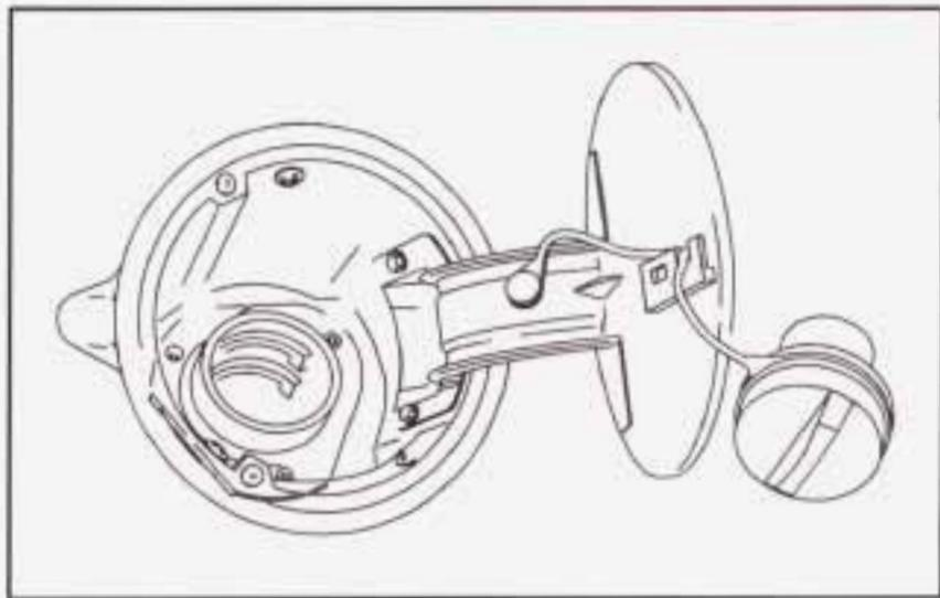
While refueling, hang the tethered cap over the hook inside the fuel door.
