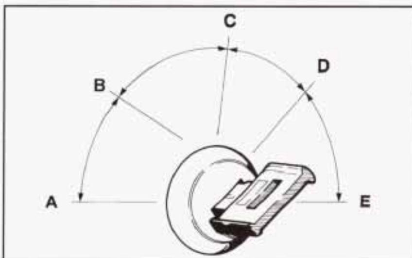
With the key in the ignition switch, you can turn the switch to five positions.
