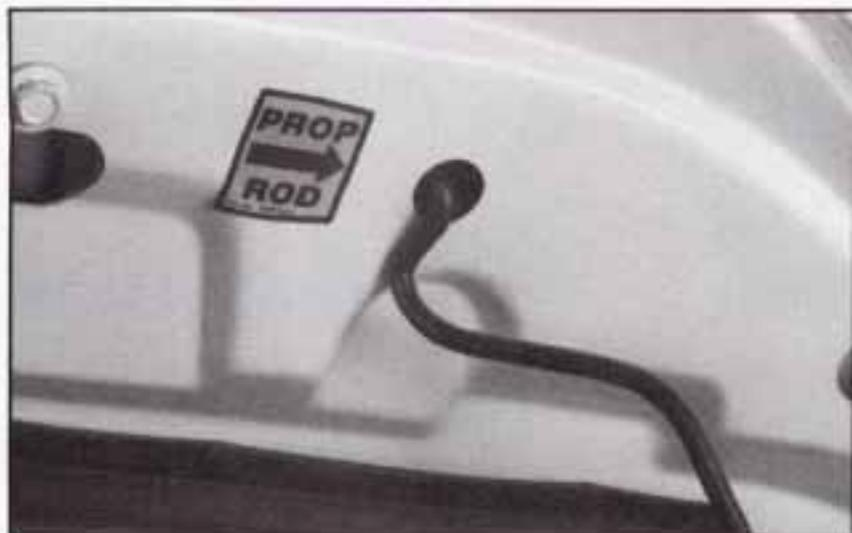
Lift the hood, release the hood prop rod from its retainer and put the hood prop rod into the slot in the hood.
