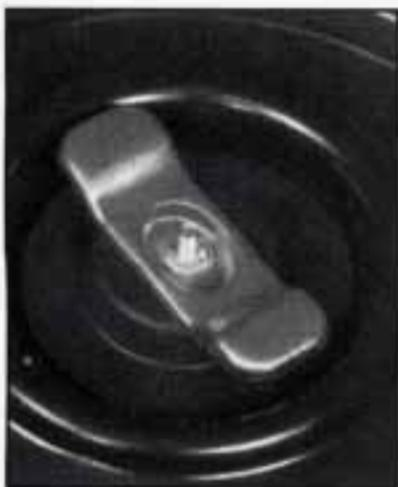
Turn the wing nut to the left and remove it. Then lift off the spacer and remove the spare tire.
