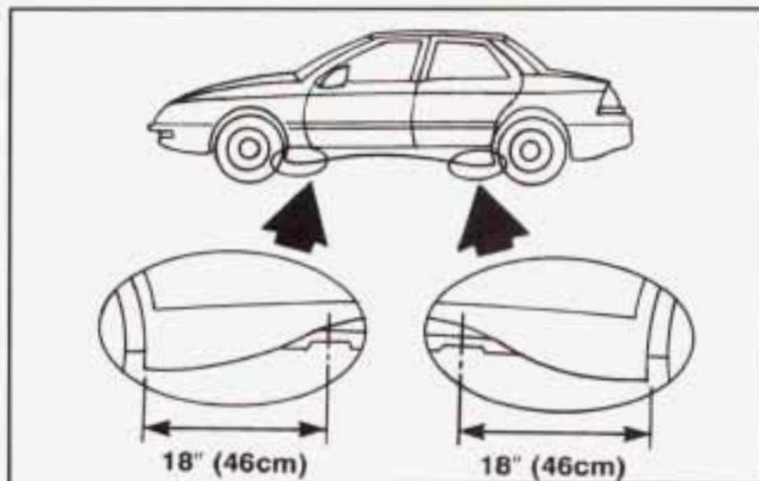
3. Position the jack and raise the jack head until it fits firmly into the notch in the vehicle's frame nearest the flat tire. Put the compact spare tire near you.
