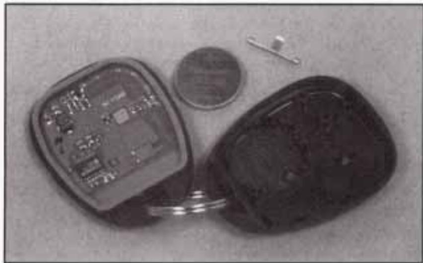
2. Remove the battery and replace it with the new one. Make sure the positive (+) side of the battery faces down. Use one 3-volt, CR2032, or equivalent type battery.
