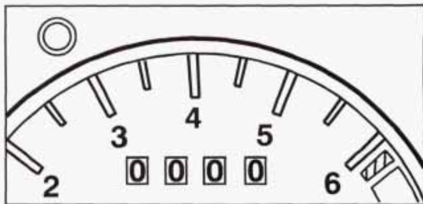
The trip odometer can tell you how far you have driven since you last reset it. To reset the trip odometer to zero, press the knob at the top left side of the instrument panel cluster.
