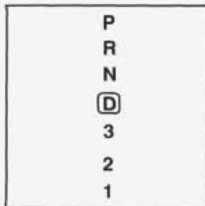
There are seven different positions for the shift lever on the four-speed automatic transaxle.
