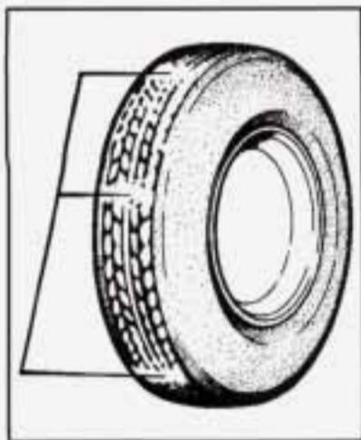
One way to tell when it's time for new tires is to check the treadwear indicators, which will appear when your tires have only 1/16 inch (1.6 mm) or less of tread remaining.
