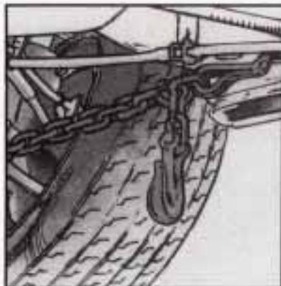
Attach T-hook chains on both sides in the slotted holes in the underbody just ahead of the wheels.
