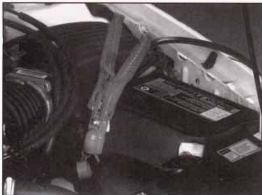
6. Connect the red positive (+) cable to the positive (+) terminal of the vehicle with the dead battery.
