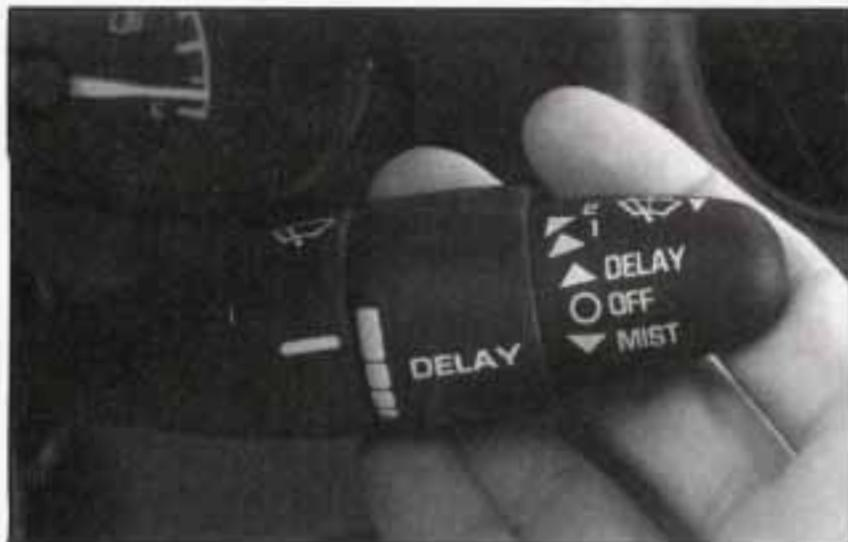
To wash your windshield, pull the stalk with the windshield washer symbol toward you until the washers begin. When the lever is pulled with the wipers in OFF, the wipers will continue to work until you return the lever to OFF. If your vehicle is equipped with the controlled cycle wipers, the wipers will automatically shut off after you release the lever if no speed was selected.
