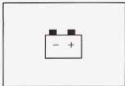
The charging system indicator light will come on briefly when you turn on the ignition, but the engine is not running. The light will go out when the engine is started.
