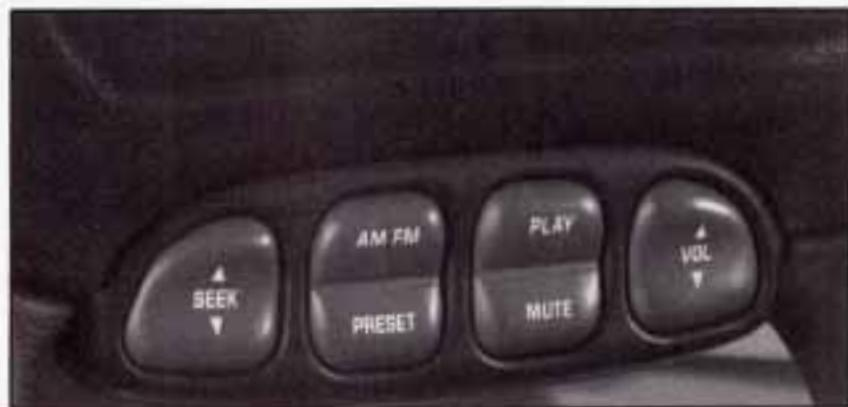
If your vehicle has this feature, you can control certain radio functions using the buttons on your steering wheel.
