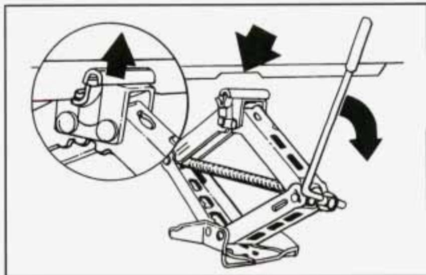
4. Raise the vehicle by rotating the wheel wrench to the right. Raise the vehicle far enough off the ground so there is enough room for the spare tire to fit.
