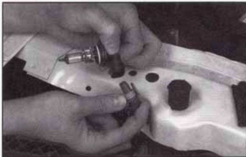
6. Unclip the bulb assembly from the wiring harness.
