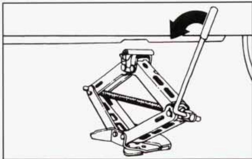
9. Lower the vehicle by rotating the wheel wrench to the left. Lower the jack completely.
