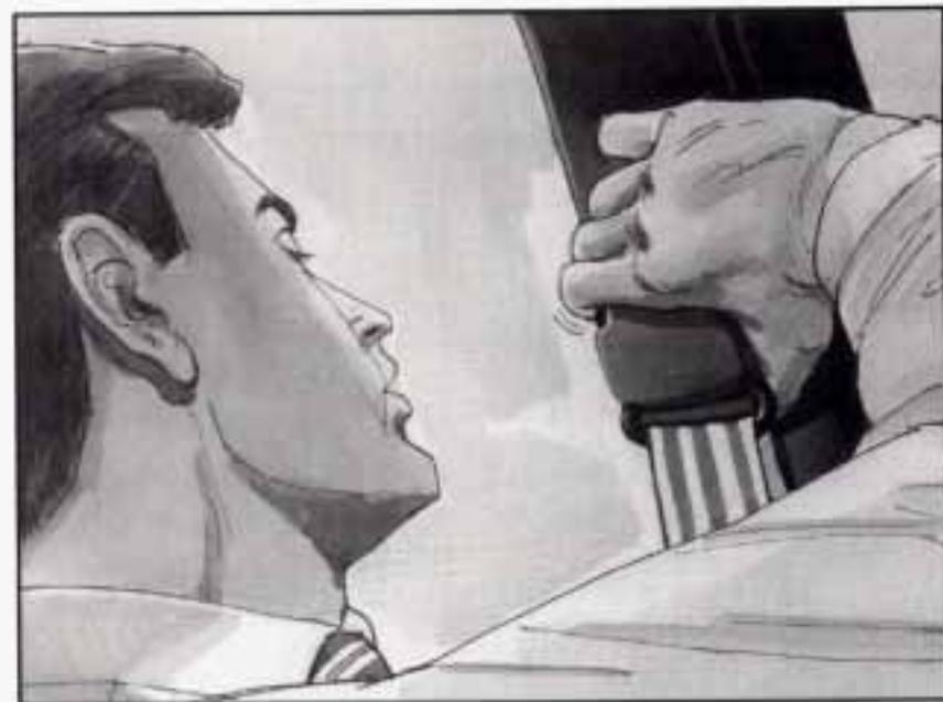
To move it down, squeeze the release button and move the adjuster to the desired position. You can move the adjuster up just by pushing up on the shoulder belt guide. After you move the adjuster to where you want it, try to move it down without squeezing the release button to make sure it has locked into position.
