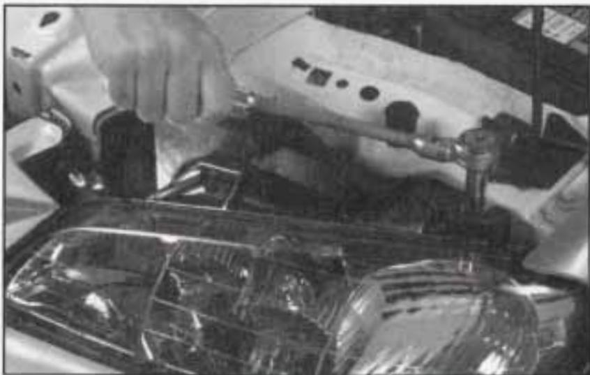
3. Remove the two headlamp assembly attachment bolts.
