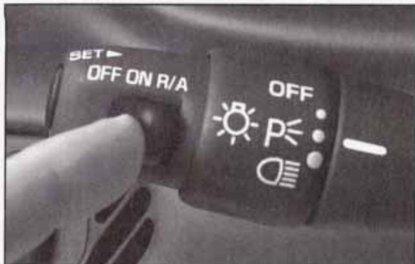
Suppose you set your cruise control at a desired speed and then you apply the brake. This, of course, shuts off the cruise control. But you don't need to reset it. Once you're going about 25 mph (40 km/h) or more, you can move the cruise control switch from ON to R/A (Resume/Accelerate) for about half a second.
