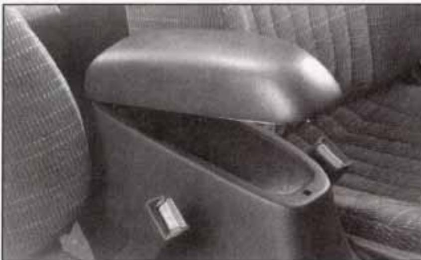
The armrest opens into a storage area for cassette tapes, gloves, etc. To open it, lift up on the front portion of the armrest.
