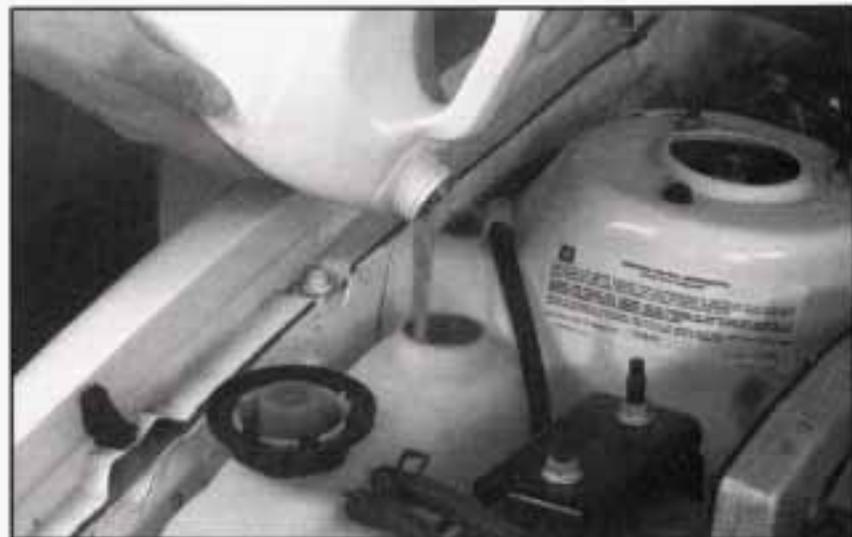
3. Then fill the coolant surge tank with the proper mixture, up to **FULL COLD**, or just above the small cylinder at the base of the opening.
