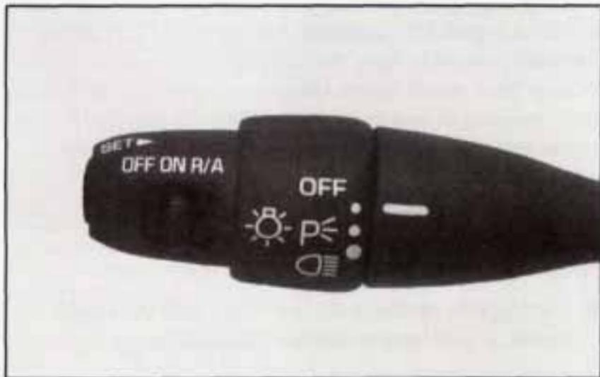
Rotate the turn signal lever middle ring up one position to turn on:
