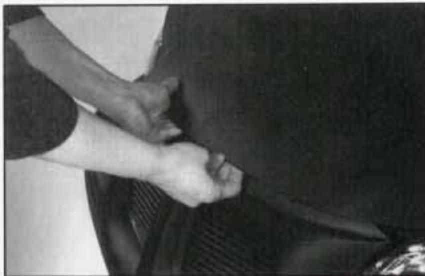
Then go to the front of the vehicle and lift the secondary hood release handle upward.
