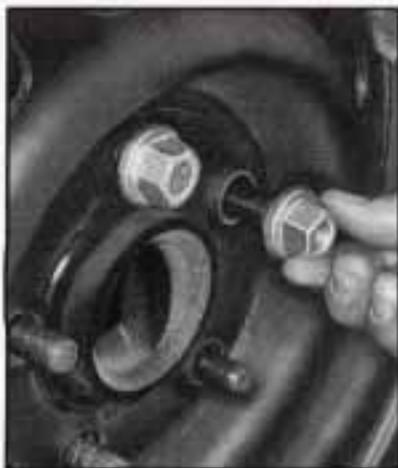
8. Replace the wheel nuts with the rounded end of the nuts toward the wheel. Tighten each nut by hand until the wheel is held against the hub.
