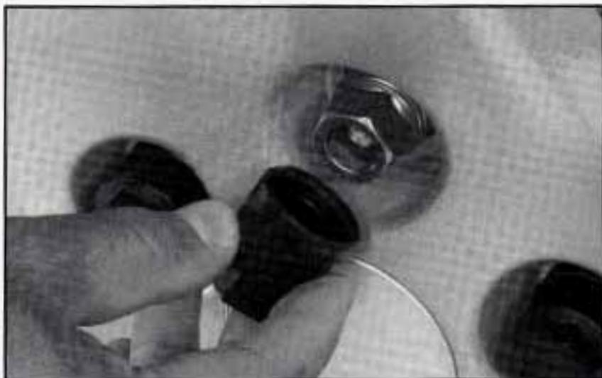
1. Using the wheel wrench, remove plastic nut, loosen all the wheel nuts. Don't remove them yet.
