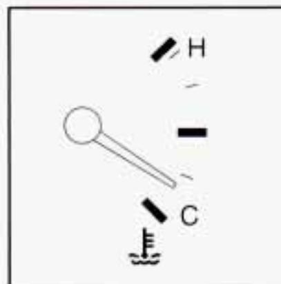
You have a gage that shows the engine coolant temperature. If the gage moves into the red area, your engine is too hot.
