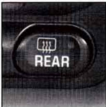
The rear window defogger uses a warming grid to remove fog from the rear window. Press the button to turn the defogger on. It will turn itself off after about 10 minutes.
