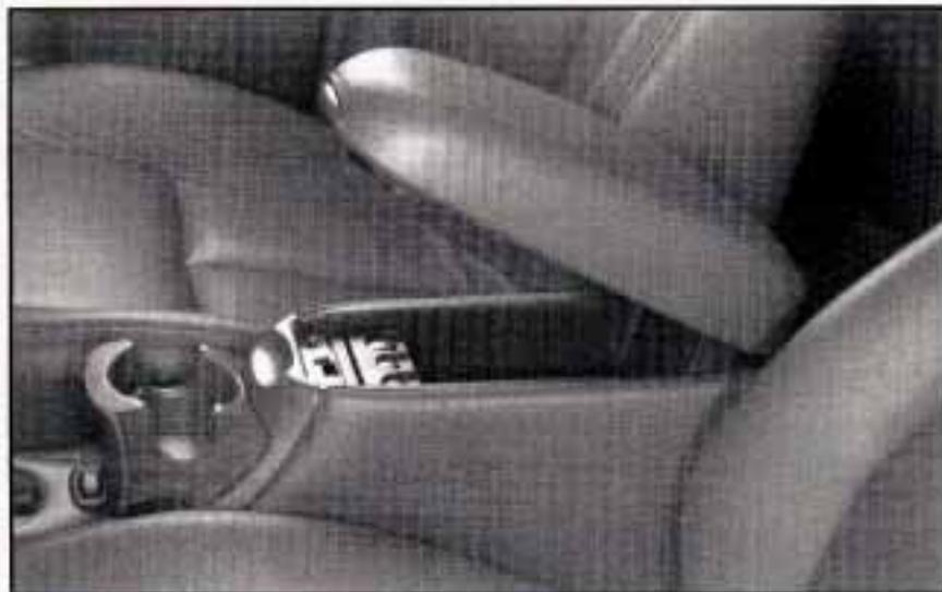
To open the storage area, press back on the front edge and lift the cover. The console has two cupholders, cassette tape and compact disc storage and a coinholder.
