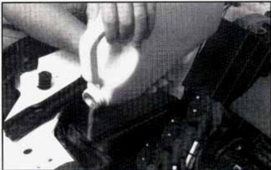
4. Fill the radiator with the proper DEX-COOL<sup>®</sup> coolant mixture, up to the base of the filler neck. (See "Engine Coolant" in the Index for more information about the proper coolant mixture.)
