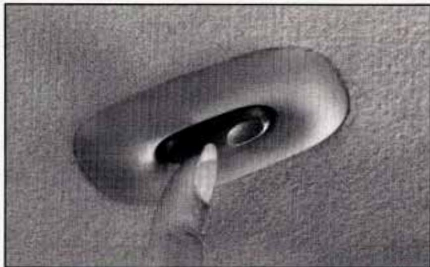
To open the power sunroof, press the rear of the switch once and the power sunroof will fully open. This is the express-open feature. During operation, press the switch again to stop the power sunroof at a desired position.
