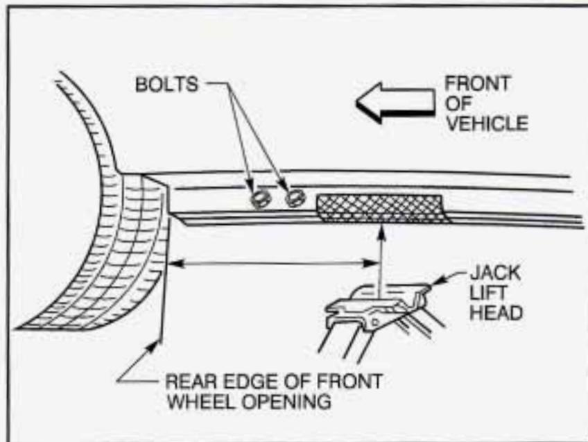
For jacking at the vehicle's front location, put the jack lift head about 8 inches (20 cm) from the rear edge of the front wheel opening or just behind the two bolts as shown.
