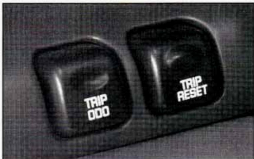
Your trip odometer (trip mode) tells you how far you have driven since you last reset it. To set it to zero, press the TRIP RESET button on the left side of the instrument panel.
