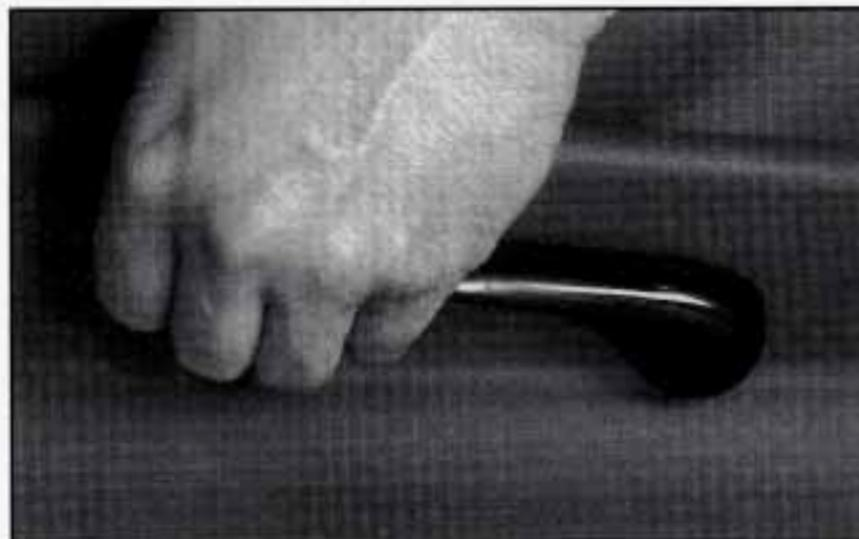
Lift the lever to release the seatback, then move the seatback to where you want it. Release the lever to lock the seatback in place. Pull up on the lever without pushing on the seatback and the seatback will move forward.
