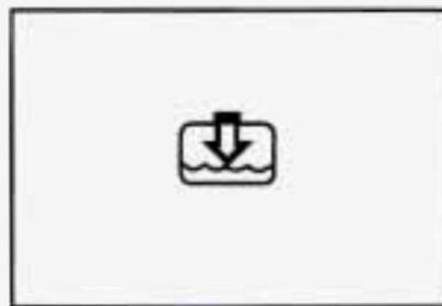
If this low coolant warning light comes on, it means you're low on engine coolant.
