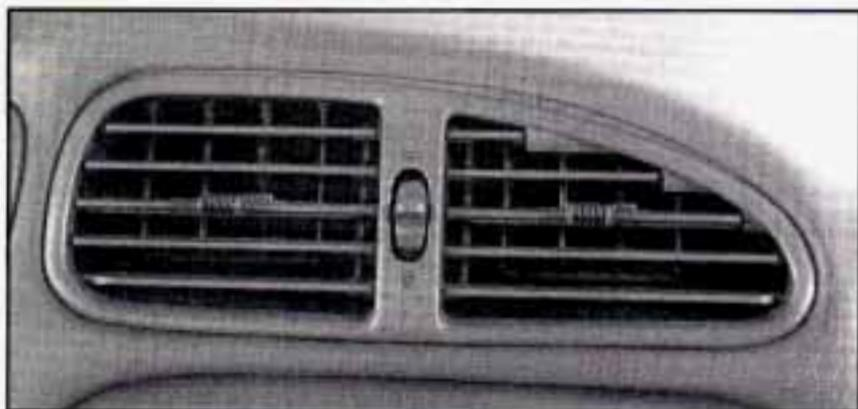
Adjust the direction of airflow by moving the louvered vents. To completely shut off airflow to the outlet move the thumbwheel down. To open the outlet for airflow move the thumbwheel up.
