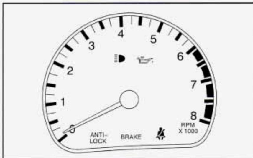
The tachometer displays the engine speed in thousands of revolutions per minute (rpm).
