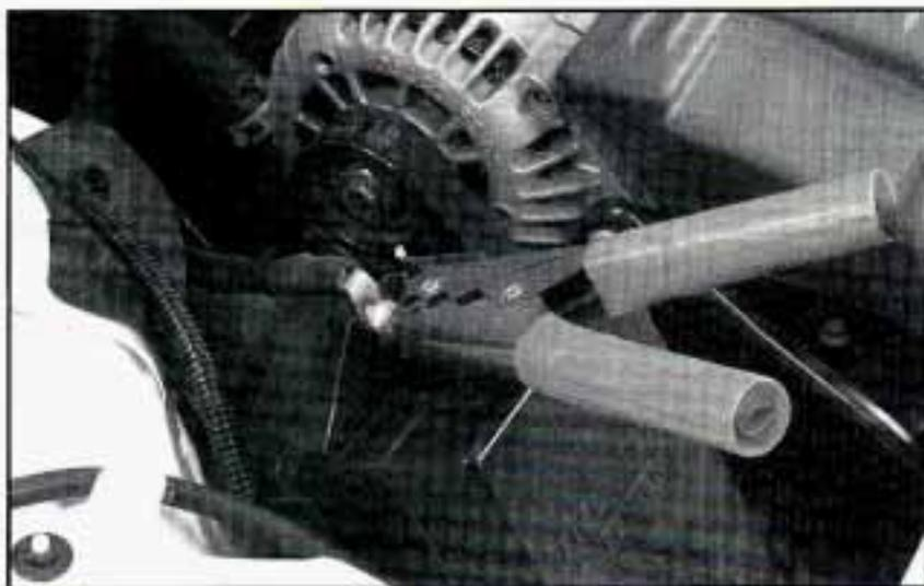
7. Connect the red positive (+) cable to the positive (+) terminal of the vehicle with the dead battery. Use a remote positive (+) terminal.
