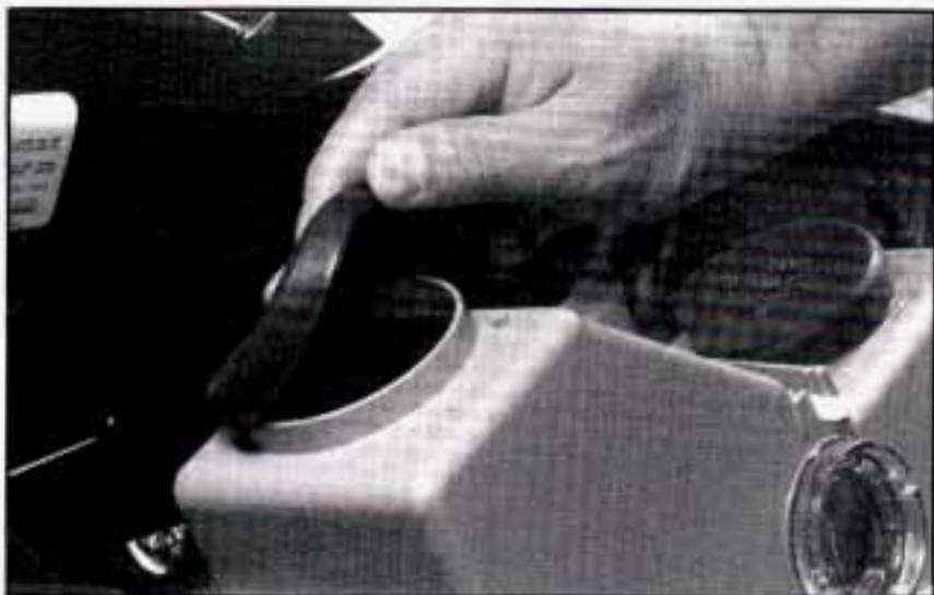
4. Remove the rubber access cover (from behind the bulb you are replacing).
