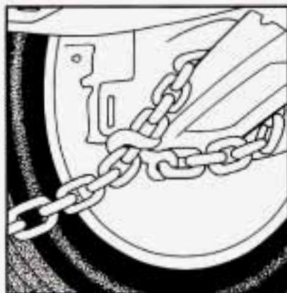
Attach a separate safety chain around the outboard end of each lower arm.
