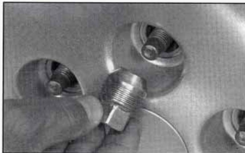
6. Replace the wheel nuts with the rounded end of the nuts toward the wheel. Tighten each nut by hand until the wheel is held against the hub.
