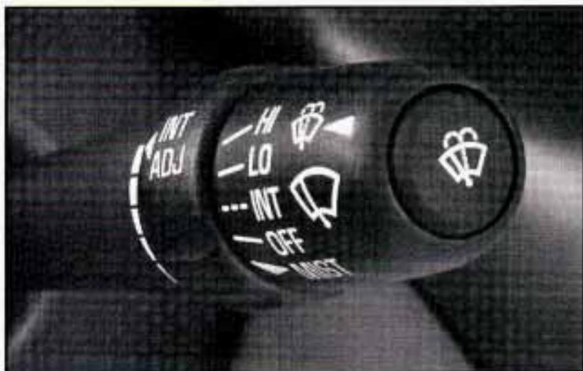
At the end of the right-hand lever on the steering wheel, there is a wiper symbol. To spray washer fluid on the windshield, push the button on the end of the lever. The wipers will run for several sweeps and then either stop or return to your preset speed.
