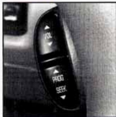
If your vehicle has this feature, you can control certain radio functions using the buttons on your steering wheel.
