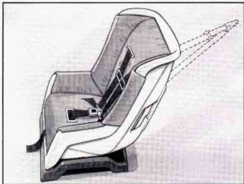
If your child restraint has a top strap, it should be anchored. If you need to have an anchor installed, you can ask your Oldsmobile retailer to put it in for you. If you want to install an anchor yourself, your retailer can tell you how to do it.
