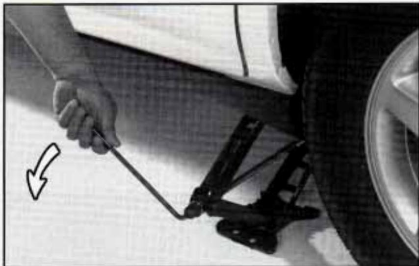
7. Lower the vehicle by turning the jack handle to the left. Lower the jack completely.
