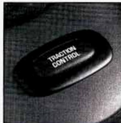
To turn the system on or off, press the button on the console.
