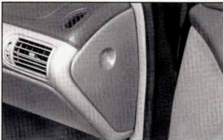
These fuses are located in a fuse block on the passenger's side of the instrument panel. Pull off the right-hand cover to expose the fuses.
