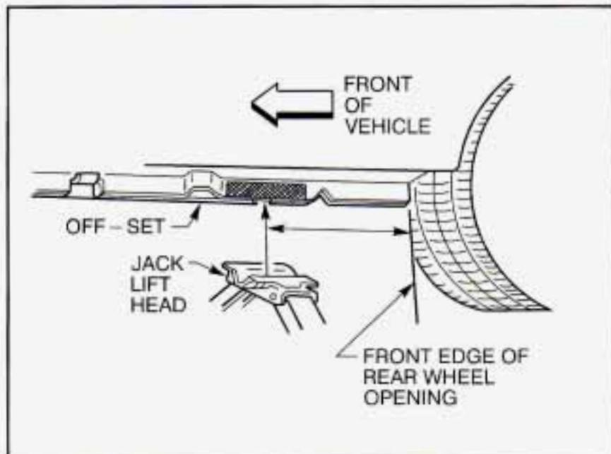
For jacking at the vehicle's rear location, put the jack lift head about 6 inches (15 cm) from the front edge of the rear wheel opening or just behind the off-set as shown.
