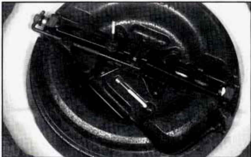
Turn the nut holding the jack to the left and remove it. Then remove the jack and wrench.
