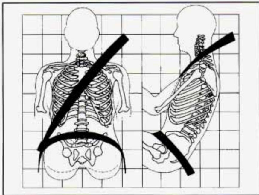
The lap part of the belt should be worn low and snug on the hips, just touching the thighs. In a crash, this applies force to the strong pelvic bones. And you'd be less likely to slide under the lap belt. If you slid under it, the belt
