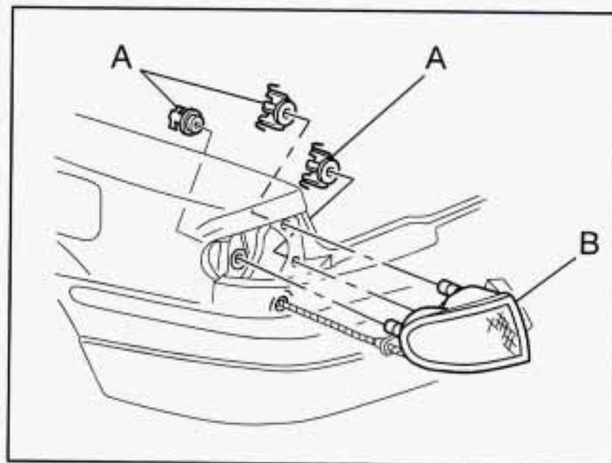
1. Remove the plastic wing nuts (A). (Pliers may be required to remove the wing nuts.)
