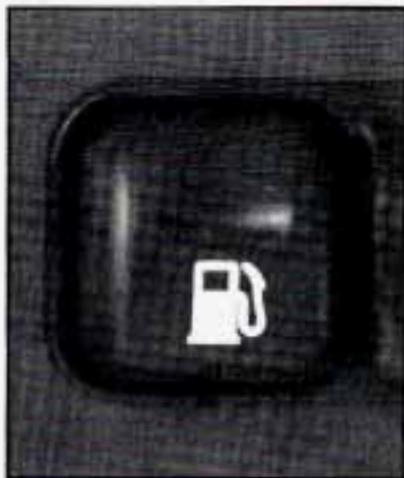
The switch for the fuel door is on the instrument panel, to the left of the steering column.
