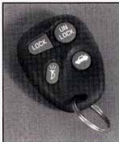
Press UNLOCK once to unlock the driver's door and to turn the interior lamps on (see "Illumination on Remote Activation" in the Index for more details).
