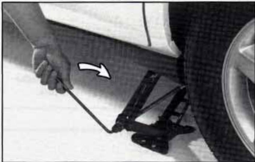
3. Raise the vehicle by turning the jack handle to the right. Raise the vehicle far enough off the ground for the spare tire to fit under the vehicle.
