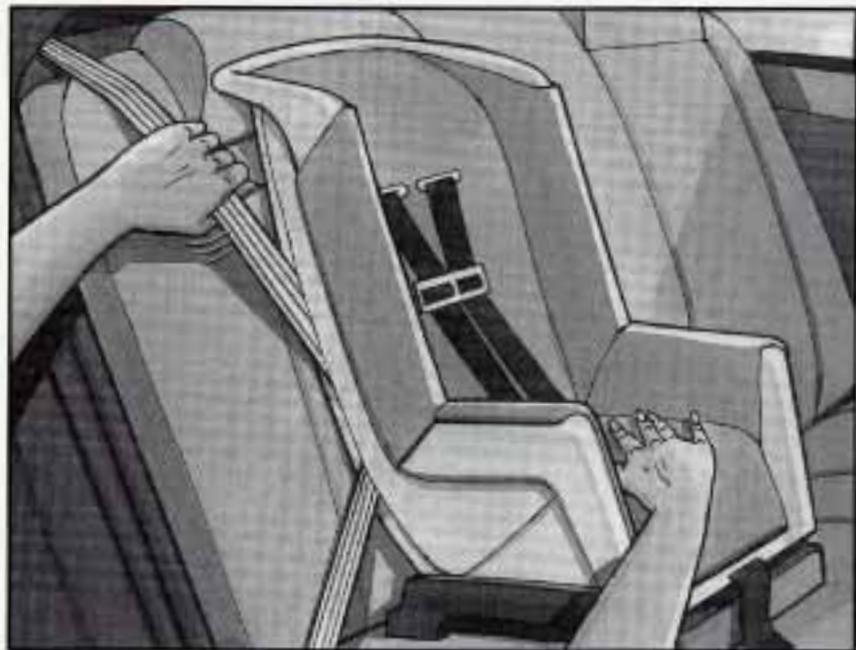
5. To tighten the belt, feed the shoulder belt back into the retractor while you push down on the child restraint. If you're using a forward-facing child restraint, you may find it helpful to use your knee to push down on the child restraint as you tighten the belt.
