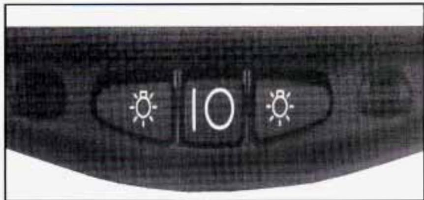
The mirror includes two map lamps, automatic dimming function and an eight-point compass display in the upper corner of the mirror face. When the compass display is turned on, the compass automatically calibrates as the vehicle is driven.
