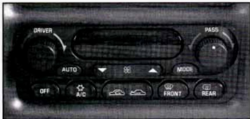
With this system, you set a temperature. You can then either let the system adjust airflow and force to maintain the temperature, or you can manually adjust the flow and force. The system works best if you keep your windows closed while using it.
