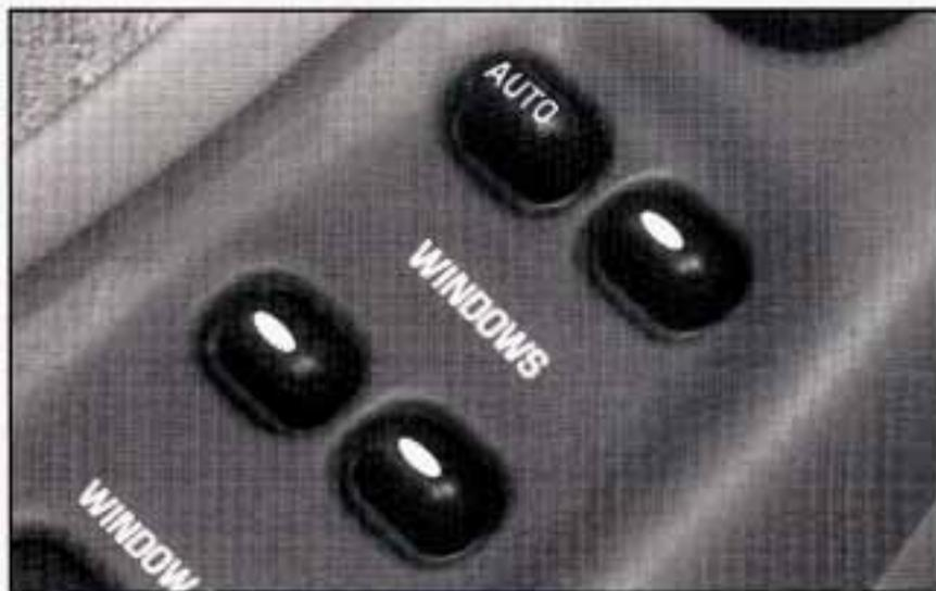
Switches on the driver's door armrest control each of the windows when the ignition is on. In addition, each passenger door has a switch for its own window.
