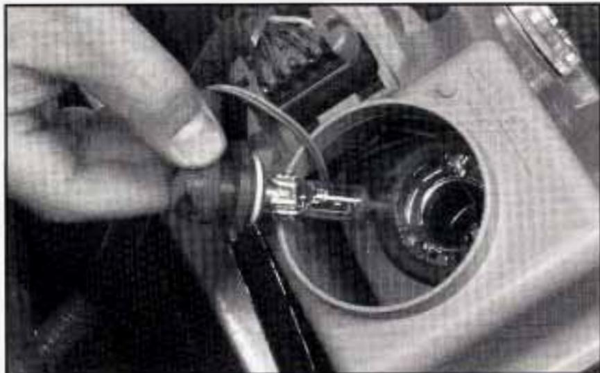
6. Replace the bulb, making sure not to touch the new bulb with bare hands.
