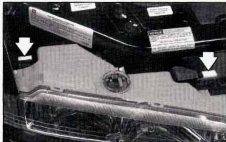
2. Pull straight up on the two headlamp retainers to release the assembly locator tabs. At the same time hold the headlamp assembly in position by applying a little pressure against the headlamp lens. This prevents the lamp from falling out.
