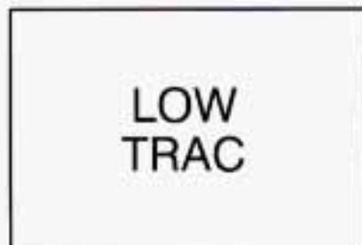
When your anti-lock system is adjusting brake pressure to help avoid a braking skid, this light will come on.
