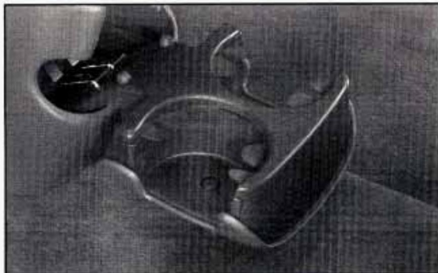
The cupholders are located in the rear of the front console. Pull down to use the cupholders.
