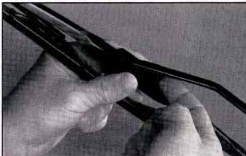
2. While holding the wiper arm away from the glass, push the release clip from under the blade connecting point and pull the blade assembly down toward the glass to remove it from the wiper arm.
