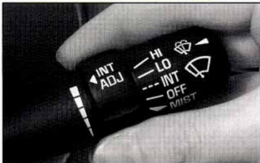
You can control the windshield wipers by turning the band with the wiper symbol on it. This lever is located on the right-hand side of the steering wheel.
