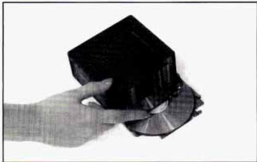
You must first load the magazine with discs before you can play a compact disc. Each of the 12 trays holds one disc. Press the button on the back of the magazine and pull gently on one of the trays. Load the trays from
