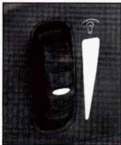
You can brighten or dim the instrument panel lights by moving the interior lamps dial. Turn the dial up to increase the brightness of the instrument panel lights. Turn the dial down to decrease the brightness.
