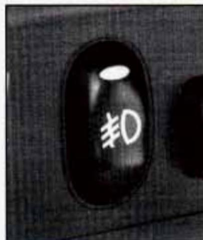
To turn the fog lamps on, press the fog lamp switch. A light will glow on the switch to let you know that they are on. (Your parking lamps must be on, or your fog lamps won't come on.) Press the switch again to turn the fog lamps off.
