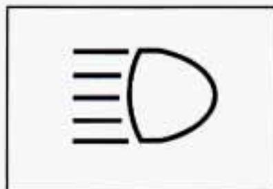
To change your headlamps from low beam to high beam, push the lever forward. To change back to low beam, pull the lever toward you.
