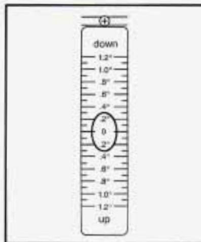
It is recommended that the upper limit not exceed plus 0.4 degrees from the center of the bubble. Other drivers may flash their high beams at you if your adjustment is much above plus 0.4 degrees.
