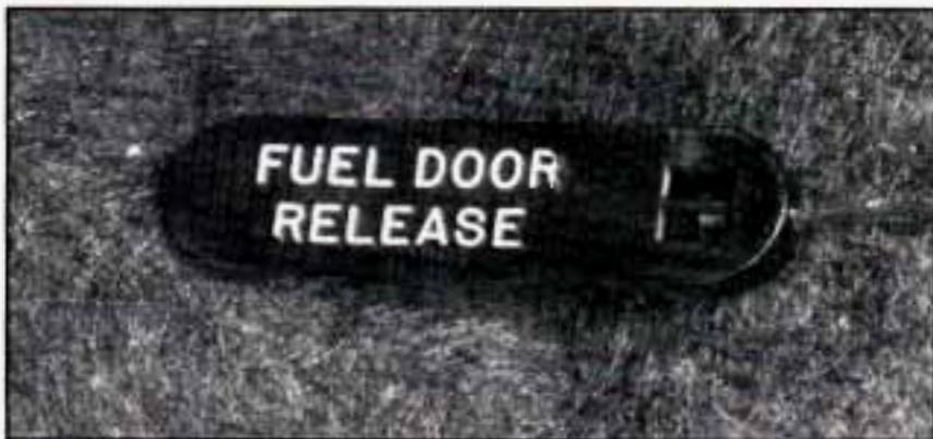
If your fuel filler door release won't operate, there is a manual release tab. The tab is located against the trim on the driver's side of the vehicle, in the trunk.
