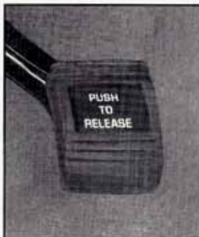
To set parking brake, hold the regular brake pedal down with your right foot. Push down the parking brake pedal with your left foot.
