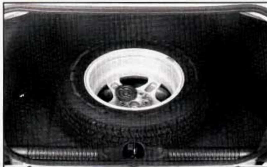
When storing a full-size tire you must use the extension to help avoid wheel surface damage. Use extension and protector/guide located in foam holder.
