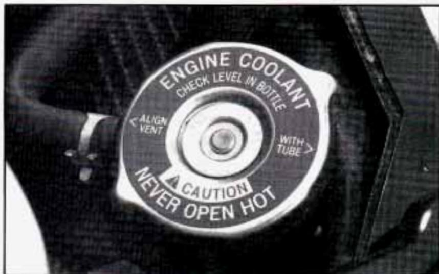
10. Then replace the pressure cap. At any time during this procedure if coolant begins to flow out of the filler neck, reinstall the pressure cap. Be sure the arrows on the pressure cap line up like this.
