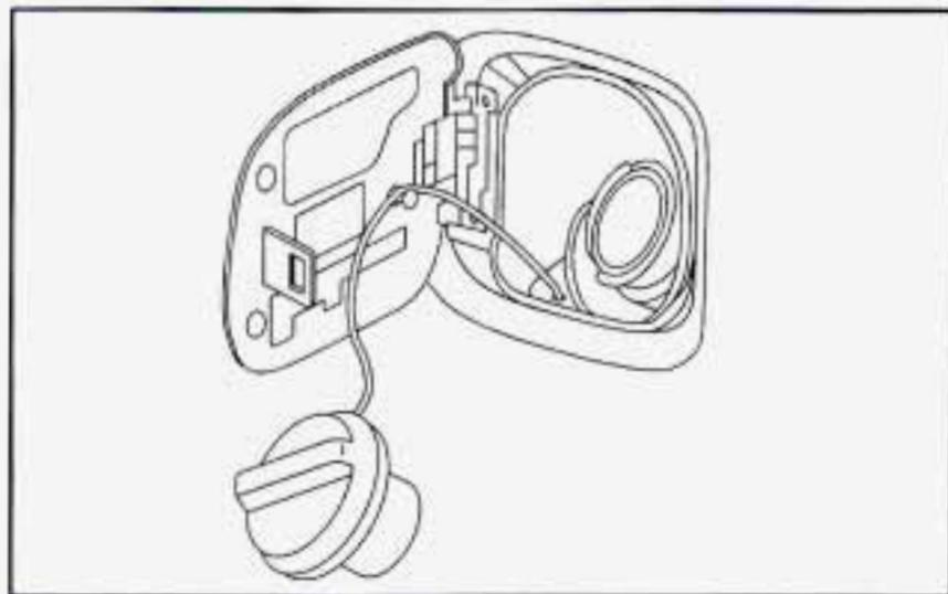
The cap is behind a hinged door on the left side of your vehicle. While refueling, hang the cap by the tether from the pin on the filler door.
