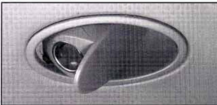
The power outlets are located on the lower left passenger side and behind the flip-out door of the lighter.
