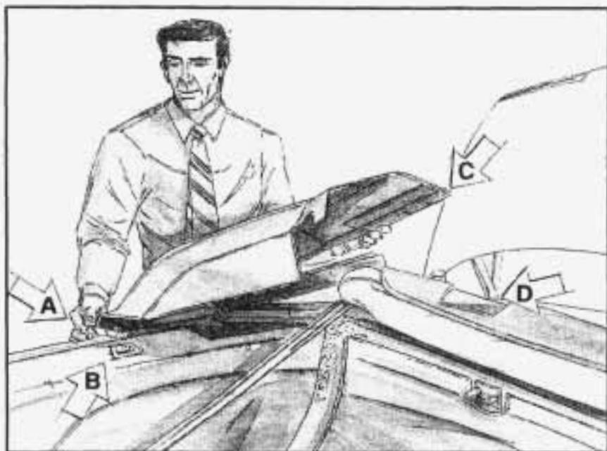
8. Install the boot side cover by inserting the tab (A) on the underside of the cover into the slot (B) at the top of the quarter trim panel. Place the rear flap of the boot side cover in the trunk lid opening, aligning the eyelet (C) over the boot snap ball stud (D).
