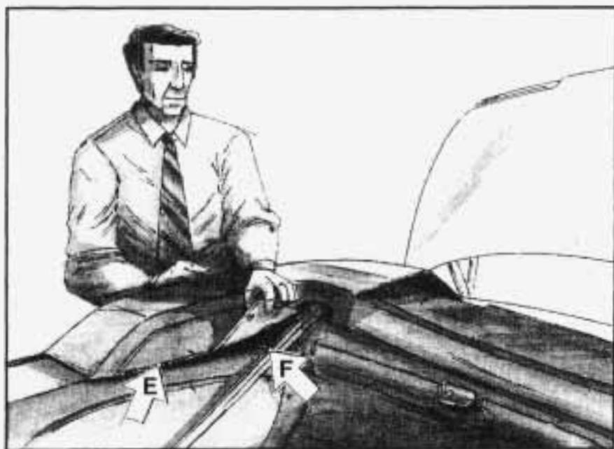
9. Attach the two snaps on the inside flap to the top of the quarter trim panel. Attach the front snap (E) first and then the rear snap (F). The rear snap is adjustable for ease of installation.
