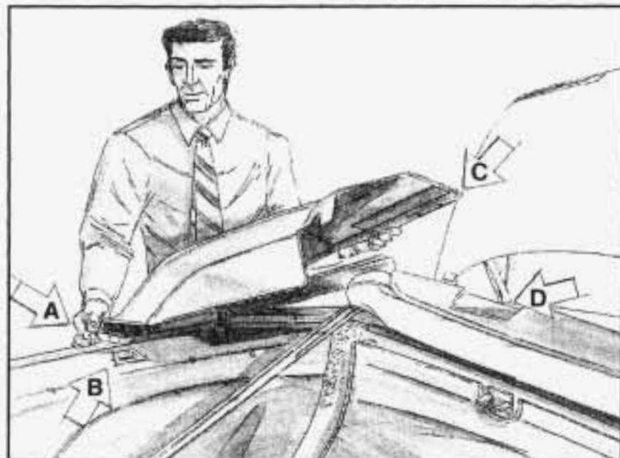
6. Lift side cover eyelet (C) at rear of side boot cover from snap ball stud (D). Raise the back of the boot side cover to unhook the tab (A) from the slot (B) in the quarter trim panel. Do the same on the other side.
