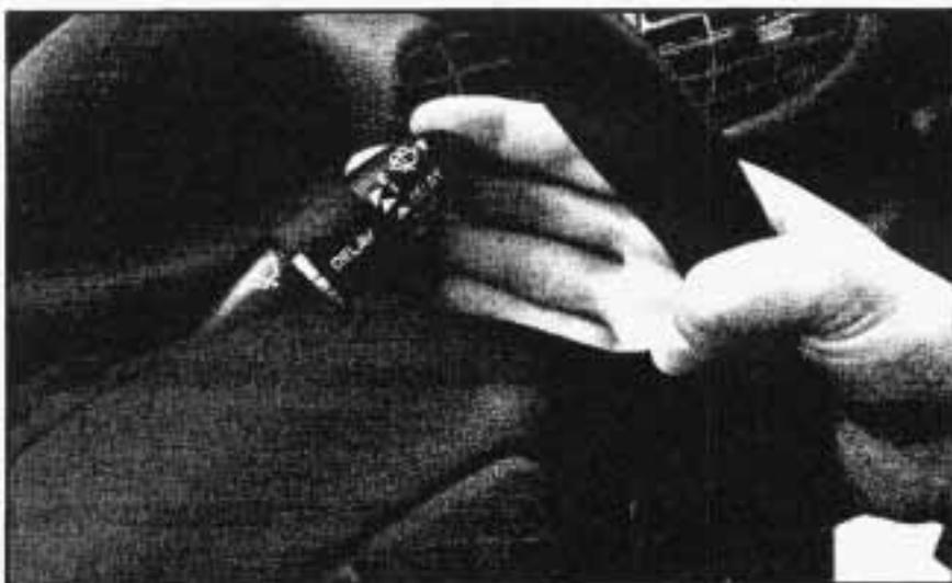
To wash your windshield, pull the stalk with the wiper symbol on it toward you one time. The wipers will clear the window and then either stop or return to your preset speed. If you had no speed selected, the wipers will stop.
