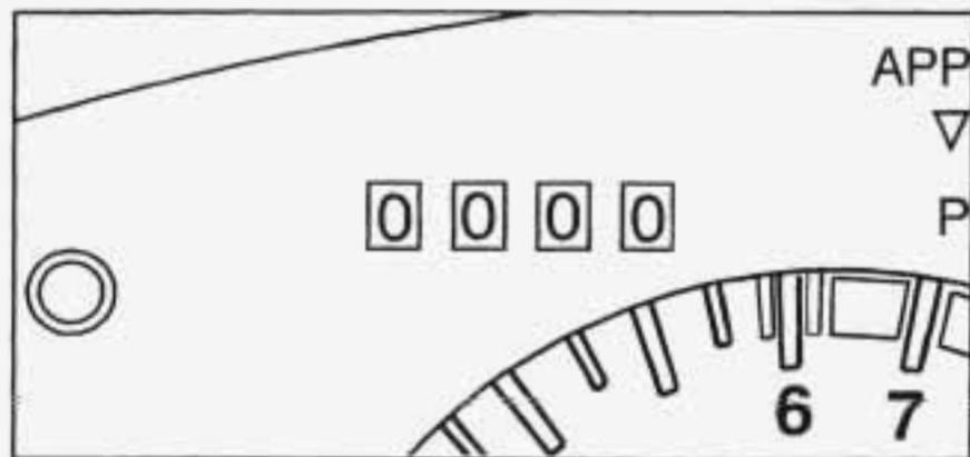
The trip odometer can tell you how far your vehicle has been driven since you last set the trip odometer to zero.
