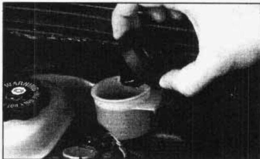
Refer to the Maintenance Schedule to determine how often you should check the fluid level in your clutch master cylinder reservoir and for the proper fluid. See "Owner Checks and Services" and "Recommended Fluids and Lubricants" in the Index.
