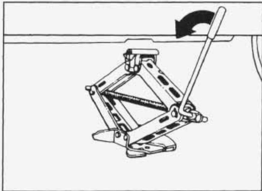
8. Lower the vehicle by rotating the wheel wrench counterclockwise. Lower the jack completely.
