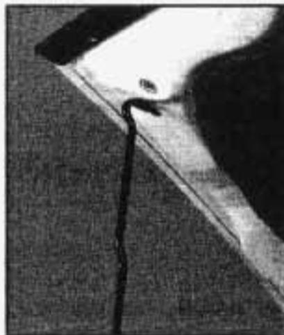
Lift the hood, release the hood prop from its retainer and put the hood prop into the slot in the hood.
