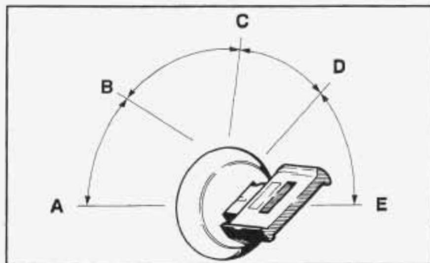
With the ignition key in the ignition switch, you can turn the switch to five position.
