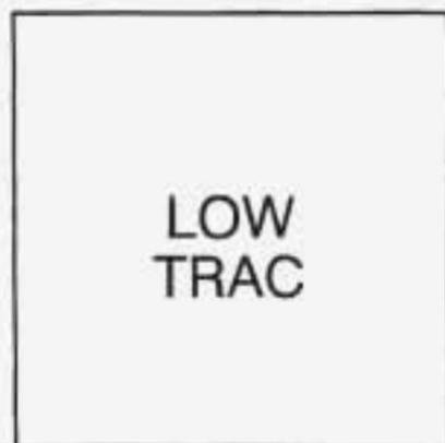
When your Enhanced Traction System is limiting wheel spin, this light will come on. Slippery road conditions may exist if the Enhanced Traction System active light comes on, so adjust your driving accordingly.
