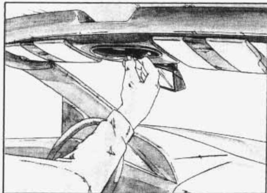
13. Turn the latch handle up to lock the top.
