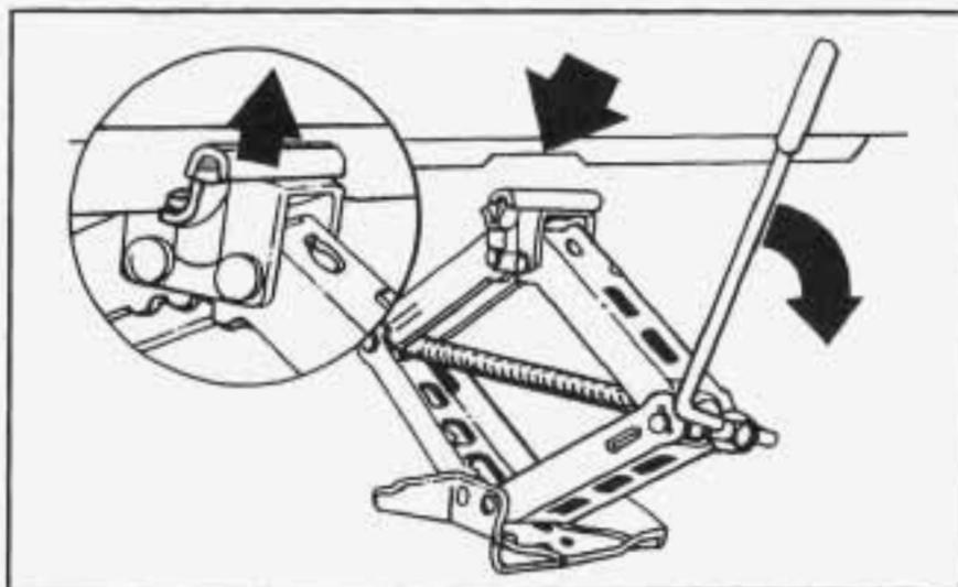
3. Raise the vehicle by rotating the wheel wrench clockwise. Raise the vehicle far enough off the ground so there is enough room for the spare tire to fit.
