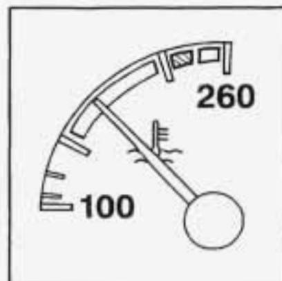
With the ignition in the RUN position, this gage shows the engine coolant temperature.
