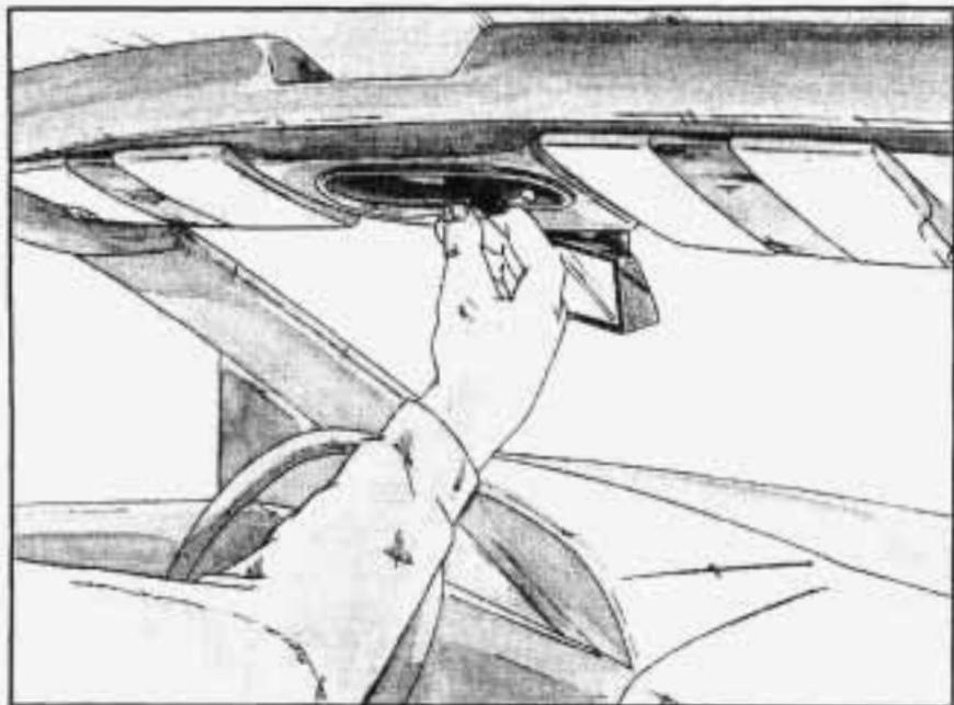
5. Turn the latch handle up to the locked position.
