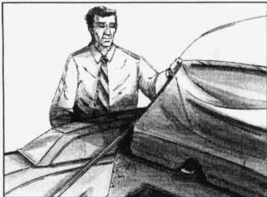
10. Pull the boot center cover from behind the rear seatback and place it over the inner sides of the boot side covers and the lowered top.
