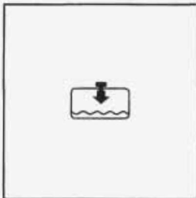
If this light comes on and stays on, your system is low on coolant and the engine may overheat.
