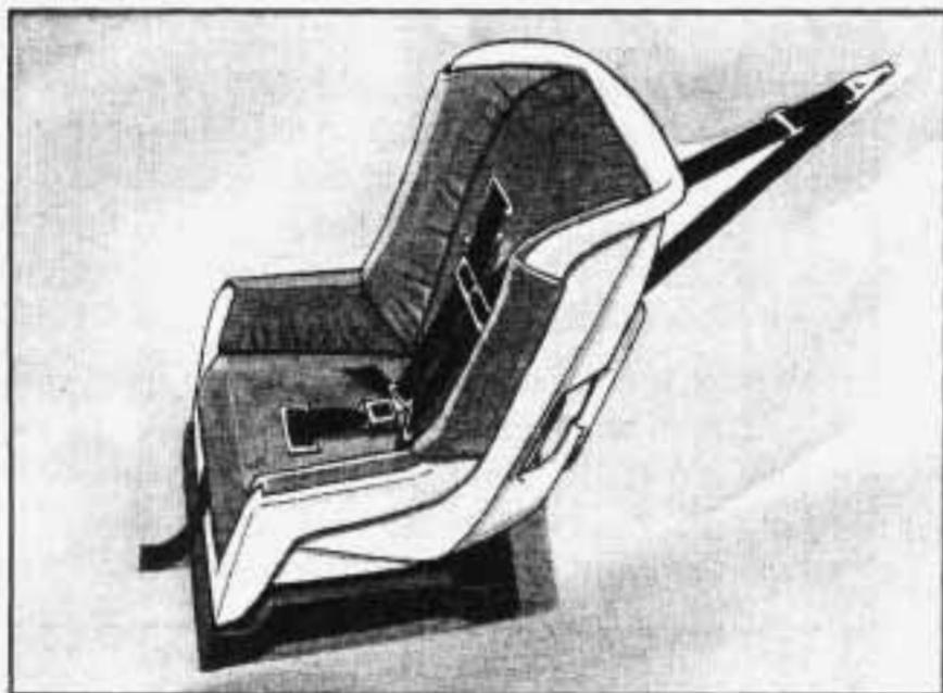
If your child restraint has a top strap, it should be anchored. If you have a convertible, don't use a restraint like that in your vehicle because the top strap anchor cannot be installed properly. You shouldn't use this type of restraint without anchoring the top strap.
