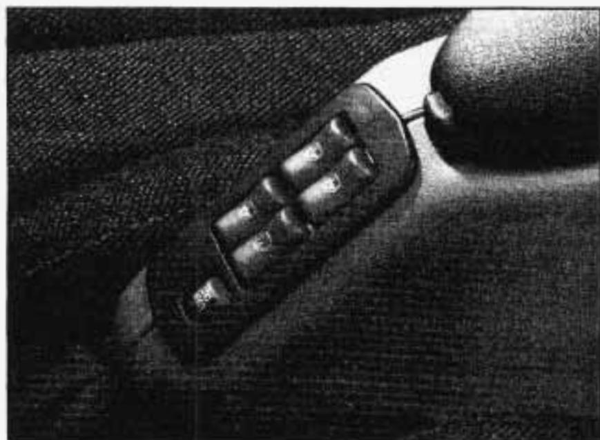
With power windows, switches on the center console control each of the windows only when the ignition is on. In addition, in four-door models, each rear passenger door has a control switch for its own window.
