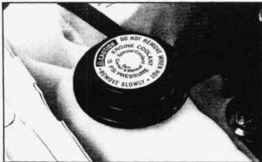
1. You can remove the coolant surge tank pressure cap when the cooling system, including the coolant surge tank pressure cap and upper radiator hose, is no longer hot. Turn the pressure cap slowly about one-quarter turn to the left and then stop.
