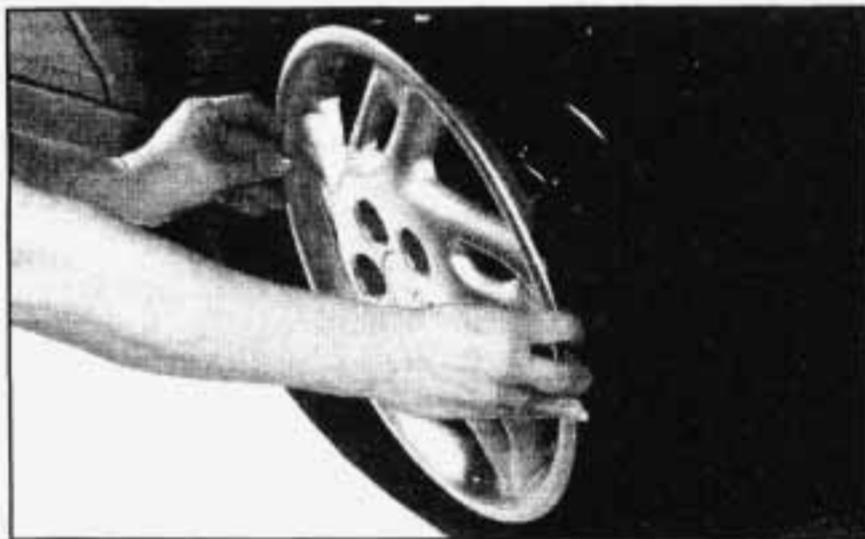
5. If you have a wheel cover, use your fingers to carefully pry the wheel cover from the wheel. Then remove the flat tire.
