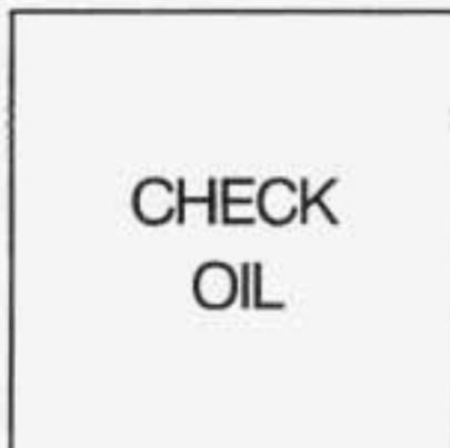
This light should come on briefly while you are starting your engine. If the light doesn't come on, have it repaired. If the light comes on while starting and stays on, your engine oil level should be checked.
