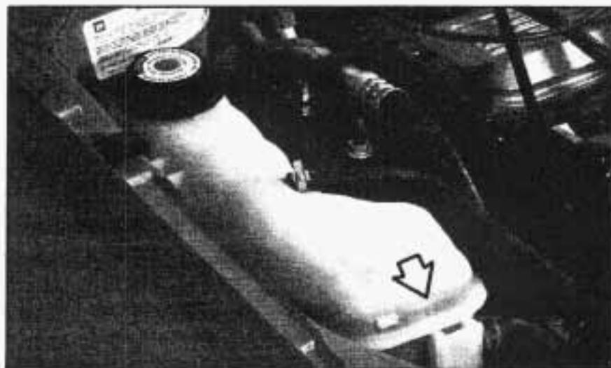
The surge tank is located on the passenger side of the engine compartment.
