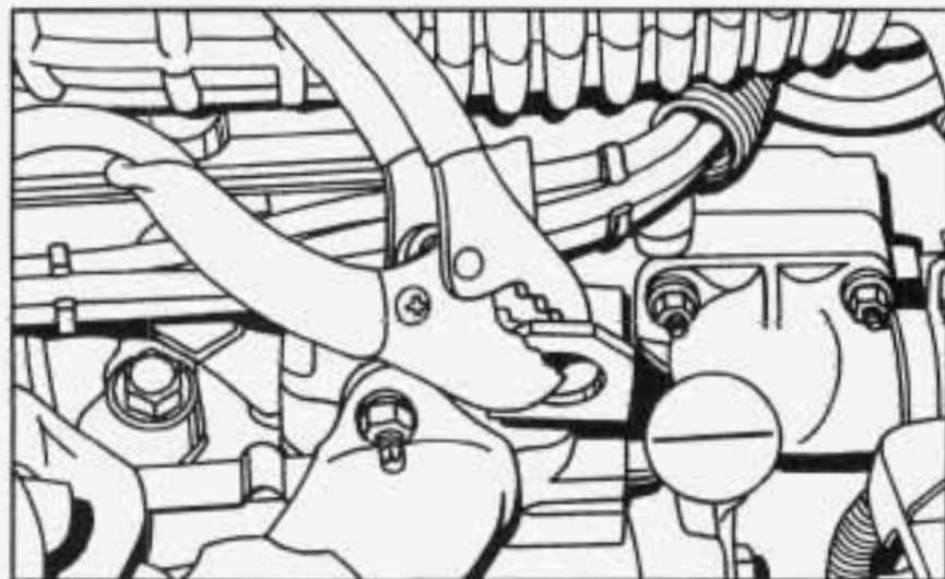
10. Attach the cable at least 18 inches (45 cm) away from the dead battery, but not near engine parts that move. The electrical connection is just as good there, but the chance of sparks getting back to the battery is much less.
