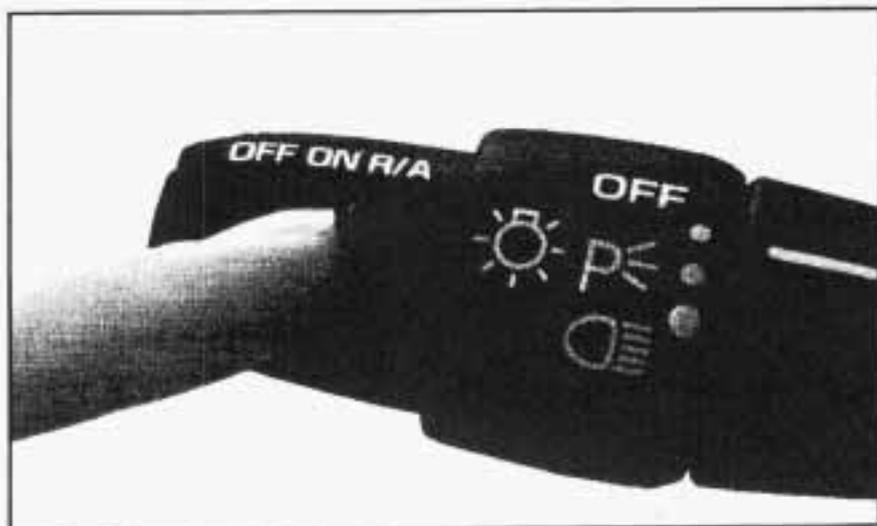
Suppose you set your cruise control at a desired speed and then you apply the brake or clutch pedal. This, of course, shuts off the cruise control. But you don't need to reset it. Once you're going about 25 mph (40 km/h) or more, you can move the cruise control switch from ON to R/A for about half a second.
