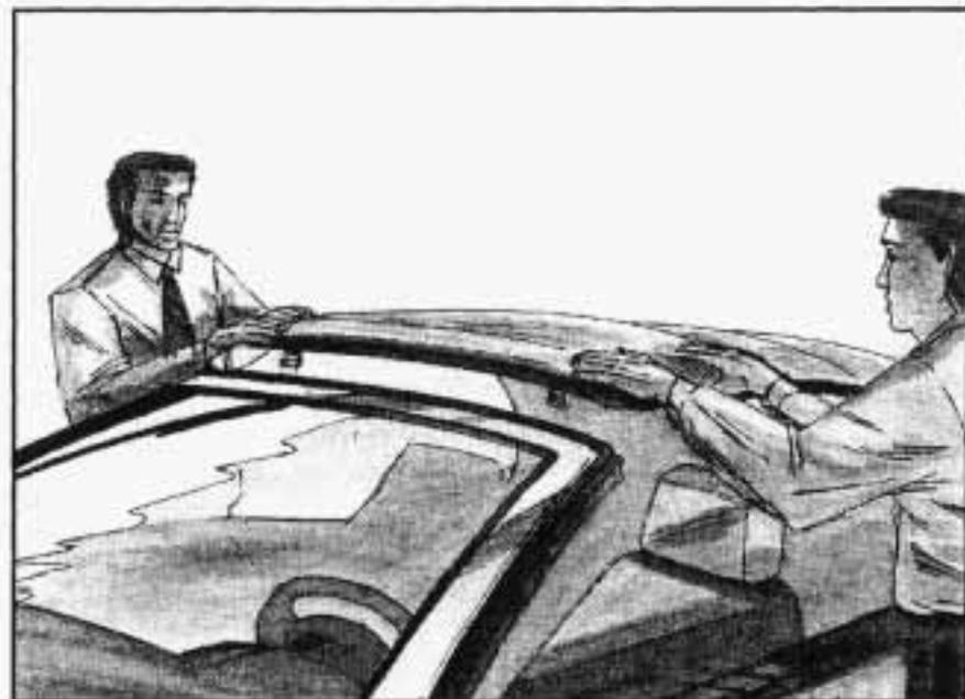
9. Pull down on the top and turn the latch handle up to lock the convertible top.
