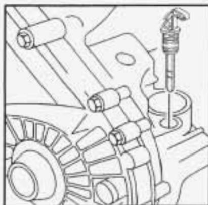
1. The manual transaxle dipstick is located below the brake master cylinder, near the rear of the transaxle case. Flip the handle up and then pull out the dipstick and clean it with a rag or paper towel.
