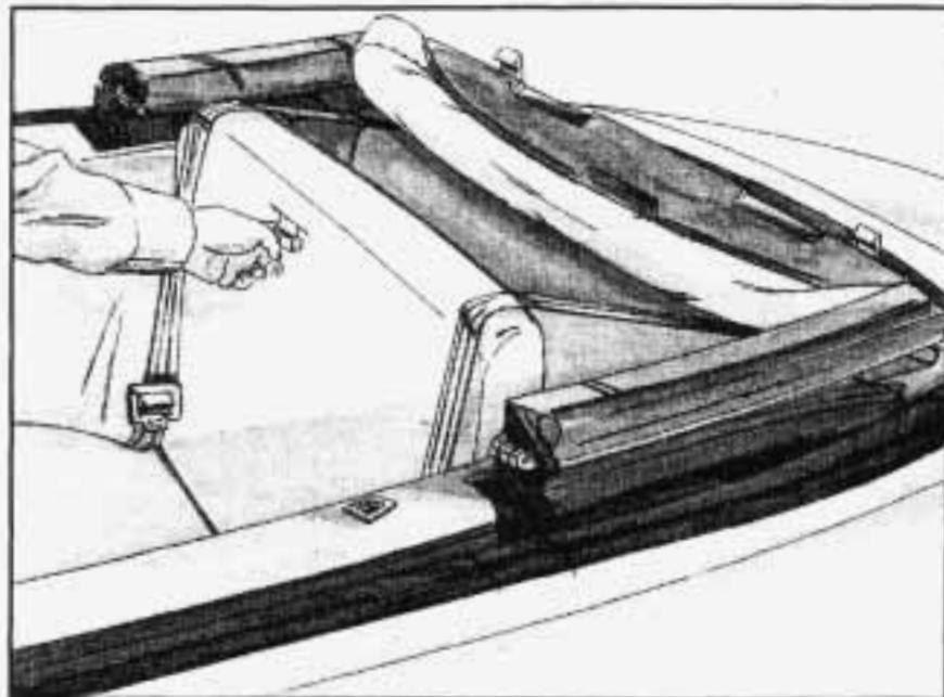
6. From inside the vehicle, pull the tab on the rear seat to fold down the seat. See "Fold-Down Rear Seat" in the Index.
