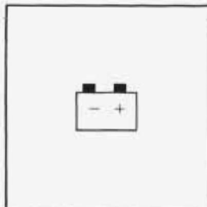
The battery light will come on briefly when you turn on the ignition, and the engine is not running, as a check to show you it is working. Then it should go out.
