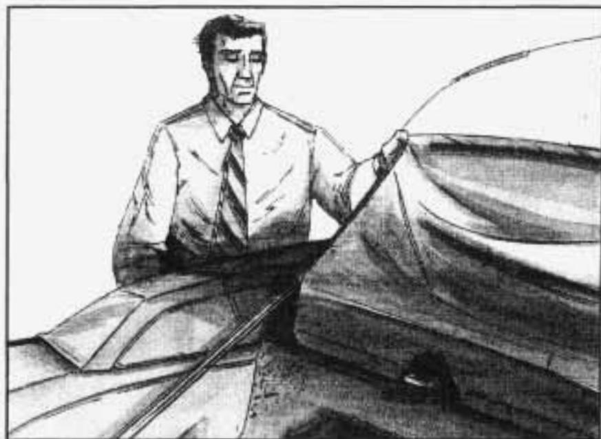
4. Go to the rear of the vehicle. Pull the snap knobs rearward to disengage the rear center cover. Carefully tuck the center boot behind the rear seatback. Make sure that the center cover is not covering the rear seatback latch. Tuck end of center boot rearward to keep it away from the rear seatback hinge.
