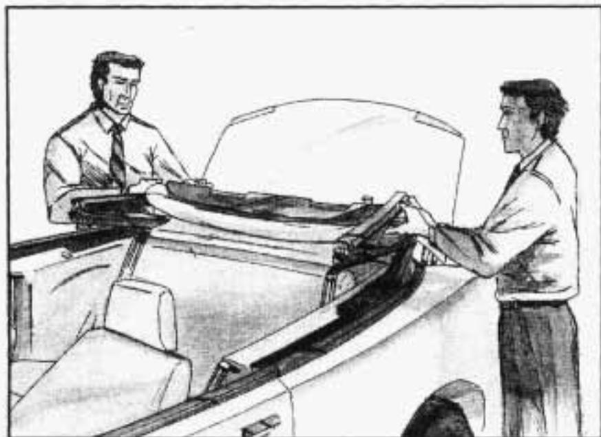
8. Raise the top until it is all the way up. Line up the top so the pins are even with the holes.
