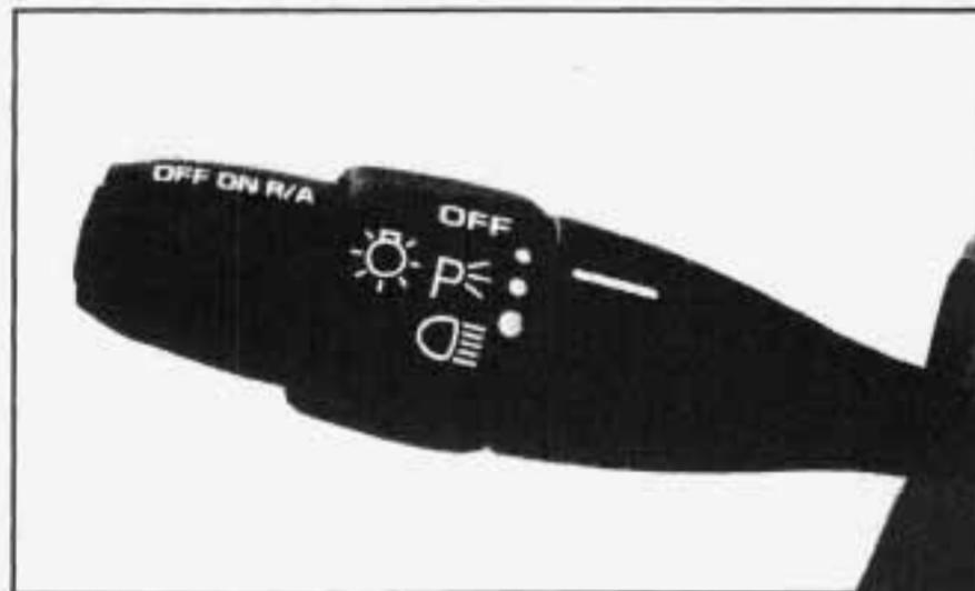
With cruise control, you can maintain a speed of about 25 mph (40 km/h) or more without keeping your foot on the accelerator. This can really help on long trips. Cruise control does not work at speeds below about 25 mph (40 km/h)
