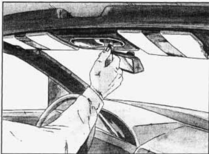
4. Pull the latch handle rearward away from the windshield and hold it to fully lower the convertible top.
