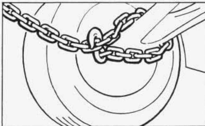
Attach a separate safety chain around the outboard end of each lower control arm.
