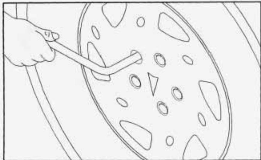
1. Using the wheel wrench, remove the plastic cap nuts (if your vehicle is so equipped) and *loosen* all the wheel nuts. Don't remove the wheel nuts yet. On some models, a cover plate must be removed to find the wheel nuts. Carefully use the wedge end of the wheel wrench to pry it off.
