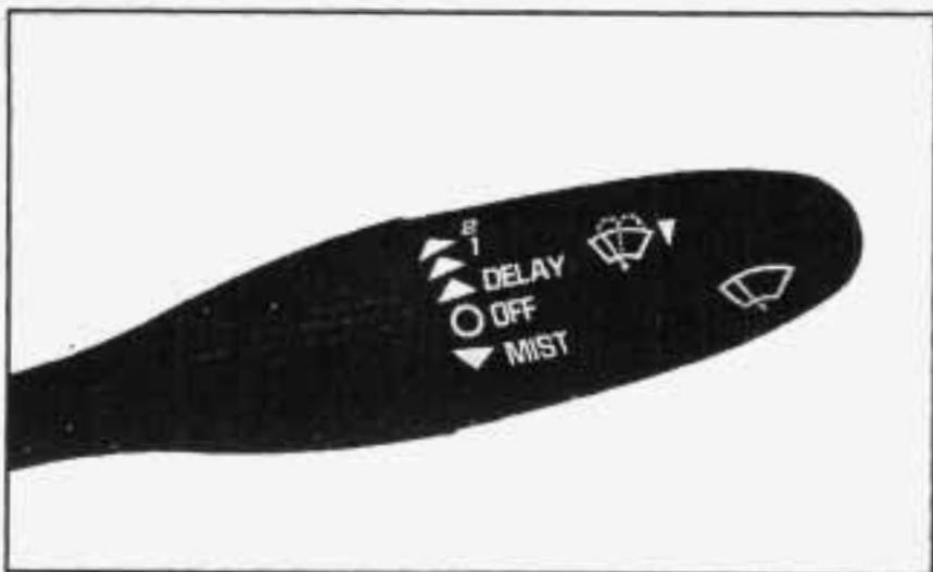
You control the windshield wipers by moving the stalk with the windshield wiper symbol on it up or down.
