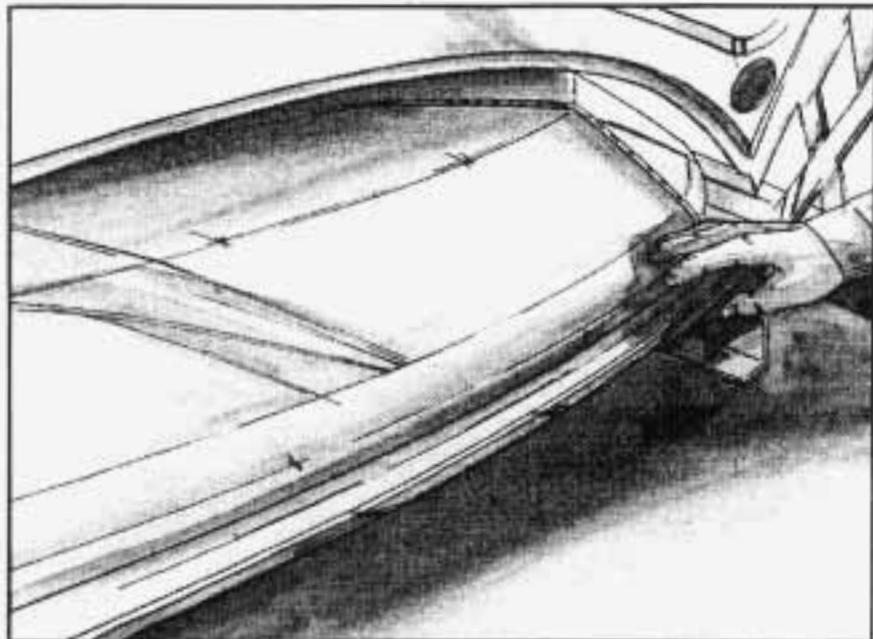
11. Go to the rear of the vehicle. Place the boot center cover flap along the trunk lid opening. Align one snap to snap ball stud and push forward. Repeat for other snap.
