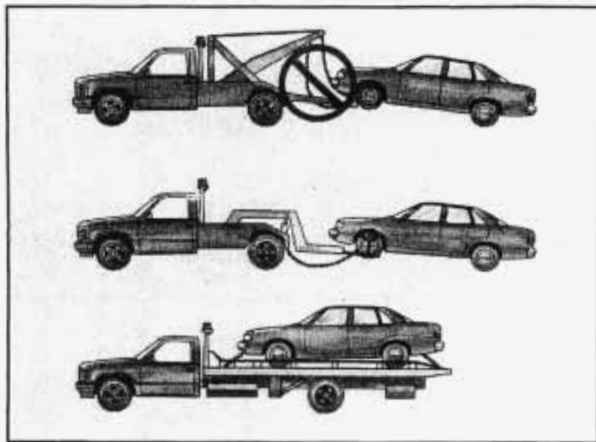
Before hooking up to a tow truck, be sure to read all the information in "Towing Your Vehicle" earlier in this section.
