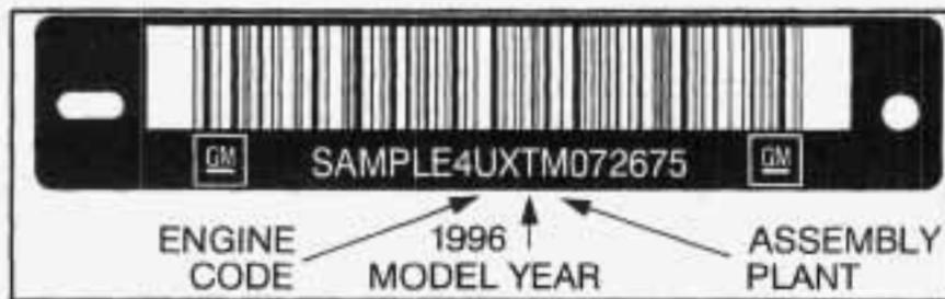
This is the legal identifier for your Pontiac. It appears on a plate in the front corner of the instrument panel, on the driver's side. You can see it if you look through the windshield from outside your vehicle. The VIN also appears on the Vehicle Certification and Service Parts labels and the certificates of title and registration.
