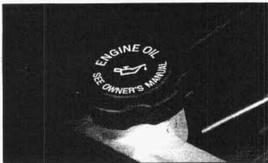
This is where you add oil if you have a 2.4L engine. Just fill it enough to put the level somewhere in the proper operating range. Push the dipstick all the way back in when you're through.
