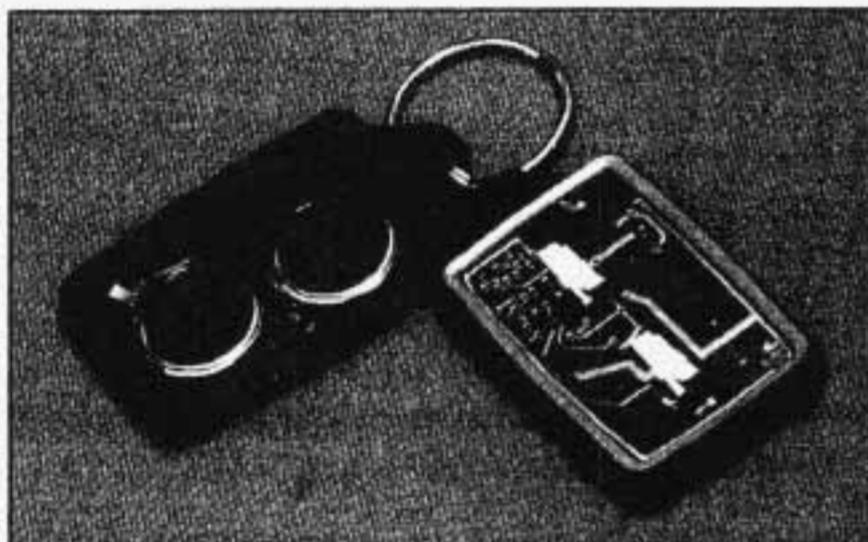
3. Remove and replace the two batteries. Use two Duracell<sup>®</sup> batteries, type DL-2016, or equivalent.
