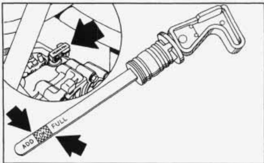
3. Check both sides of the dipstick and read the lower level. The fluid level must be between the ADD and FULL marks. (Note: Fluid may appear at the bottom of the dipstick even when the fluid level is several pints low.)
