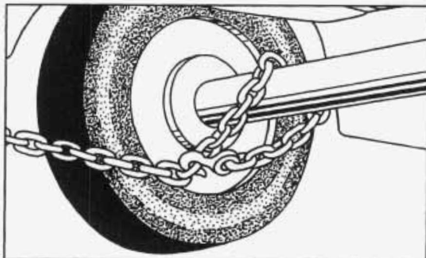
Attach a separate safety chain to each side of the axle inboard of the rear shock absorber attachment. (Do not use this chain as a tie down.)
