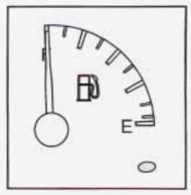
Your fuel gage tells you about how much fuel you have left, when the ignition is on. When the indicator nears EMPTY (E), you still have a little fuel left, but you should get more soon. An amber light will come on below the gage when the fuel tank is near EMPTY (E).
