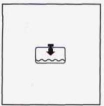
If this light comes on and stays on, the vehicle should be promptly pulled off the road and the coolant level checked. See "Engine Coolant" in the Index.
