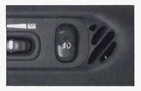
The switch for your fog lamps is next to the instrument panel intensity control.
