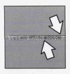
Check both sides of the dipstick, and read the lower level. The fluid level must be in the cross-hatched area.
