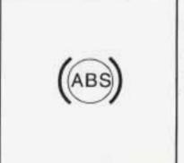
If there's a problem with the anti-lock brake system, this warning light will stay on. See "Anti-Lock Brake System Warning Light" in the Index.
