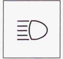
To change the headlamps from low beam to high or high to low, pull the turn signal lever all the way toward you. Then release it. When the high beams are on, this blue light on the instrument panel also will be on.
