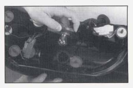
To remove a socket, push in the lock tab and turn the socket counterclockwise to pull it out.
