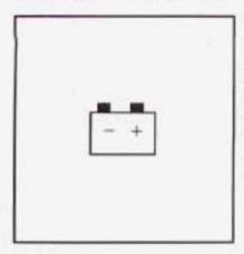
The charging system indicator light will come on briefly when you turn on the ignition, but the engine is not running, as a check to show you it is working. Then it should go out,
