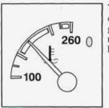
This gage shows the engine coolant temperature. If the gage pointer moves into the red area, your engine is too hot!
