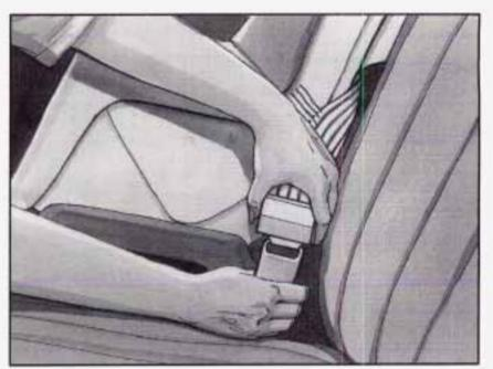
Buckle the belt. Make sure the release button is positioned so you would be able to unbuckle the safety belt quickly if you ever had-to.
