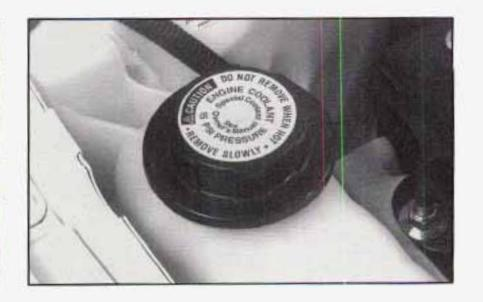
You can remove the coolant surge tank pressure cap when the cooling system, including the coolant surge tank pressure cap and upper radiator hose, is no longer hot. Turn the pressure cap slowly about one-quarter turn to the left and then stop.
