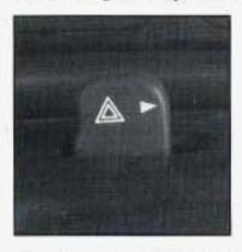
Move the switch to the right to make your front and rear turn signal lamps flash on and off.
