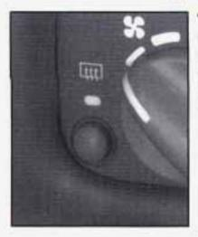
The rear window defogger uses a warming grid to remove fog from the rear window. Press the defogger switch. The indicator light will glow.
