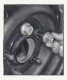
Replace the wheel nuts with the rounded end of the nuts toward the wheel. Tighten each nut by hand until the wheel is held against the hub.
