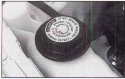
4. With the coolant surge tank pressure cap off, start the engine and let it run until you can feel the upper radiator hose getting hot. Watch out for the engine fan. By this time, the coolant level inside the coolant
