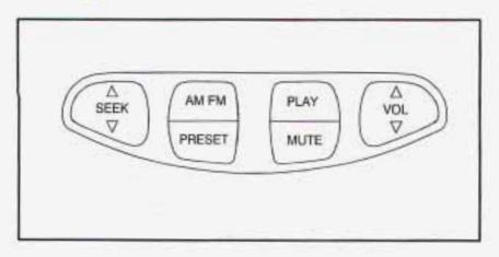
If your vehicle has this feature, you can control certain radio functions using the buttons on your steering wheel.
