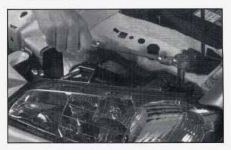
Remove the two headlamp assembly attachment bolts.
