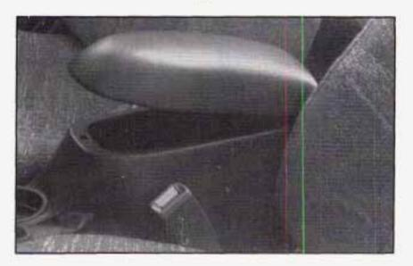
Pull up on the front edge of the armrest to open the center console storage area for cassette tapes, gloves, etc.
