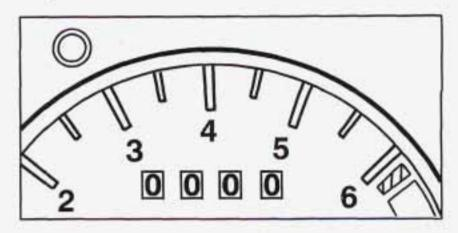
The trip odometer can tell you how far you have driven since you last reset it. To reset the trip odometer to zero, press the knob at the top left side of the instrument panel cluster.
