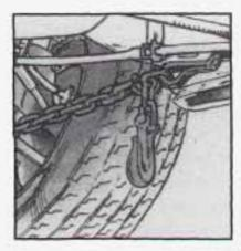
Attach T-hook chains on both sides in the slotted holes in the underbody just ahead of the wheels.
