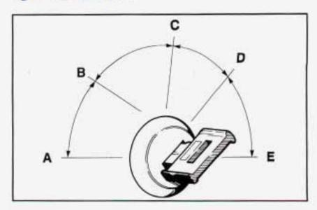
With the key in the ignition switch, you can turn the switch to five positions.
