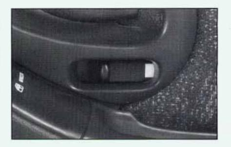
From the inside, you can lock the door by sliding the locking lever rearward.
