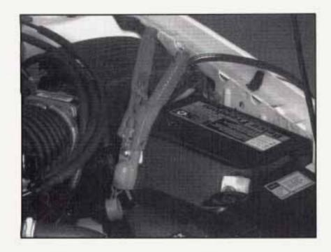
Connect the red positive (+) cable to the positive (+) terminal of the vehicle with the dead battery.
