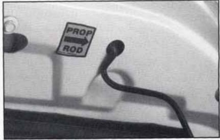
Lift the hood, release the hood prop rod from its retainer and put the hood prop into the slot in the hood.
