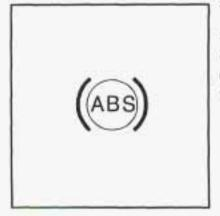
With the anti-lock brake system, this light will come on when you start your engine and it will stay on for three seconds. That's normal.
