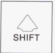
This light comes on when you need to shift to the next higher gear. See "Manual Transaxle" in the Index.
