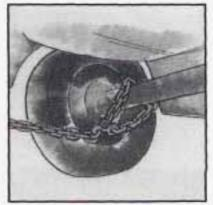
Attach a separate safety chain to each side of the axle inboard of the spring.
