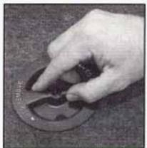
The equipment you'll need is in the trunk. Pull the carpeting from the floor of the trunk. Turn the center retainer nut on the compact spare cover counterclockwise to remove it.
