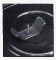
Turn the wing nut counterclockwise and remove it. Then lift off the spacer and remove the spare tire.
