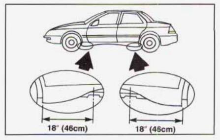
Position the jack and raise the jack head until it fits firmly into the notch in the vehicle's frame nearest the flat tire. Put the compact spare tire near you.
