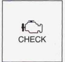
Your Pontiac is equipped with a computer which monitors operation of the fuel, ignition and emission control systems.
