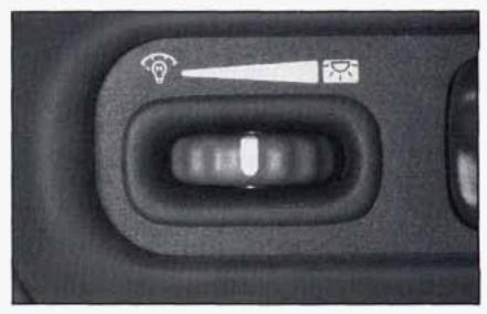
You can brighten or dim your instrument cluster lamps by rotating the instrument panel intensity control switch. Rotate the switch all the way to the right to turn on the interior courtesy lamps. Rotate the switch to the left to turn off the instrument cluster lamps and displays.
