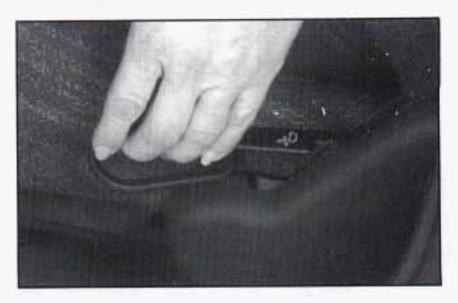
To adjust the seatback, lift the lever on the outer side of the seat and move the seatback where you want it. Release the lever to lock the seatback. Pull up on the lever and the seat will go to an upright position.
