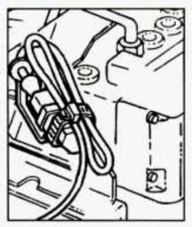
The engine coolant heater cord is secured on the driver's side of the vehicle. by the brake controller.
