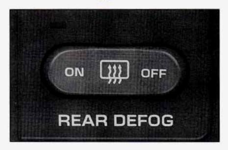
The rear window has lines that warm the glass. For best results, clear the window of as much snow or ice as possible before using the rear window defogger.
