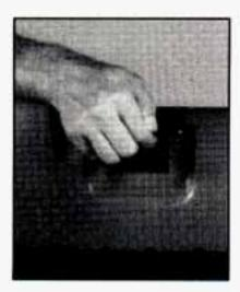
Reach inside the endgate to lift the handle and open the endgate.
