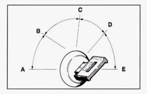
ACCESSORY (A): ACCESSORY lets you use things like the radio and the windshield wipers when the engine is off. Push in the key and turn it toward you. Your steering wheel will remain locked, just as it was before you inserted the key.
