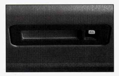
The rear dome lamp has a switch that lets you turn it on from the rear of the vehicle.
