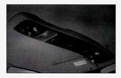
The overhead console includes reading lamps, a driver information system, a storage compartment for sunglasses and a universal transmitter.
