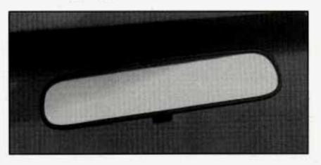
Press the tab under the mirror to reduce glare from headlamps behind you.
