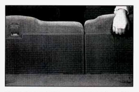
Your vehicle has a folding rear seat which lets you fold the seatbacks down for more cargo space. The rear seat release handles are in the upper center of the rear of the seatbacks. Push back on the seatbacks as you pull up on the handles.
