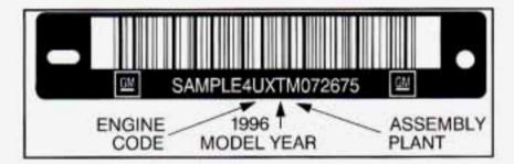
This is the legal identifier for your Oldsmobile. It appears on a plate in the front corner of the instrument panel, on the driver's side. You can see it if you look through the windshield from outside your vehicle. The VIN also appears on the Vehicle Certification and Service Parts labels and the certificates of title and registration.
