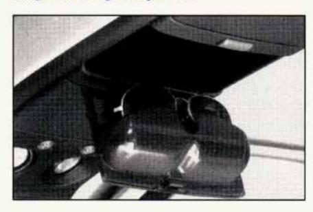
To open the sunglasses storage compartment in the overhead console, press the release button. Then pull the compartment down.
