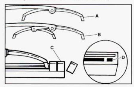
To install the new wiper insert, slide the insert (D), notched end last, into the end with two blade claws (A). Slide the insert all the way through the blade claws at the opposite end (B). The
