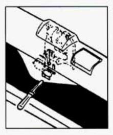
Use a thin screwdriver to reach through the access holes in both the trim panel and the hardware cover.
