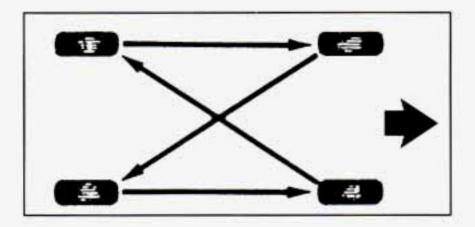
The purpose of regular rotation is to achieve more uniform wear for all tires on the vehicle. The first rotation is the most important. See "Scheduled Maintenance Services" in the Index for scheduled rotation intervals. When rotating your tires, always use the correct rotation pattern shown here.
