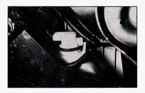
3. Turn the socket counterclockwise and pull it out.
