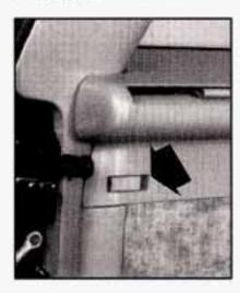
To remove the jack cover, pull up on the latch at the end of the cover, near the endgate.
