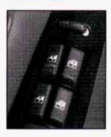
These switches on the driver's door control each of the windows when the ignition is in the RUN position.
