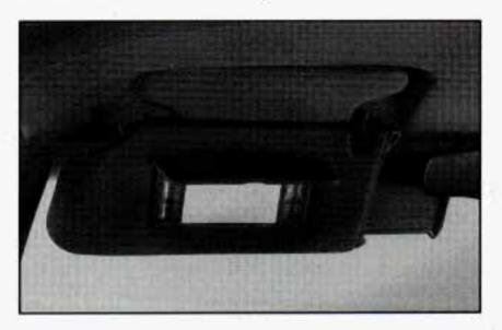
Pull the sun visor down and lift the mirror cover to turn on the lamps.
