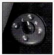
The control is located on the driver's door armrest. Turn the control to L or R to choose the mirror, then press the arrows on the outside switch ring to adjust the mirror.
