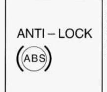
If there's a problem with the anti-lock brake system, this warning light will stay on. See "Anti-Lock Brake System Warning Light" in the Index.
