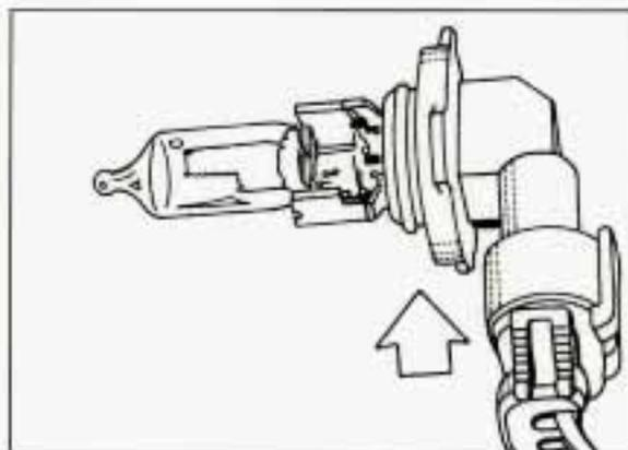
3. Disconnect the bulb base from the socket by lifting the plastic locking tab.
