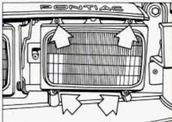
2. Remove the four Torx® screws from the corners of the frame around the headlight.
