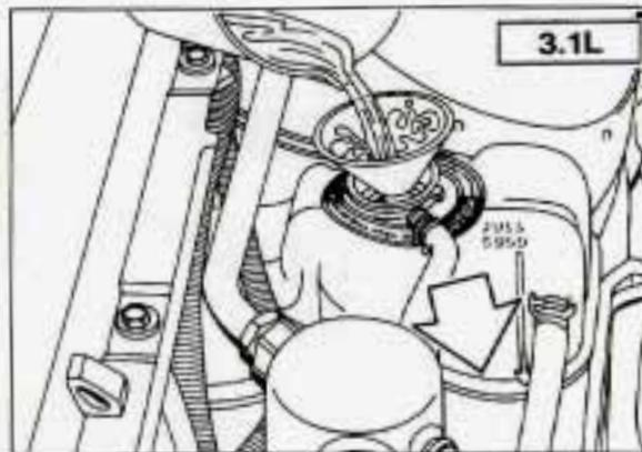
3. Fill the coolant surge tank with the proper mix, up to **FULL COLD**.
