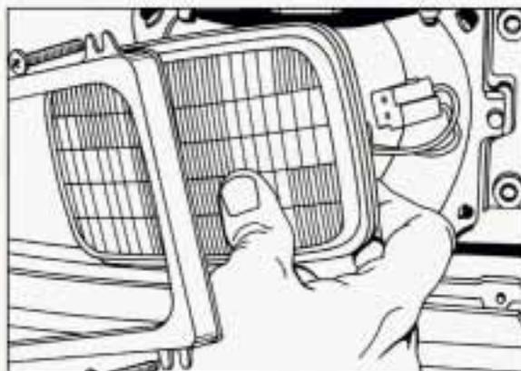
3. Separate the headlight from the back plug by pulling the plug straight back.
