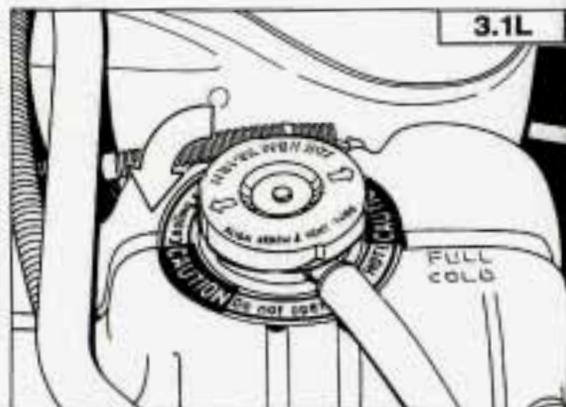
1. You can remove the coolant surge tank pressure cap when the cooling system, including the coolant surge tank pressure cap and upper radiator hose, is no longer hot. Turn the pressure cap slowly to the left until it first stops. (Don't press down while turning the pressure cap.) If you hear a hiss, wait for that to stop. A hiss means there is still some pressure left.
