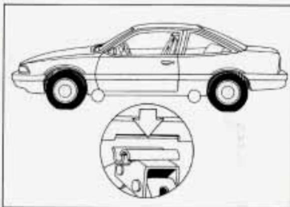
10. Position the jack under the vehicle. Raise the jack head until it fits firmly into the notch in the vehicle's frame nearest the flat tire. Put the compact spare tire near you.
