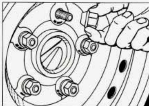
14. Replace the wheel nuts with the rounded end of the nuts toward the wheel. Tighten each nut by hand until the wheel is held against the hub.
