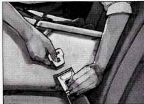
3. Put the belt's special latch plate into the vehicle's safety belt buckle.
