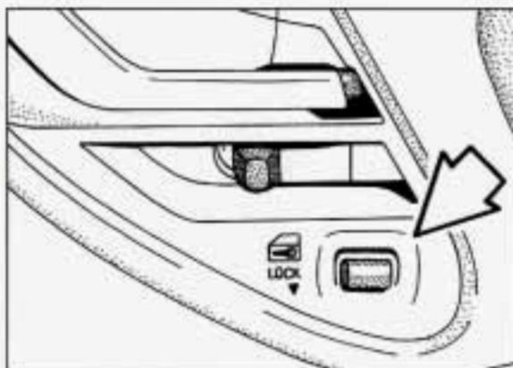
On 2-door models, push the switch down to lock your doors and up to unlock them.
