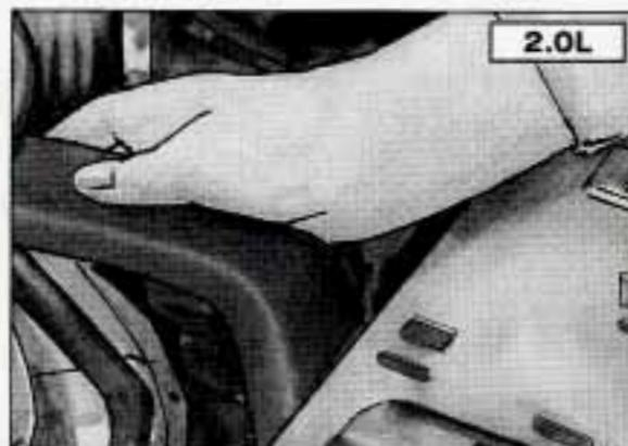
7. Start the engine and let it run until you can feel the upper radiator hose getting hot. Watch out for the engine fan.
