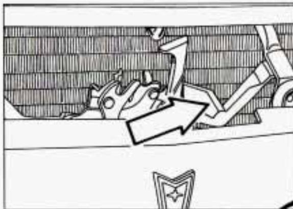
Then go to the front of the vehicle and release the secondary hood release by pushing the lever to the right.
