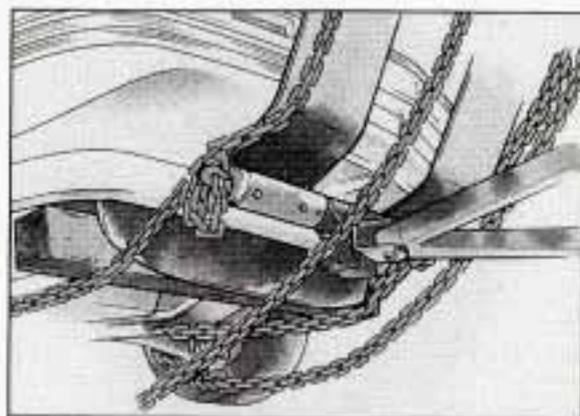
2. Position a 4x4 wood beam across sling chains, contacting the bottom of the radiator support just behind the air dam.
