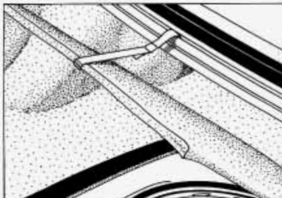
**3.** If your vehicle is equipped with a spare tire housing lid hook, pull the front of the lid up and hook it to the rear upper edge of the trunk.
