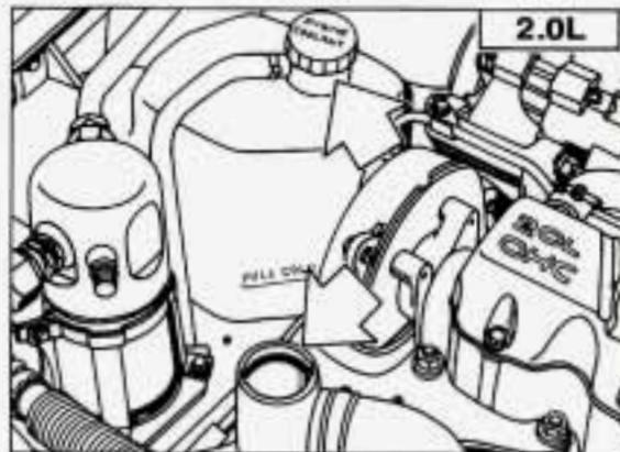
6. Put the cap back on the coolant recovery tank, but leave the thermostat housing pressure cap off.
