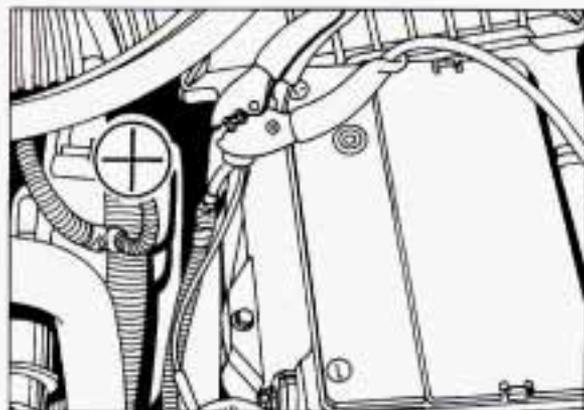
6. Connect the red positive (+) cable to the positive (+) terminal of the vehicle with the dead battery. Use a remote positive (+) terminal if the vehicle has one.
