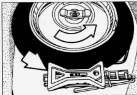
**2.** Remove the wing bolt securing the compact spare tire, spacer and wheel wrench by turning it counterclockwise. Then lift off the spacer and remove the spare tire.
