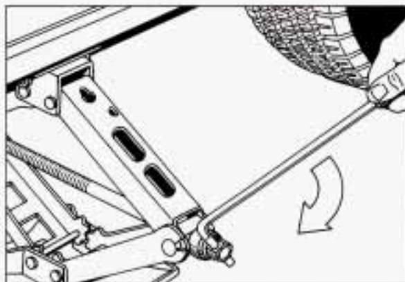
8. Raise the vehicle by rotating the jack handle clockwise. Raise the vehicle far enough off the ground so there is enough room for the spare tire to fit.
