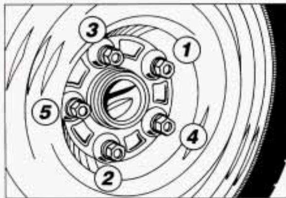
13. Tighten the wheel nuts firmly in a criss-cross sequence, as shown.
