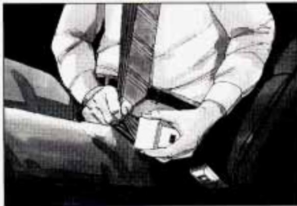
If the belt stops before it reaches the buckle, tilt the latch plate and keep pulling until you can buckle it.
