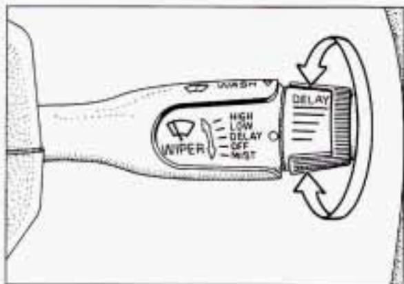
You can set the wiper speed for a long or short delay between wipes. This can be very useful in light rain or snow.
