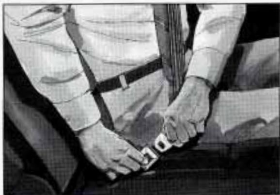
We hope you'll always keep your automatic belt buckled. However, you may need to unbuckle it in an emergency. To unbuckle the automatic belt, just push the button on the buckle.
