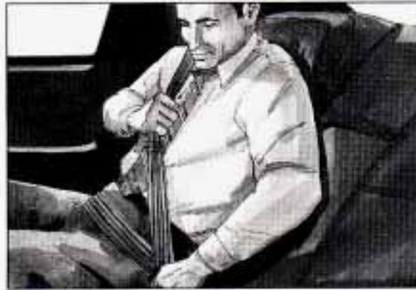
3. To make the lap part tight, pull down on the buckle end of the belt as you pull up on the shoulder part.
