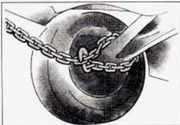
2. Attach a separate safety chain around the outboard end of each lower control arm.
