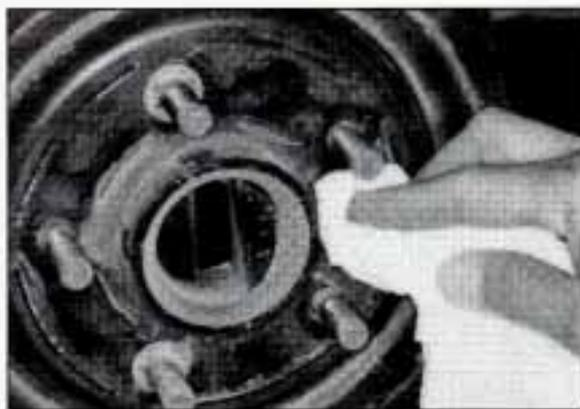
10. Remove any rust or dirt from the wheel bolts, mounting surfaces and spare wheel. Place the spare on the wheel mounting surface.
