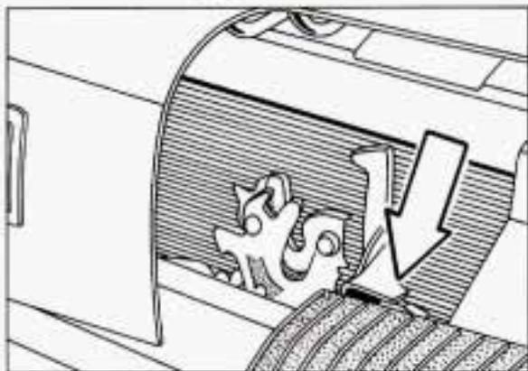
Then go to the front of the vehicle and push the secondary hood release down to lift the hood.
