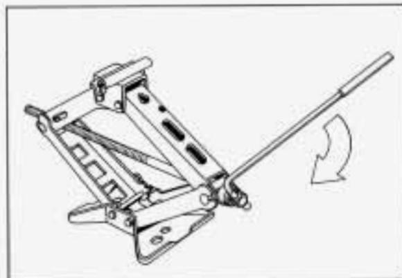
**4.** Remove the band around the jack. Turn the jack handle clockwise to raise the jack head a few inches.
