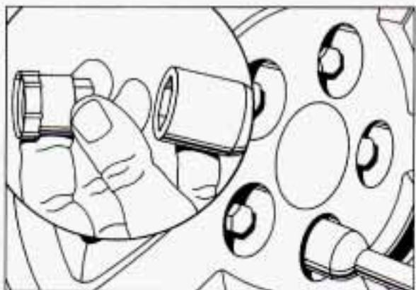
5. Using the wheel wrench, remove the wheel nut caps (if your vehicle has them) and loosen all the wheel nuts. Don't remove them yet. On some models, a cover plate must be removed to find the wheel nuts. Carefully use the wedge end of the wheel wrench to pry it off.
