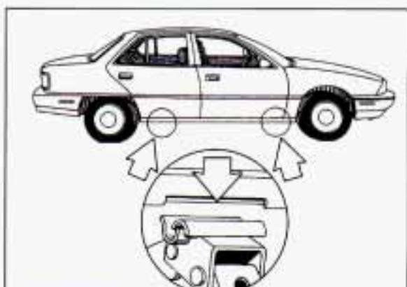
7. Position the jack under the vehicle. Raise the jack head until it fits firmly into the notch in the vehicle's frame nearest the flat tire. Do not raise the vehicle yet. Put the compact spare tire near you.
