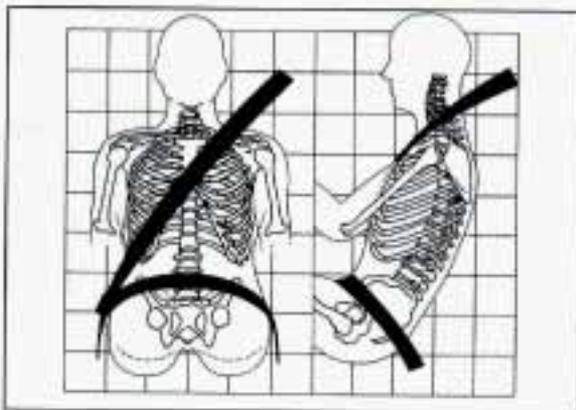
The lap part of the belt should be worn low and snug on the hips, just touching the thighs. In a crash, this applies force to the strong pelvic bones. And you'd be less likely to slide under the lap belt. If you slid under it, the belt would apply force at your abdomen. This could cause serious or even fatal injuries. The shoulder belt should go over the shoulder and across the chest. These parts of the body are best able to take belt restraining forces.
