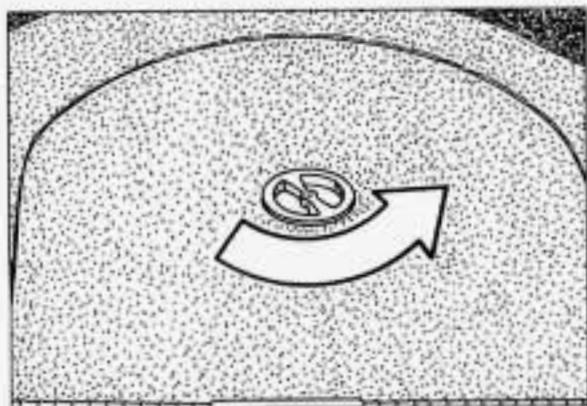
**1.** Turn the center retainer nut on the compact spare tire housing counterclockwise to remove it, then lift the tire cover. You will find the jacking instructions label on the underside of the tire cover.
