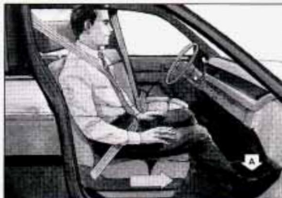
Adjust the seat (to see how, see *Seats* in the *Index*) so you can sit up straight. Move your seat far enough forward that your feet touch the part of the car that is called the "toeboard" (A). That way you'd be less likely to slide under the lap belt in a crash.
