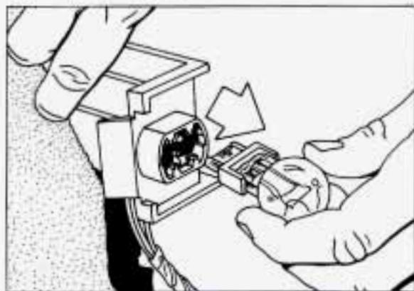
3. Wiggle the bulb out of the socket.
