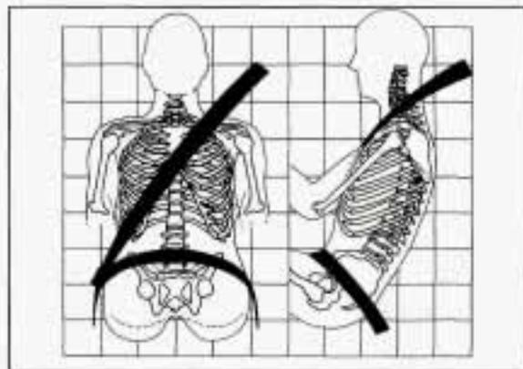
The lap belt should be worn as low on the hips as possible. In a crash, this applies force to the strong pelvic bones. And you'd be less likely to slide under the lap belt. If you slid under it, the belt would apply force at your abdomen. This could cause serious or even fatal injuries. The shoulder belt should go over the shoulder and across the chest. These parts of the body are best able to take belt restraining forces.
