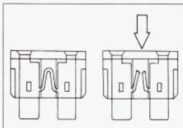
Look at the silver-colored band inside the fuse. If the band is broken or melted, replace the fuse. Be sure you replace a bad fuse with a new one of the correct size.
