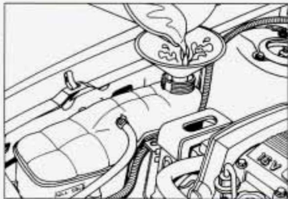
4. Fill the coolant surge tank with the proper mix, up to **FULL COLD**, or just above the small cylinder at the base of the opening.
