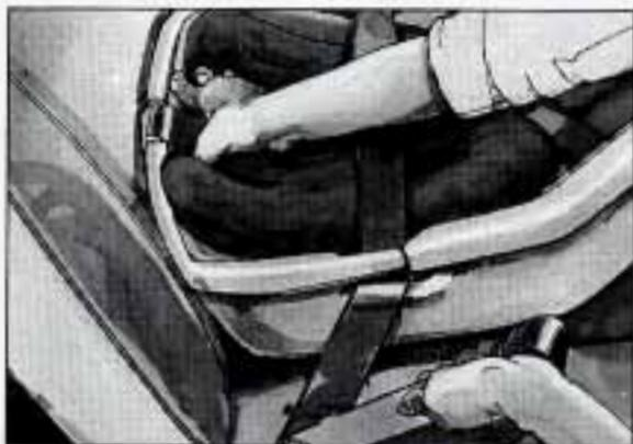
9. To make it tight, pull the belt while you push down on the child restraint. If the belt won't stay tight, switch it end for end.
