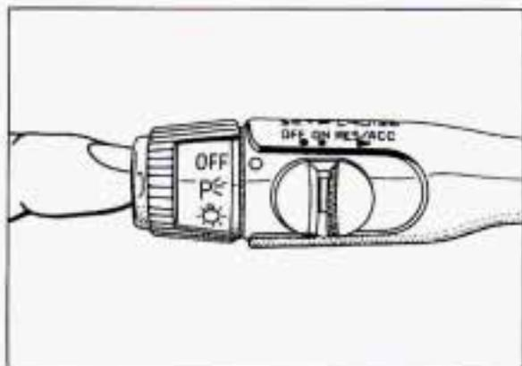
3. Press in the **SET** button at the end of the lever and release it.
