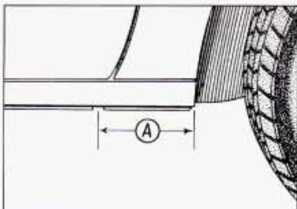
6. Near each wheel well is a notch in the frame which the jack head fits in. The front notch is 9" (23 cm) back from the rear wheel well. The rear notch is 8" (20 cm) forward from the rear wheel well. If your vehicle has flared side moldings, both front and rear notches are 18" (46 cm) from the wheel wells.
