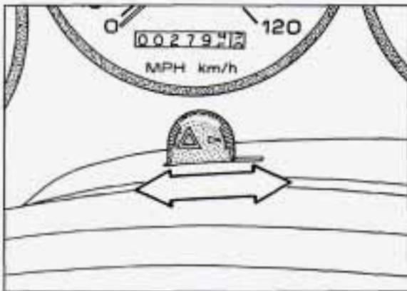
Move the switch to the right to make your front and rear turn signal lights flash on and off.
