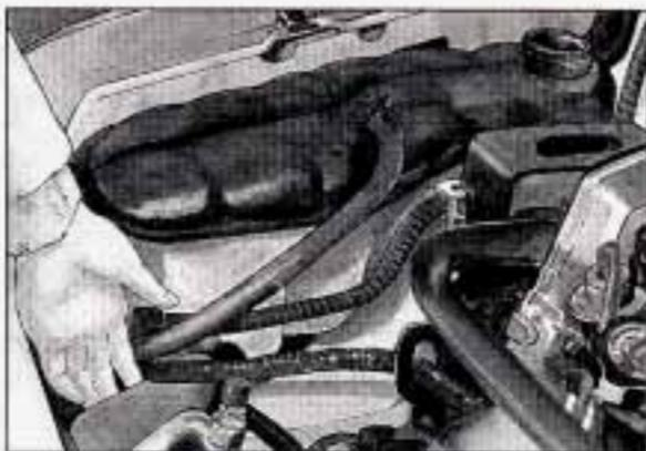
5. With the coolant surge tank pressure cap off, start the engine and let it run until you can feel the upper radiator hose getting hot. Watch out for the engine fan. By this time, the coolant level inside the coolant surge tank may be lower. If the level is lower, add more of the proper mix to the coolant surge tank until the level reaches **FULL COLD**, or just above the small cylinder at the base of the opening.
