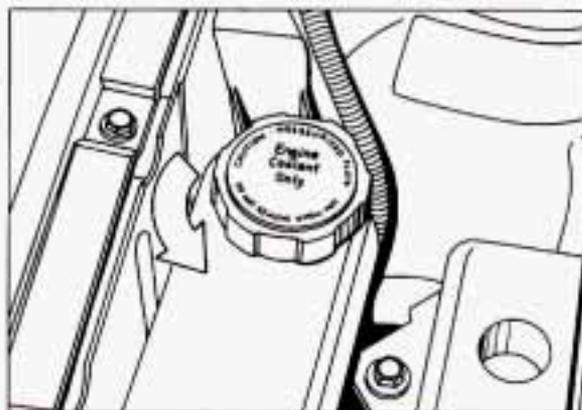
1. You can remove the coolant surge tank pressure cap when the cooling system, including the coolant surge tank pressure cap and upper radiator hose, is no longer hot. Turn the pressure cap slowly about one-quarter turn to the left and then stop. If you hear a hiss, wait for that to stop. A hiss means there is still some pressure left.
