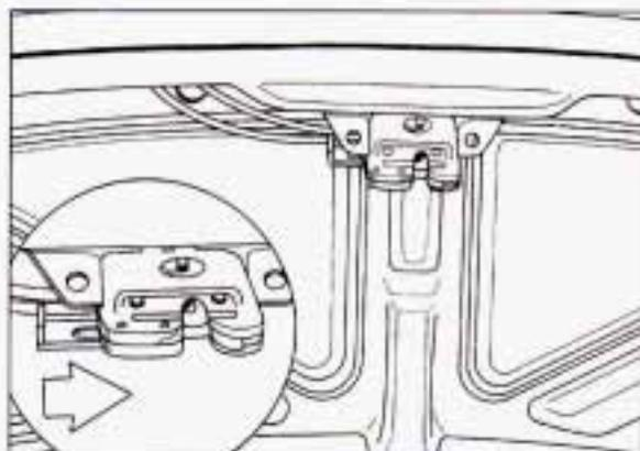
**Lockout Feature:** Your remote trunk release may be equipped with a lockout feature to help prevent unauthorized entry into the trunk when leaving the vehicle unattended. The switch is located on the inside of the trunk lid, mounted to the trunk lid latch.
