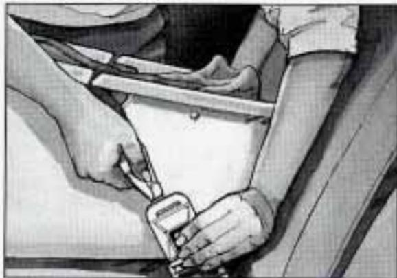
8. Put the hook on the free end through the slot in the latch plate.
