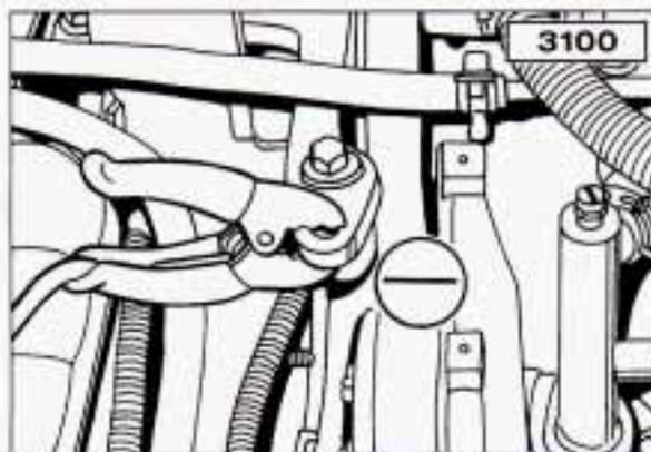
7. Don't let the other end touch metal. Connect it to the positive (+) terminal of the good battery. Use a remote positive (+) terminal if the vehicle has one.
