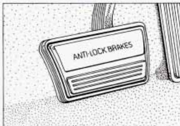
When you start your vehicle, or when you begin to drive away, you may hear a momentary motor or clicking noise. And you may even notice that your brake pedal moves a little while this is going on. This is the ABS system testing itself. If there's a problem with the anti-lock brake system, the anti-lock brake system warning light will stay on or flash.
