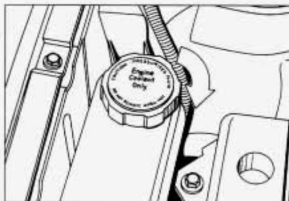
6. Then replace the pressure cap. Be sure the pressure cap is tight.
