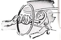
instruments, and accessories. Parking lights operate by rotating knob to "S" position—also controls instrument light. Turning the knob to "H" will turn headlights on and front parking lights off. A map light switch is located under dash panel, to right of the cigarette lighter.
