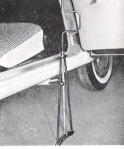
Continental Tire Carrier • The spare tire can be easily removed when necessary. First, remove the two bolts that secure the hub cap assembly with the wheel wrench. With the hub cap assembly suspended, remove the wheel key lock on the top nut with the trunk key turning clockwise. Using the wheel wrench, remove the three hex nuts. The spare tire and wheel assembly is now free. The vinyl tire cove. is secured with snaps and can readily be removed and replaced.
