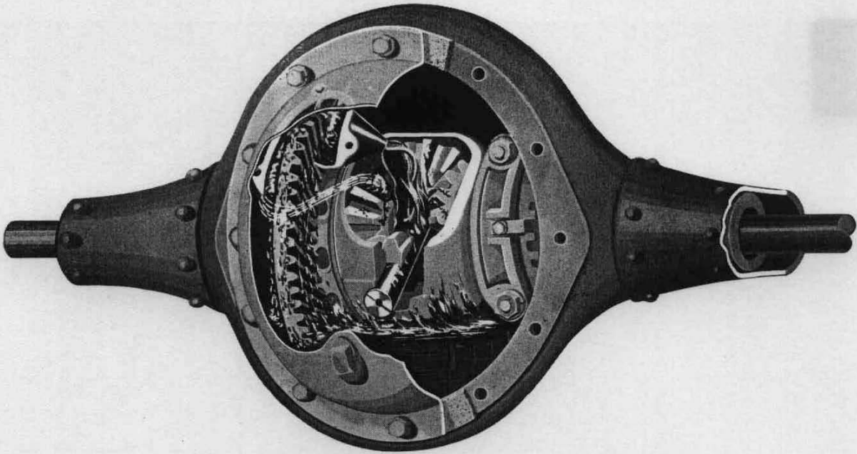
Fig. 25. Cut-a-Way Showing Oil Baffle.
