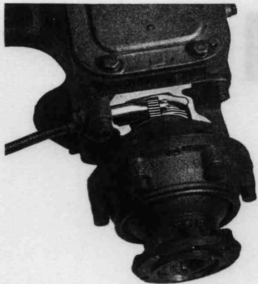
Fig. 27. Housing Cut-a-Way Showing Speedometer Gears.
