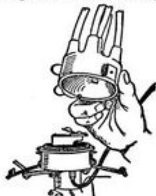
Fig. B. Remove distributor case and wires
