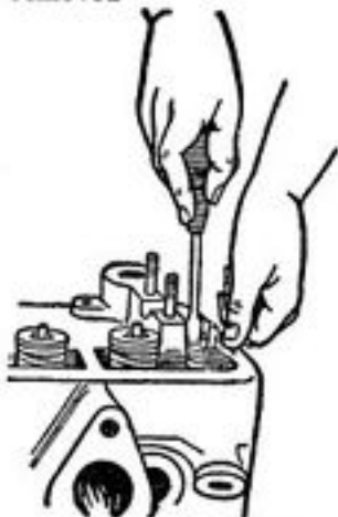
Fig. 17—Removing valve springs.
