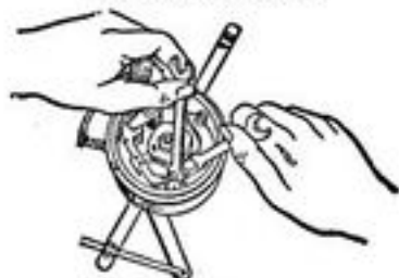
Fig. F. Adjusting contact points
