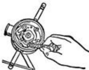
Fig. E. Close contacts and square points by moving file up and down three or four times
