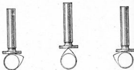
Figure 69.—Operation of Cam and Valve Push Rod.
