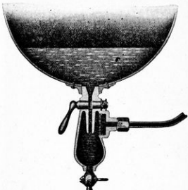
Figure 12.—Fuel Tank and Sediment Trap.
