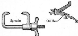
Figure 89.—Using Spring Leaf Spreader for Oiling.
