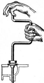
Figure 71.—Using the Valve Grinding Tool.
