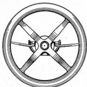
Figure 44.—Spark and Throttle Levers Under Steering Wheel.
