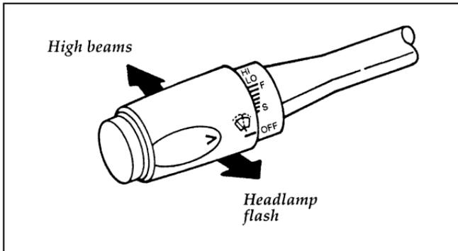
Turning on the high beams
