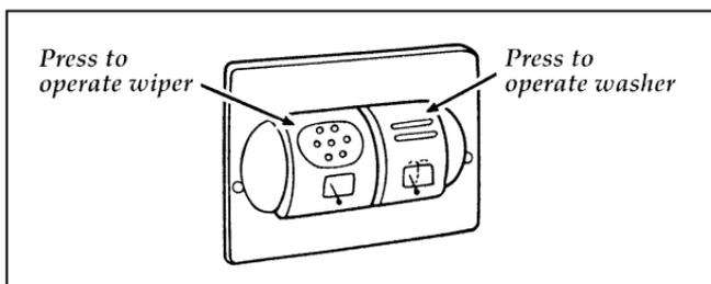
The liftgate window wiper and washer switches
