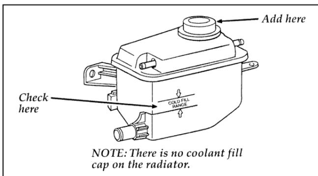
**NOTE:** There is no coolant fill cap on the radiator.
