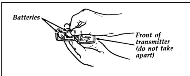
**Replacing the batteries**
