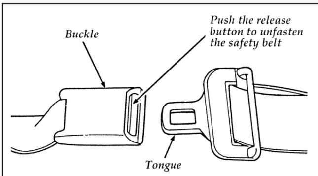
Unfastening the combination lap and shoulder belts — front and rear outboard seating positions
