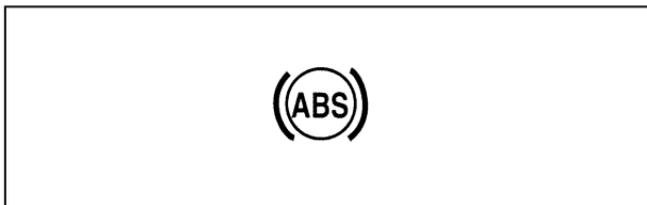
**Anti-lock brake system warning light**
