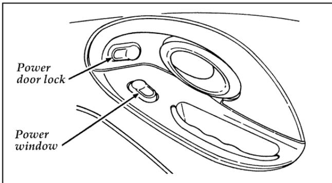
**The window controls on the passenger's door**
