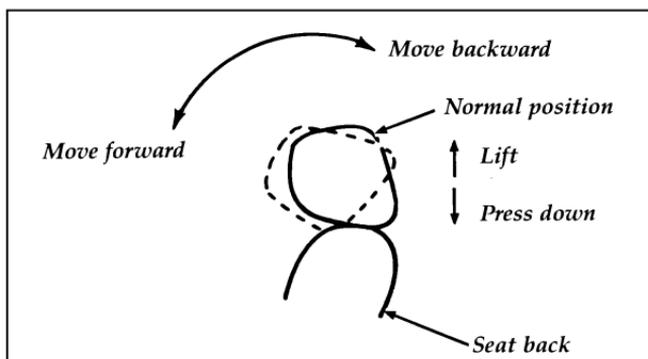
**Adjusting the four-way head restraint**
