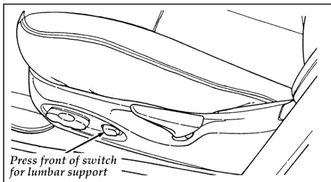
**The seat controls for the lumbar support on the driver's seat**
