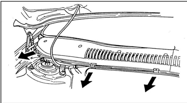
Removing the vacuum hose clips
