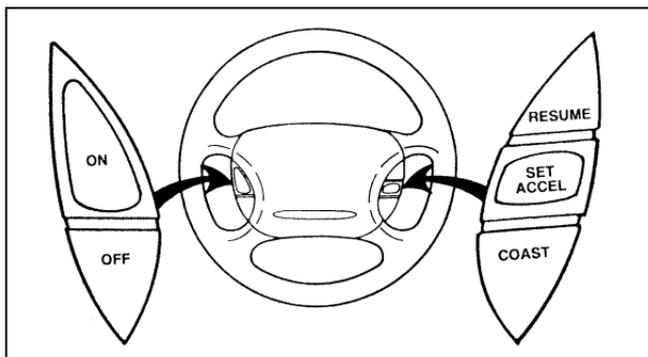
**The speed control buttons on the steering wheel**
