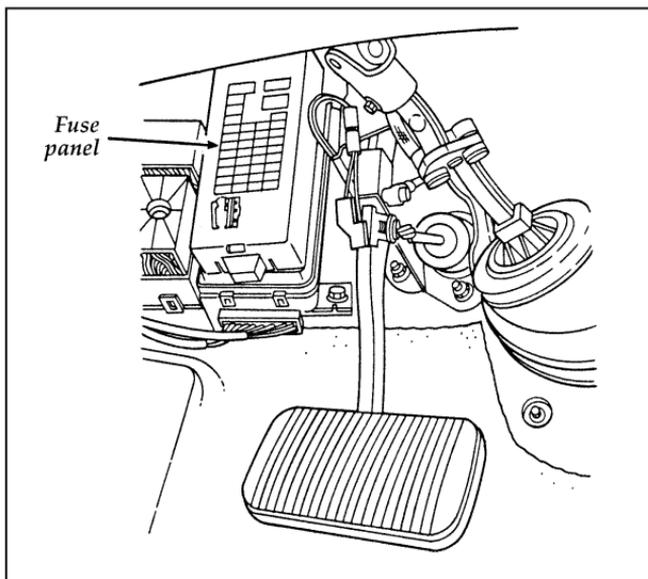
**The instrument panel fuse panel location**
