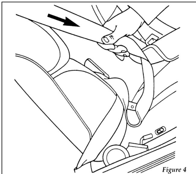
**Setting the retractor to automatic locking mode**
