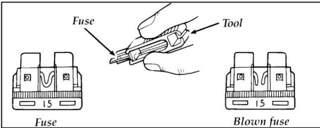
**Fuse puller tool and fuse**
