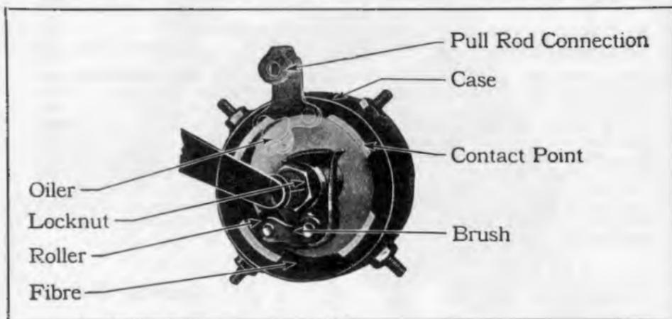
connected with a coil unit, an electrical circuit is passed through the entire system of primary wires. This circuit is only momentary, however, as the roller passes over the contact point very rapidly and sets up the circuit in each unit as the roller touches the contact point connected with that unit. The commutator should be kept clean and well oiled at all times.
