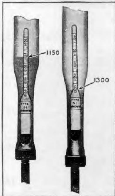
Hydrometer Readings. (Cut No. 26)
