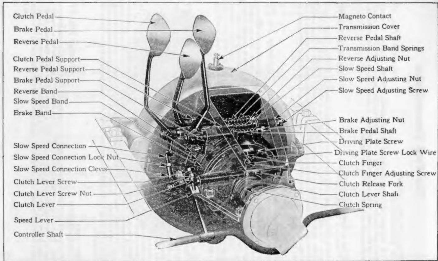
The above drawing of Transmission shows clearly the operation of Clutch, Reverse and Brake Pedals. (Cut No. 12)
