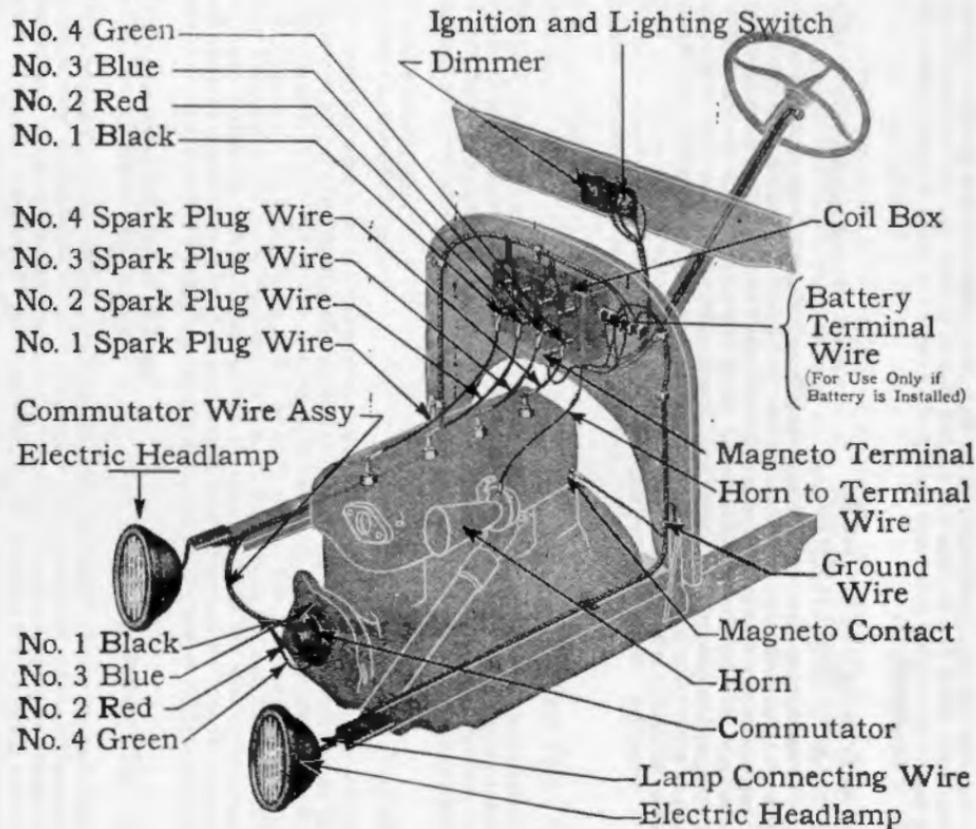
Wiring of Ford Ignition System. (Cut No. 8)
