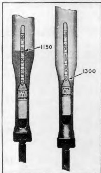
Hydrometer Readings. (Cut No. 26)
