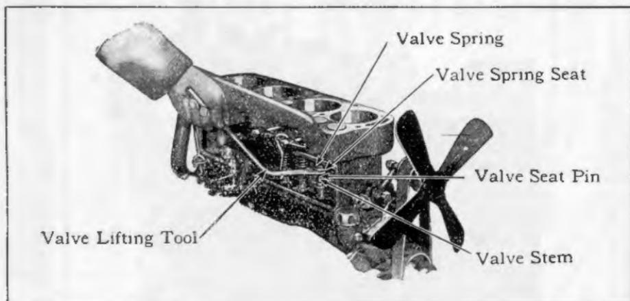
How the valve lifting tool should be used. (Cut No. 4)
