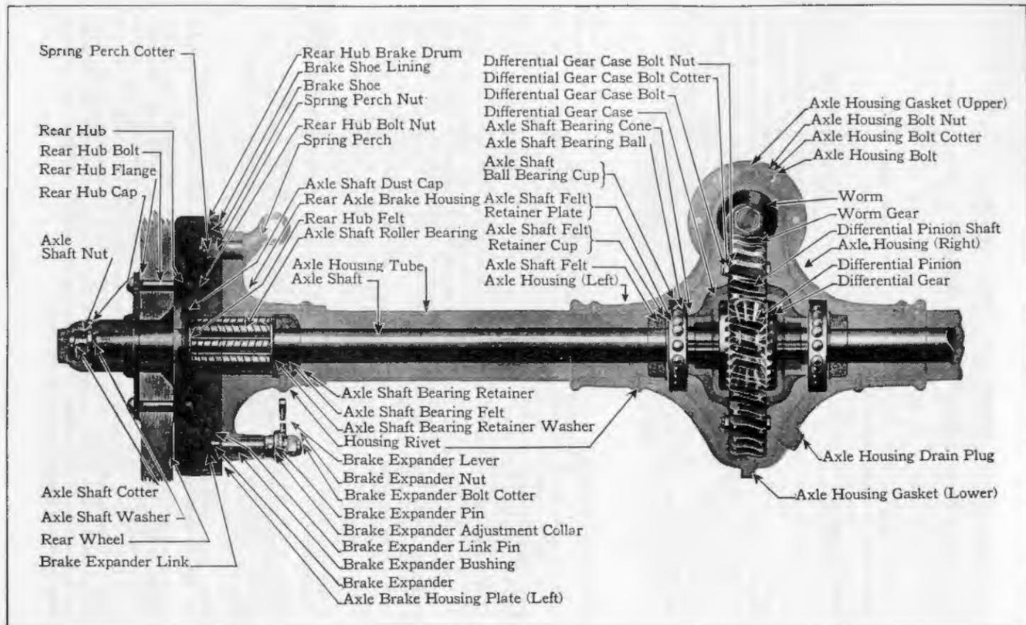
Truck Rear Axle—Longitudinal View. (Cut No. 20)
