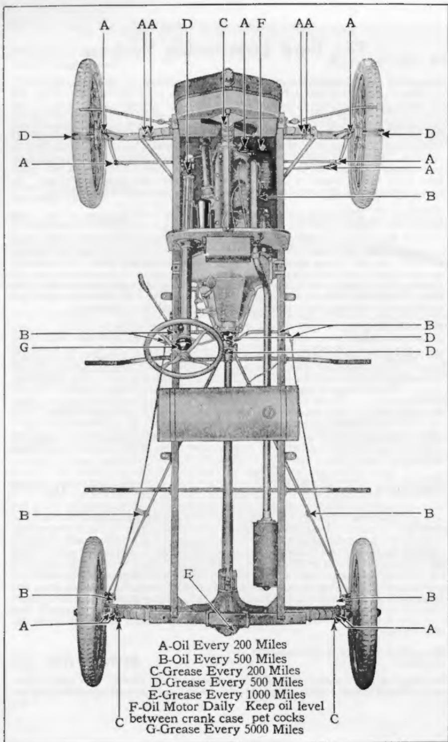
Don't be afraid to put a little oil into the commutator every other day—at least every 200 miles. Remember that the commutator roller revolves very rapidly, and without sufficient lubrication the parts soon become badly worn. When in this condition perfect contact between the roller and the four contact points is impossible; as a result the engine is apt to misfire when running at a good rate of speed.
