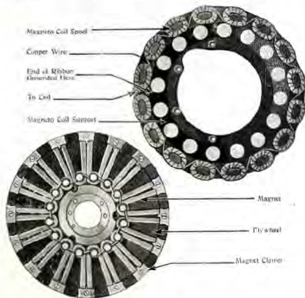
The Ford Magneto. The flywheel with magnets revolves with the engine, while magneto coils remain stationary. (Illus. No. 11).
