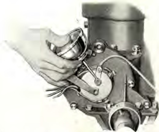
Oiling the Ford Commutator. (Illus. No. 20)
