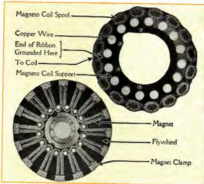
The Ford Magneto. The flywheel with magnets revolves with the engine, while magneto coils remain stationary. (Cut No. 12)
