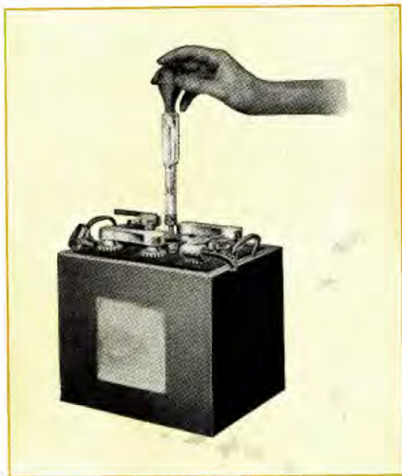
Testing Battery. (Cut No. 30)
