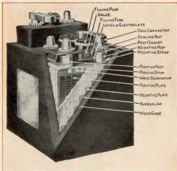
Battery Cut-Out View. (Cut No 36).
