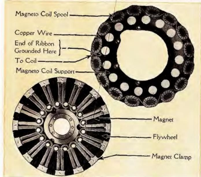
The Ford Magneto. The flywheel with magnets revolves with the engine, while magneto coils remain stationary. (Cut No. 12)
