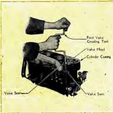
Method of grinding valve. (Cut No. 6)
