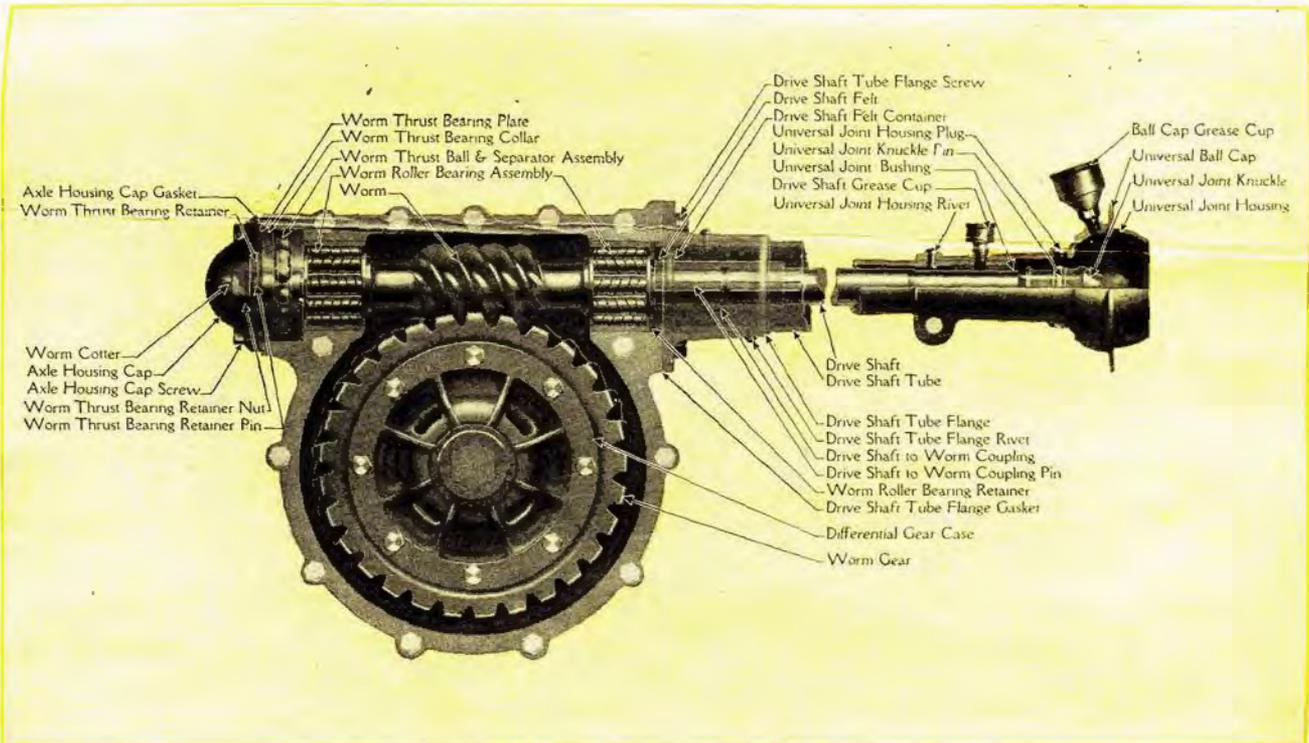
Truck Rear Axle - Cross Section showing Worm and Worm Gear
