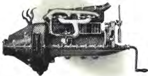
Model T. Motor, Showing Intake and Exhaust Manifolds; also Valve setting. All on right side of motor
