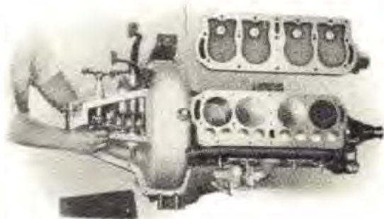
Top view of Motor with cylinder head removed; also showing method of adjusting transmission bands
