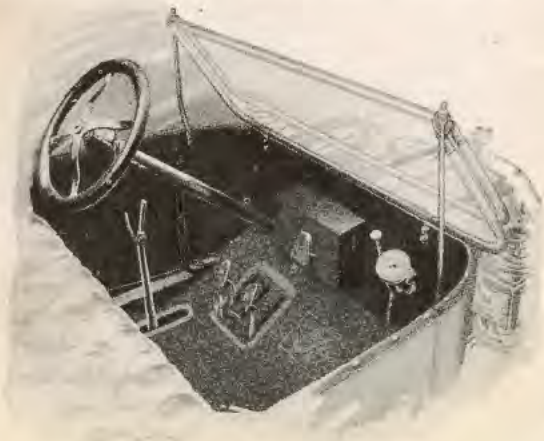
Showing the Simplicity of the Ford Left Hand Control
