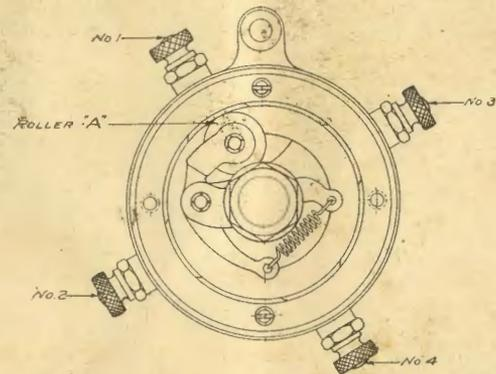
Roller "A" should be on Contact Post No. 1 when Cylinder No. 1 is ready to fire
