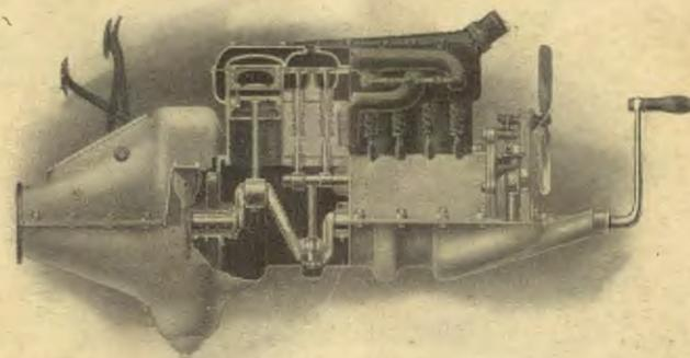
Semi-Sectional View of Model T Engine
